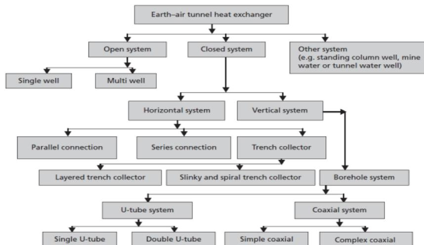
Fig.II.3: Classification of earth to air heat exchanger [4].
