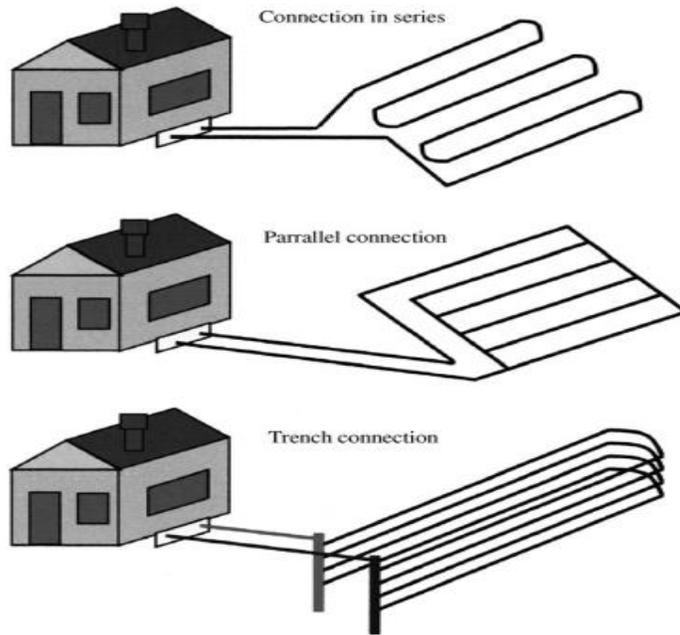
**Fig.II.5:** Horizontal-type ground heat exchangers [5].
