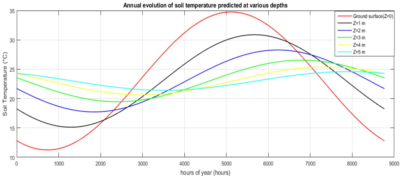
**Fig IV.14:** Annual evolution of soil temperature predicted at various depths.
