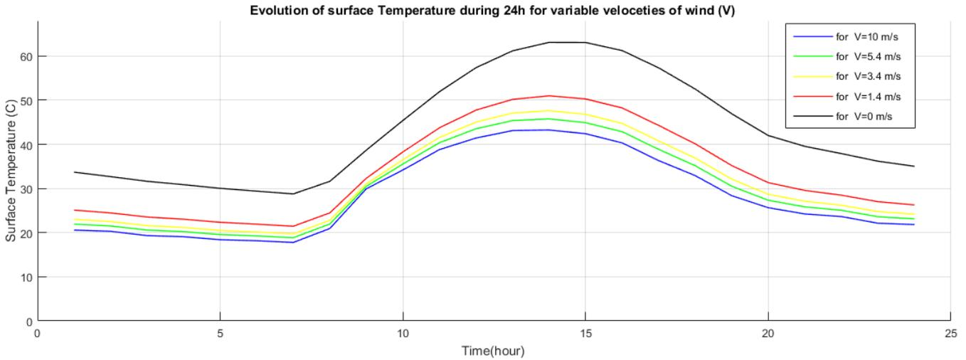
**Fig.IV.6:** Evolution of surface temperature during 24h for variable wind speed values.
