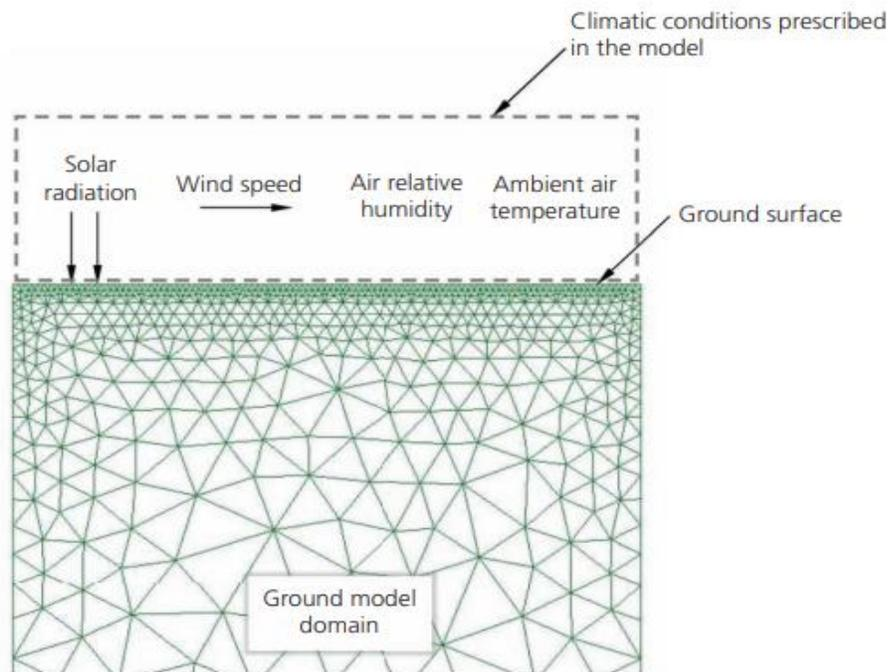
**Fig.IV.2:** Schematic diagram of a ground domain showing the ground surface boundary condition and the climatic variables required in order to calculate the ground surface boundary components [1].
