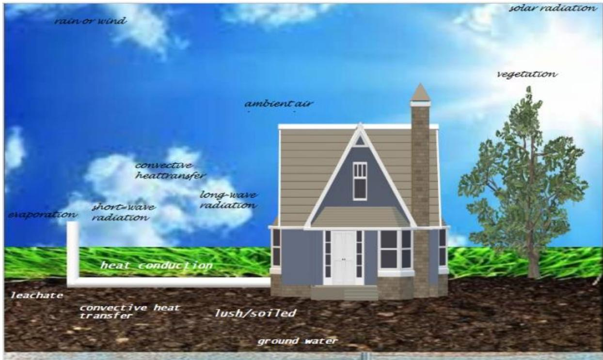
**Fig.1.** EAHE and main environmental and heat transfer mechanisms affecting system performance [1].
