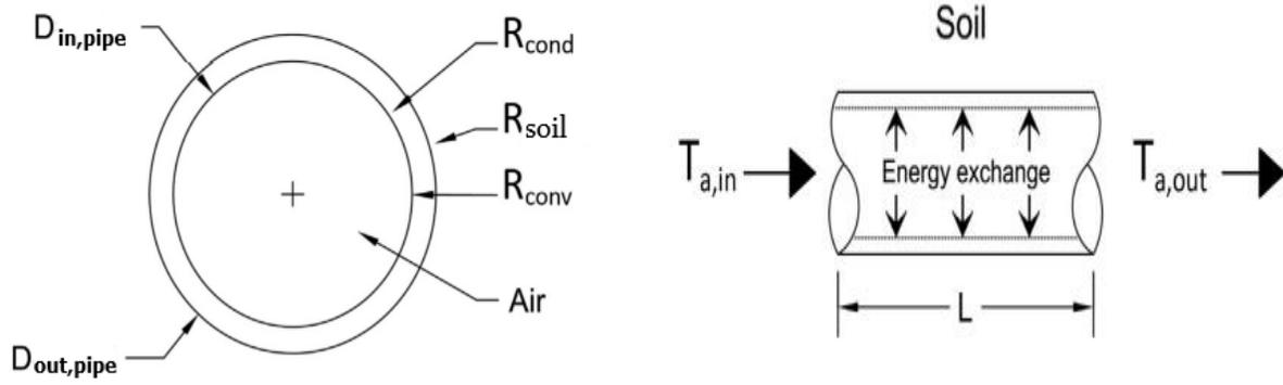
**Fig.III.10.** Schematic diagram of the modeled EAHE system [13].
