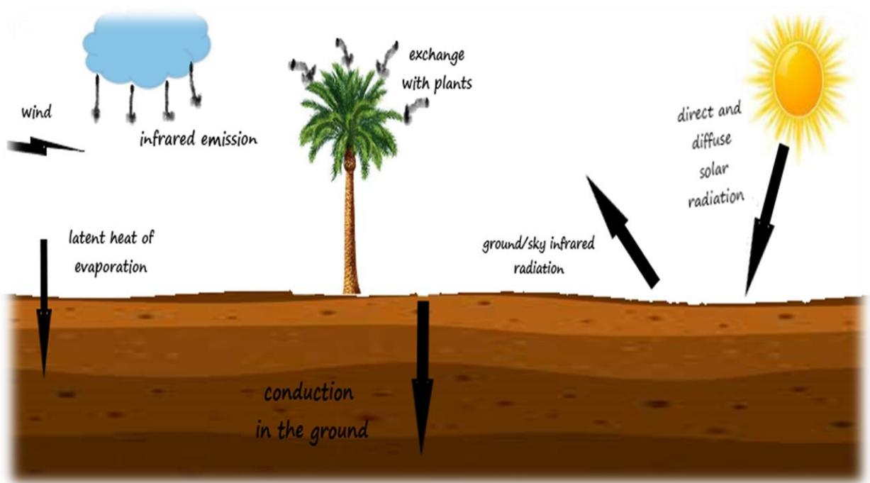
**Fig.III.1:** Major mechanisms of energy exchange at the soil–atmosphere interface.
