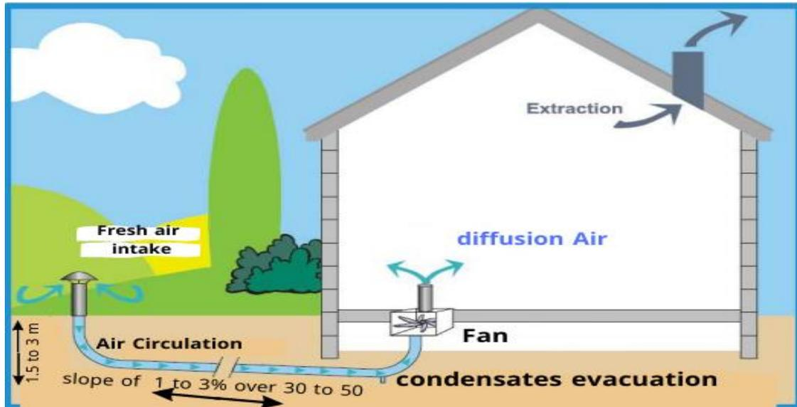
**Fig .II.1:** Simplified diagram of a single-tube Canadian well [2].
