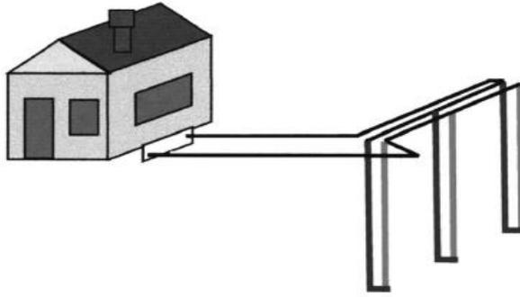
**Fig.II.7:** Vertical ground heat exchangers [5].
