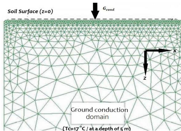
**Fig.IV.1.**Modelling of conductive transfer in soil.
