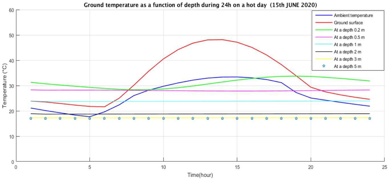
Fig.IV.12: Ground temperature as a function of depth 24h on hot day JUNE.
