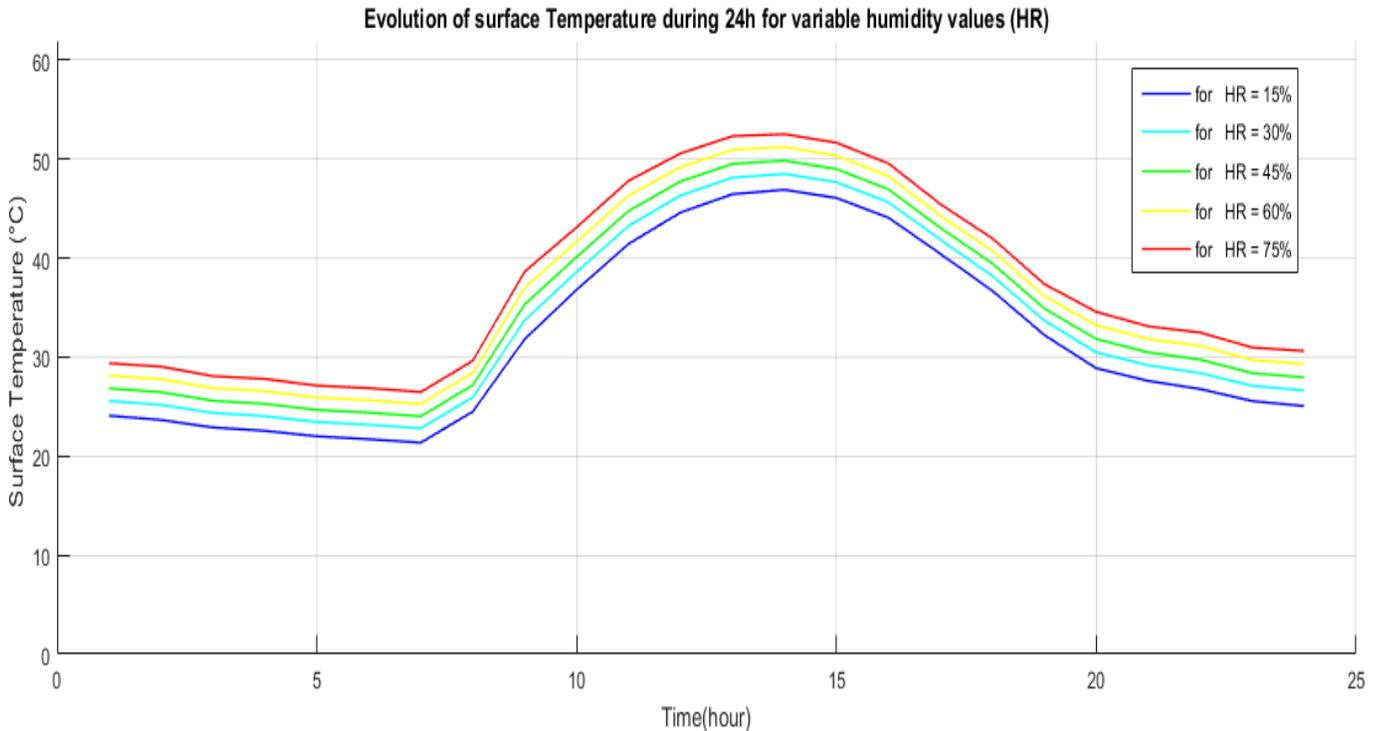
**Fig.IV.8:** Evolution of surface temperature during 24h for variable relative humidity values.
