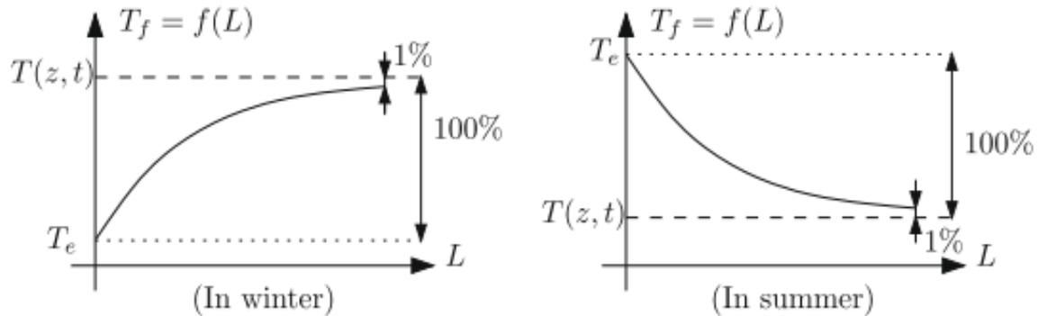
**Fig.III.11.** Evolution of the temperature air as a function of the length  $L$ , in winter and in summer [11].
