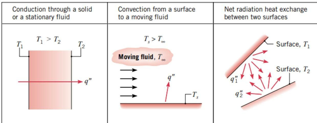
**Fig III.2:** Conduction, convection, and radiation heat transfer modes [1].
