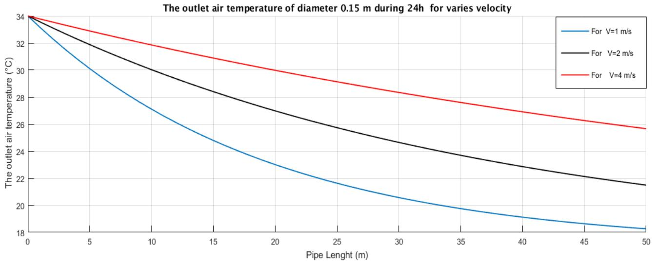
**Fig IV.18:** The outlet air temperature of diameter =0.15m for varies velocity of air.
