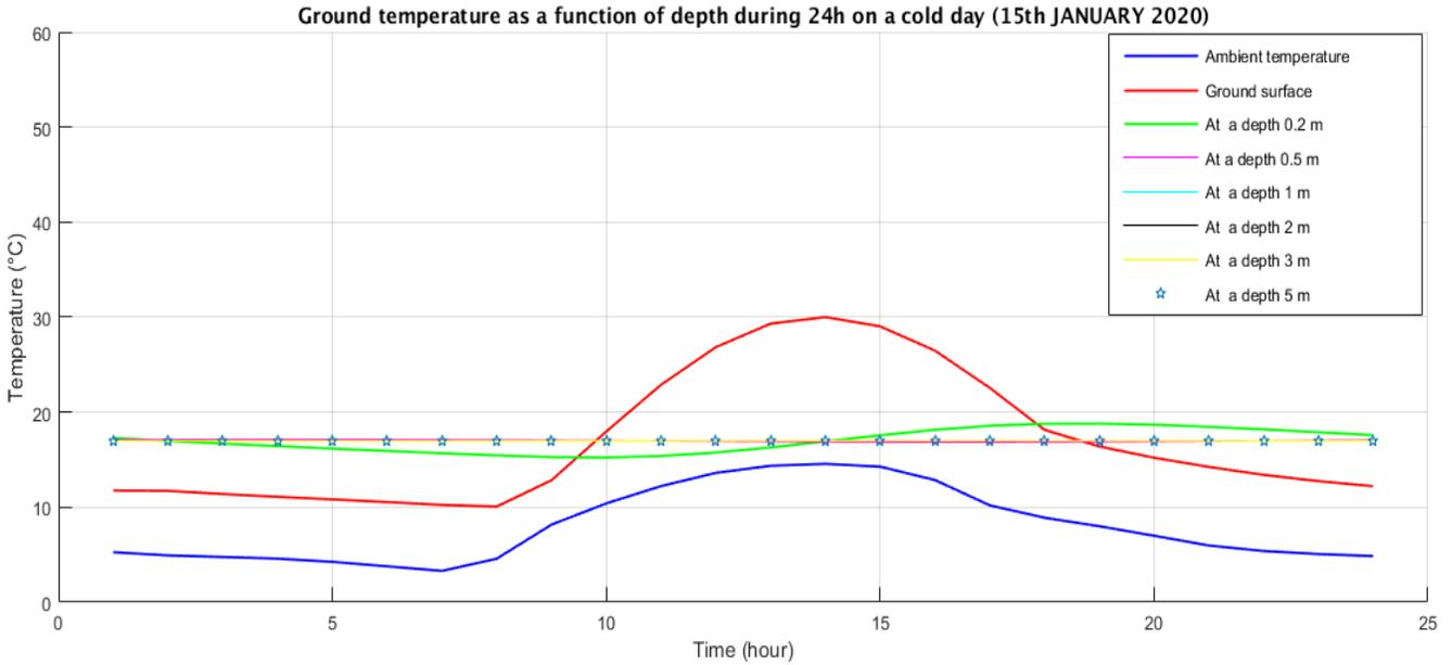
**Fig.IV.10:** Ground temperature as a function of depth 24h on cold day JANUARY.
