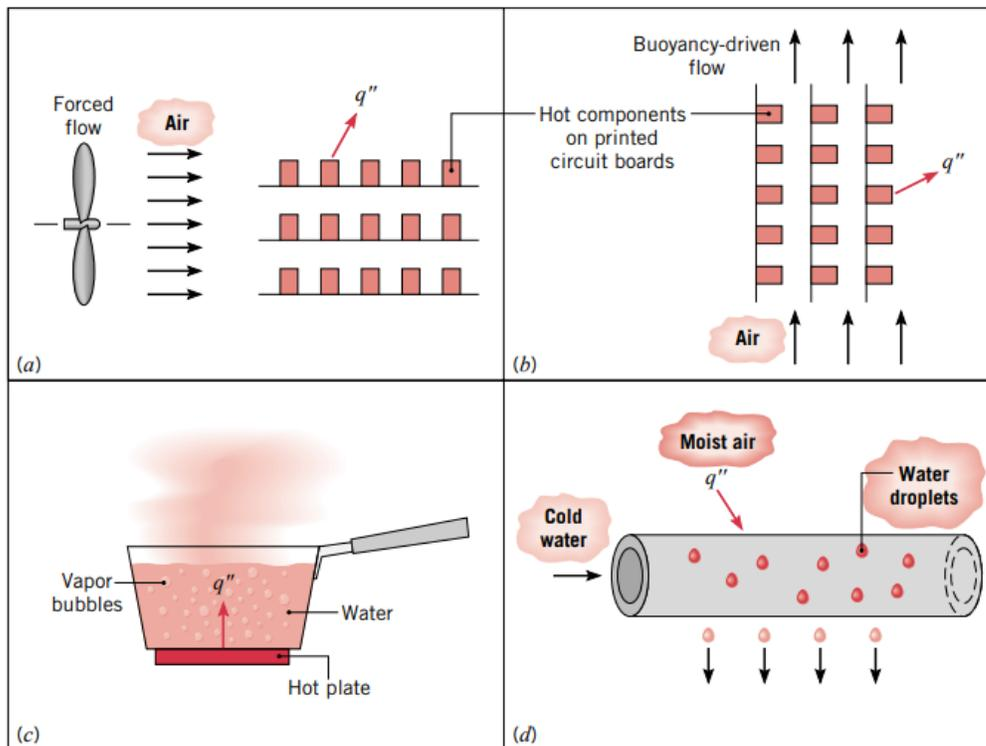
**Fig.III.5:** Convection heat transfer processes. **(a)** Forced convection. **(b)** Natural convection. **(c)** Boiling. **(d)** Condensation [1].
