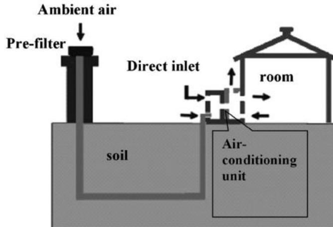
**Fig.II.4:** Basic principle of ground preheating or pre-cooling of air in an open system [5].
