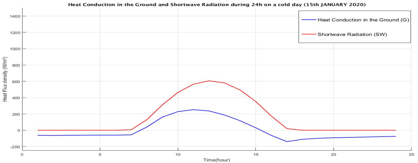
**Fig.IV.11:** Heat conduction in the ground and shortwave radiation during 24h on cold day JANUARY.
