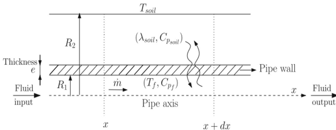
Fig.III.9.Schematic heat exchange between flowing fluid and ground. [10]
