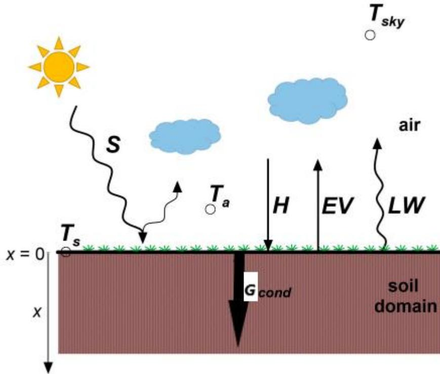
Fig.III.8: Heat fluxes on the surface of the ground [7].
