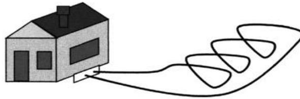
**Fig.II.6:** “Slinky” type ground heat exchanger [5].
