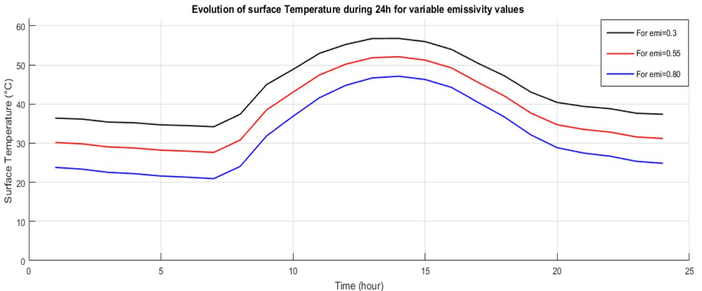
**Fig.IV.7:** Evolution of surface temperature during 24h for variable emissivity values.
