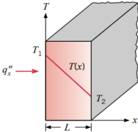
**Fig.III.3:** One-dimensional heat transfer by conduction (diffusion of energy) [1].
