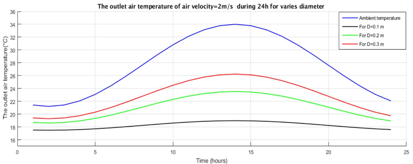
**Fig IV.21:** Ambient and outlet air temperatures (EAHE) system during 24h for varies diameter.
