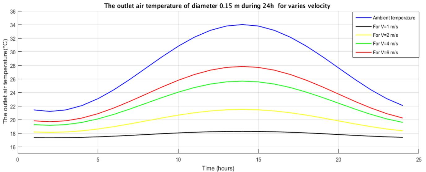
**Fig.IV.19:** Ambient and outlet air temperatures (EAHE) system during 24h for varies velocity.
