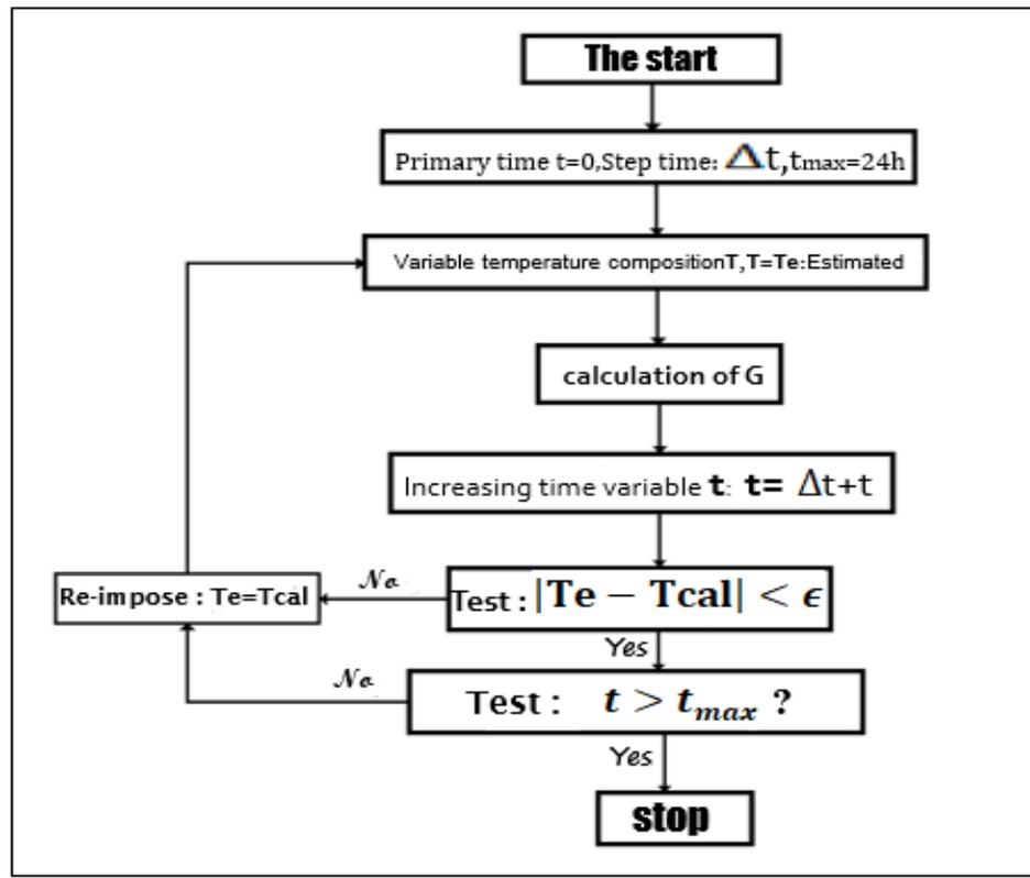
Fig.IV.3: Calculation algorithm within 24 hours.
