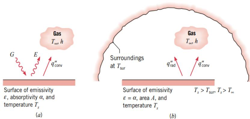
**Fig.III.6:** Radiation exchange, (a) at a surface and (b) between a surface and large surroundings [1].
