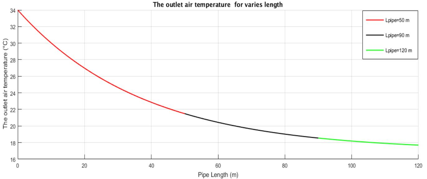
Fig IV.16: The outlet air temperature of velocity =2m/s for varies length of pipe
