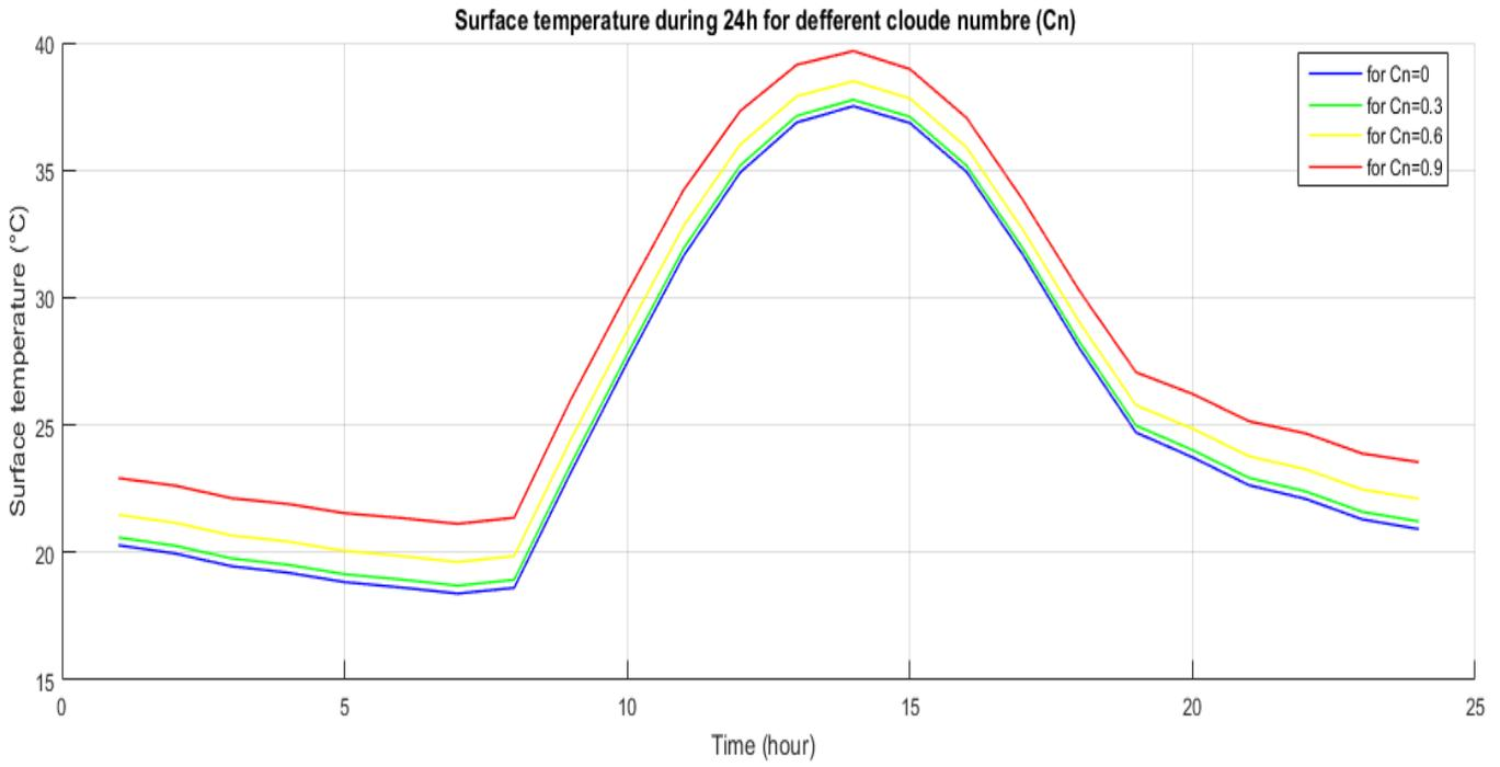
**Fig.IV.9:** Evolution of surface temperature during 24h for variable cloud number values.
