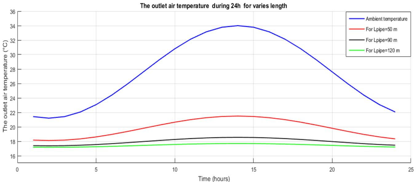
Fig IV.17: Ambient and outlet air temperatures (EAHE) system during 24h for varies length.
