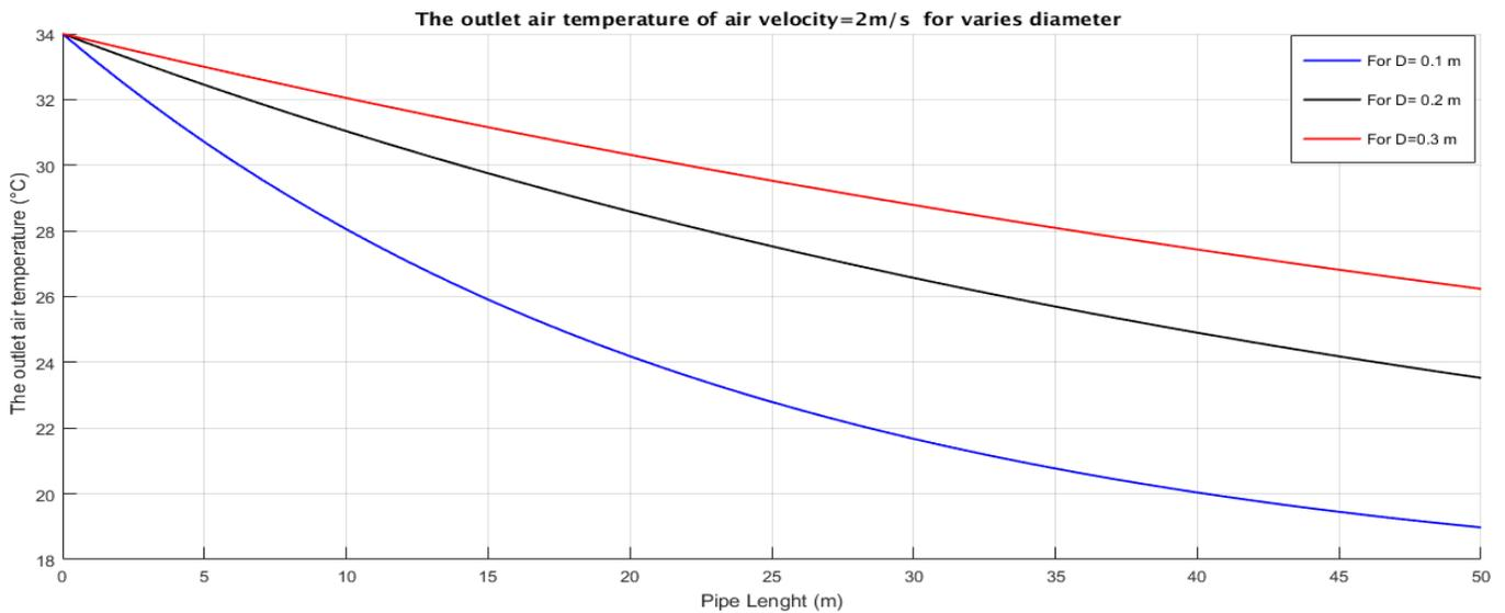
**Fig.IV.20:** The outlet air temperature of velocity =2m/s for varies diameter
