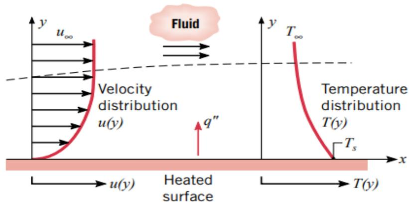
**Fig.III.4:** Boundary layer development in convection heat transfer [1].
