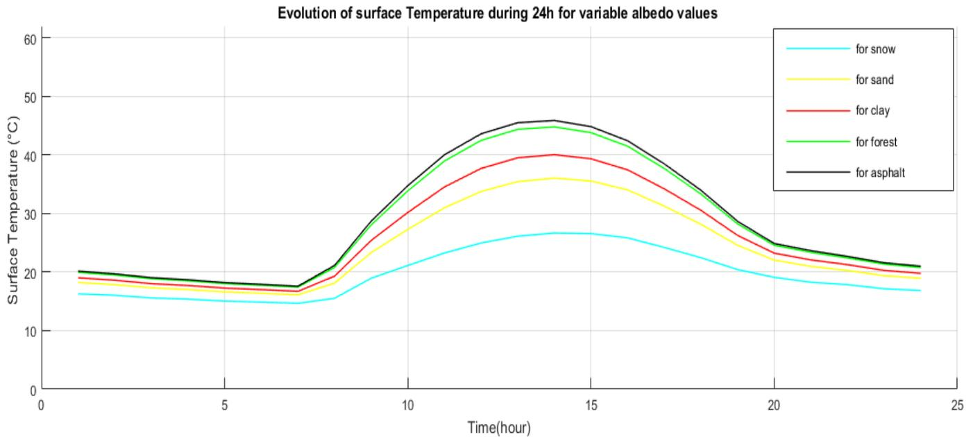
**Fig.IV.5:** Evolution of surface temperature during 24h for variable albedo values.
