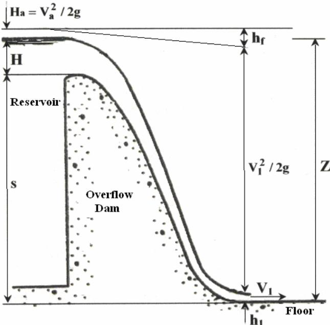
Fig.1. Components for writing the functional relationship  $f(Z, H, h_1) = 0$
