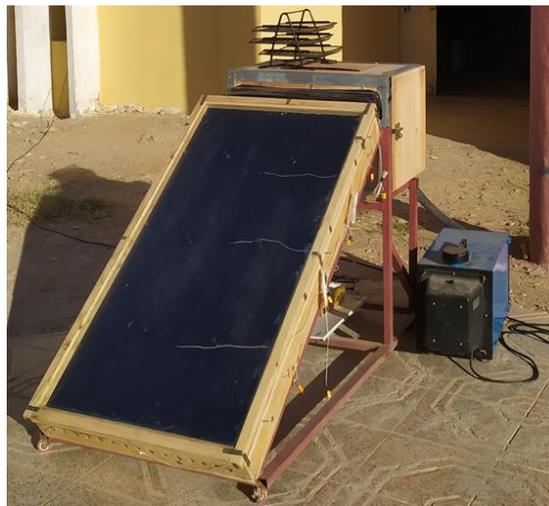
Figure III.3: Experimental setup (solar collector with drying chamber and air suction motor)
