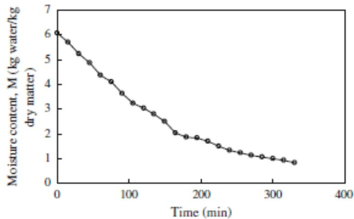
**Figure II.10:** Moisture content versus drying time for potato cylinders dried in indirect solar dryer [5].
