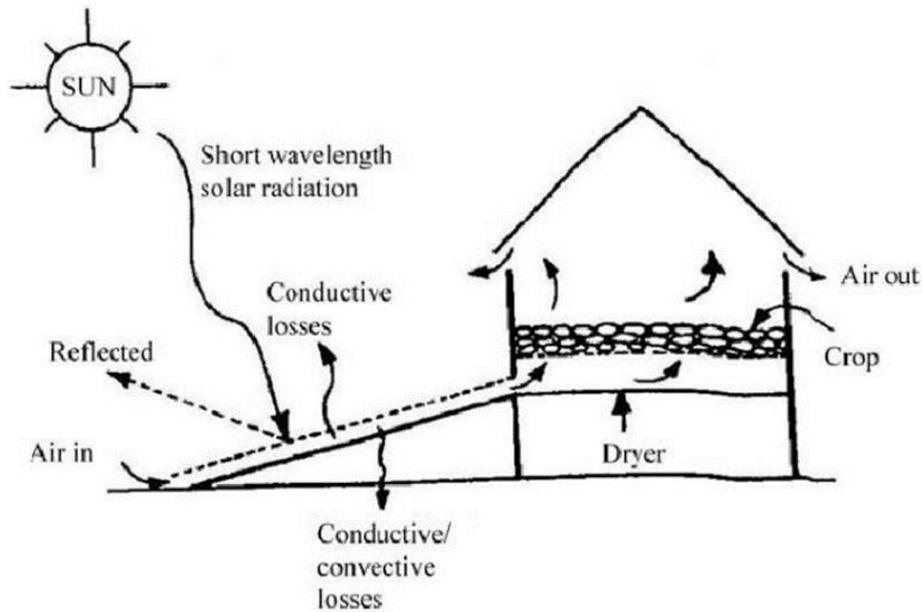
**Figure I.7:** Indirect solar dryer [11].
