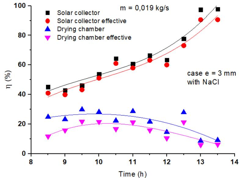
**Figure IV.24:** Performance of the solar collector and drying room with air flows 0.019 kg/s.
