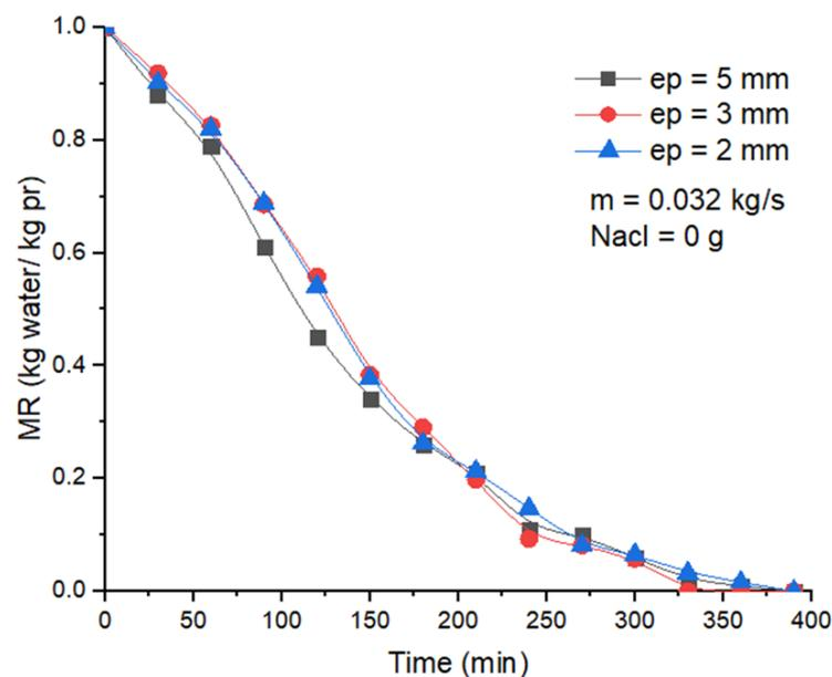
**Figure IV.3:** Moisture Ratio vs Drying Time for Different Models of 2,3 and 5mm Thickness Potato Chips, with air flows 0,032 kg/s (C).
