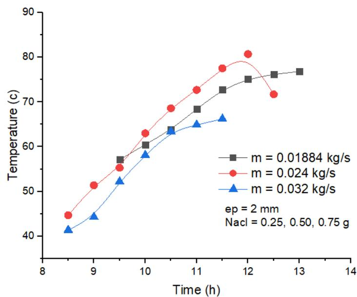
**Figure IV.9:** potato drying temperatures for samples 2 mm with three different air flows, with three different amounts of salt for this sample.
