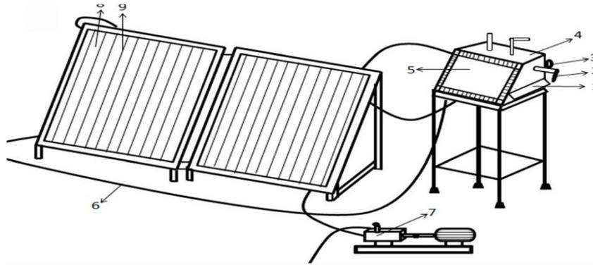
**Figure II.34:** Vacuum-assisted solar drying system (a) schematic diagram where (1) drying chamber (2) vacuum release valve (3) vacuum gauge (4) storage tank (5) drying chamber glass cover (6) pipe (7) water ring vacuum pump (8) solar collector (9) riser pipe, and (b) photograph of the drying set up [12].
