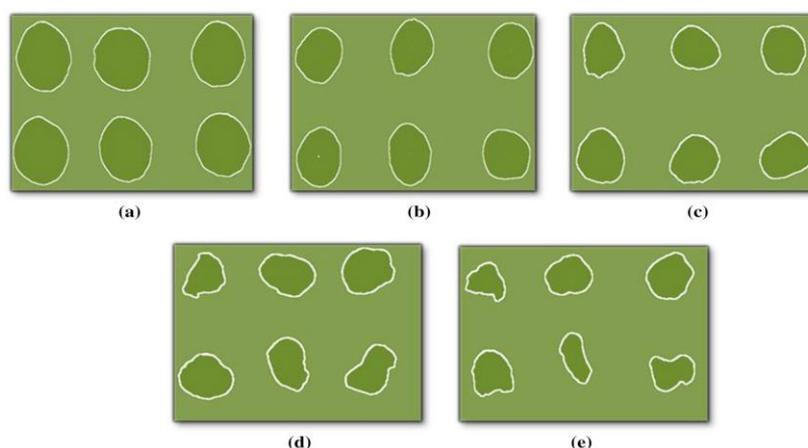
**Figure II.33:** Binary images of turmeric slices (25 mm diameter and 6 mm thickness) at drying time of a 0, b 60, c 120, d 180 and e 240 min, respectively [11].
