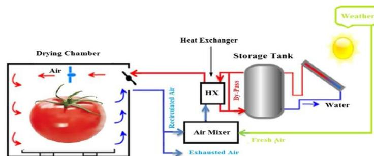
Figure II.7: Simplified schematic of the solar tomato dryer installation [4].
