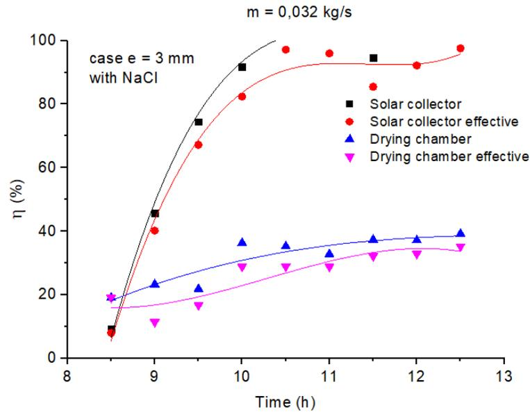
**Figure IV.26:** Performance of the solar collector and drying room with air flows 0.032 kg/s.
