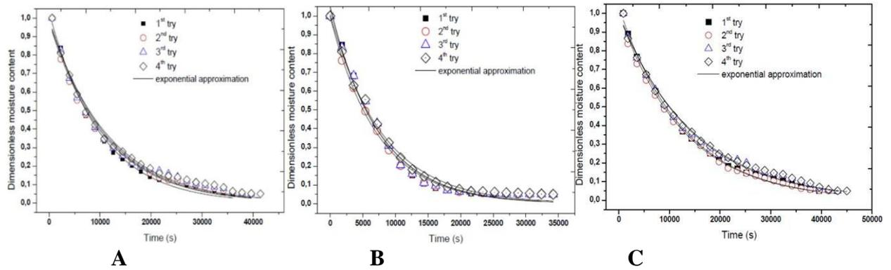
**Figure II.41:** Experimental with exponential approximation average dimensionless moisture ratio vs drying time for the four try of A: cube and B: disc and C: paralyses shape [15].
