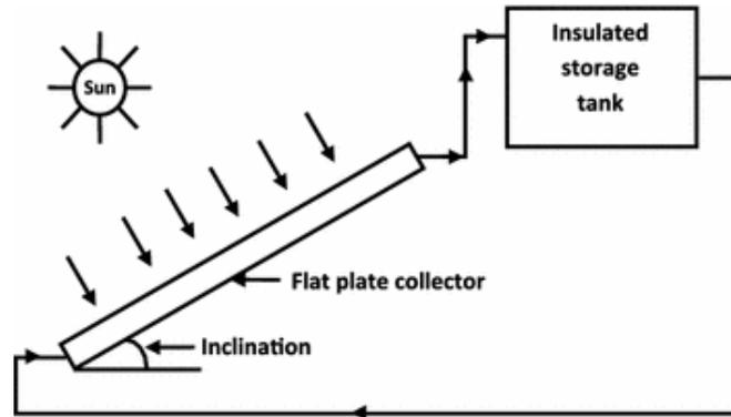
**Figure I.13:** operation of a flat solar collector [18].
