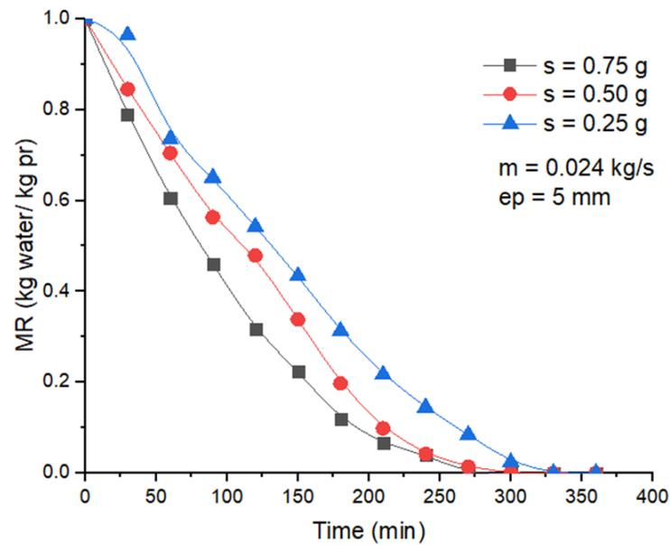
**Figure IV.17:** Moisture versus drying time of 5 mm thick potato chips with air flows 0,024 kg/s (B).
