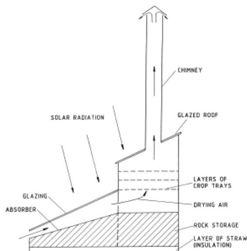
**Figure I.9:** Mixed solar dryer [6].
