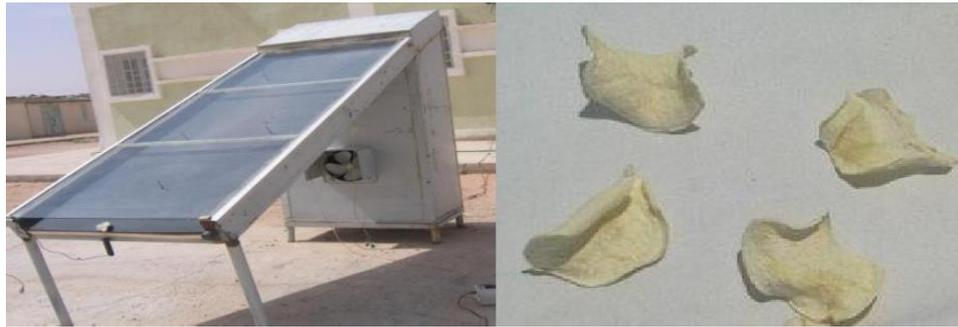
**Figure II.29:** Schematic of the drying system and Visual quality of the dried potato [10].
