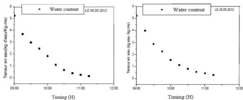
**Figure II.30:** variation of water content as function of time associate with one panel (a) and two panels (b) [10].
