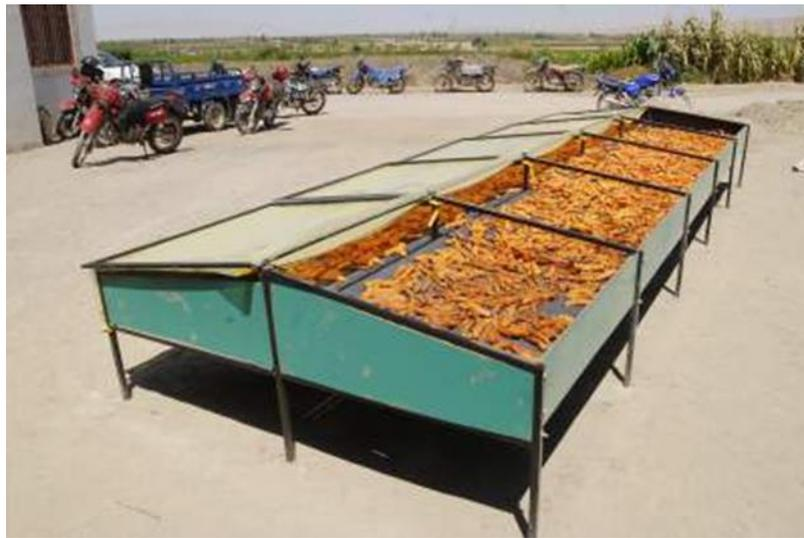
**Figure I.3:** Direct Solar dryers [7].
