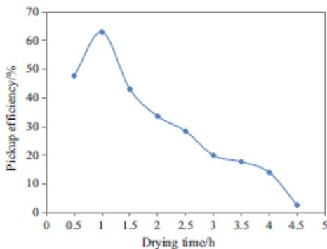
Figure II.19: Variation of pickup efficiency over drying time [7].
