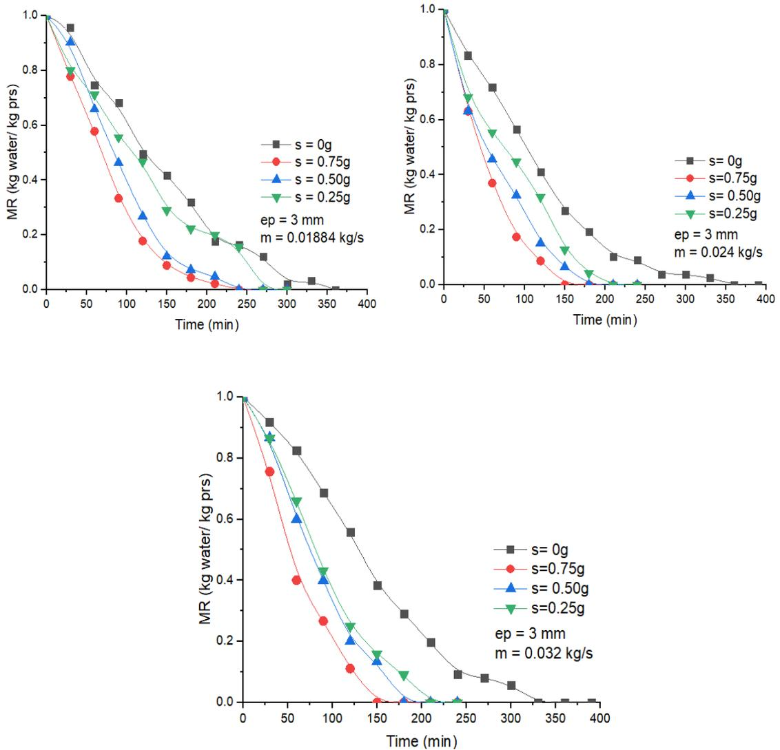
**Figure IV.22:** Moisture ratio versus drying time for 3 mm thick potato chips with three different air flows 0.01884, 0.024, 0.032 kg/s with amounts of salt 0 g, 0.75g, 0.50g, 0.25g.
