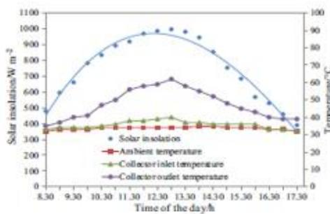
Figure II.17: Variations of solar insolation thermal and temperature [7].
