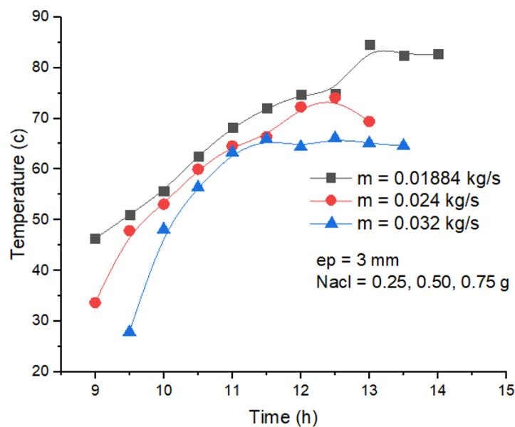
**Figure IV.14:** potato drying temperatures for samples 3 mm with three different air flows, with three different amounts of salt for this sample.
