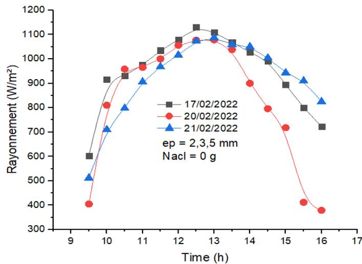
**Figure IV.5:** Variation of solar radiation intensity in 1-3 days of potato drying for three different samples.
