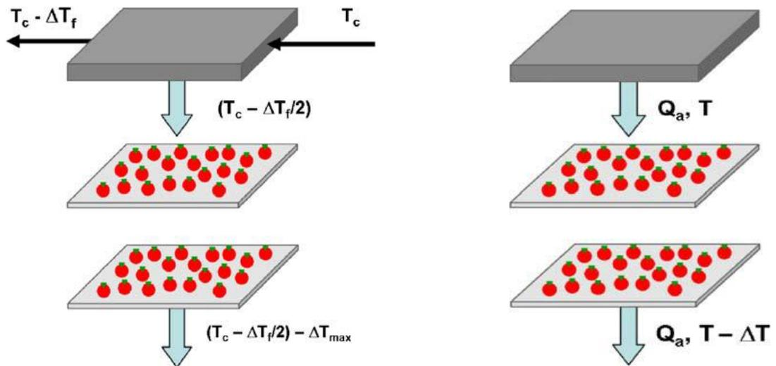
**Figure II.36:** Minimum outlet temperature if the radiators are perfect heat exchangers and Temperature drop in a drying zone between two radiators [13].
