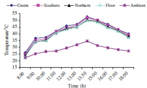
**Figure II.24:** Temperature variation at full load [8].
