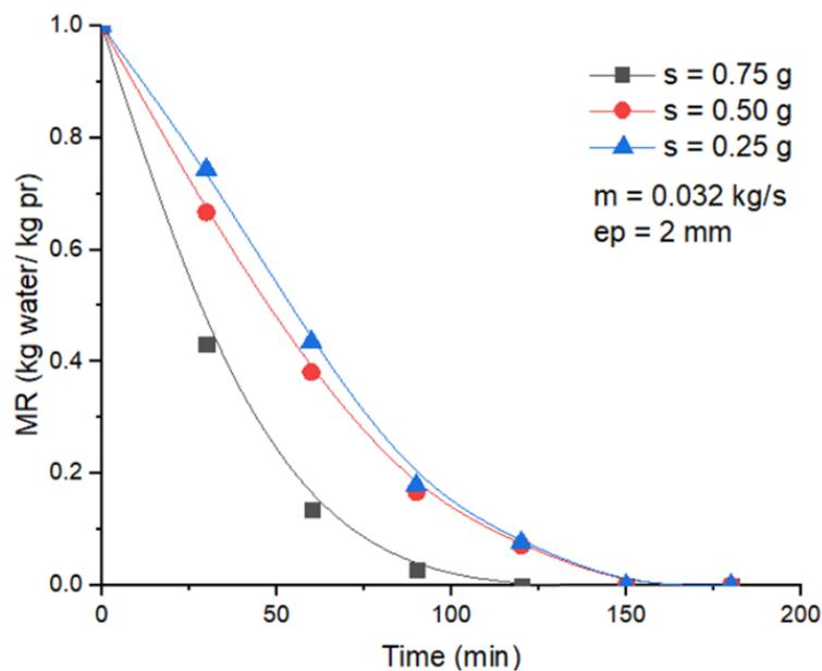
**Figure IV.8:** Moisture versus drying time of 2 mm thick potato chips with air flows 0,032 kg/s (C).
