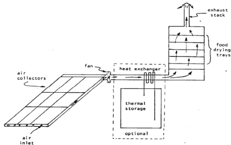
**Figure I.8:** Hybrid Solar Dryer [6].
