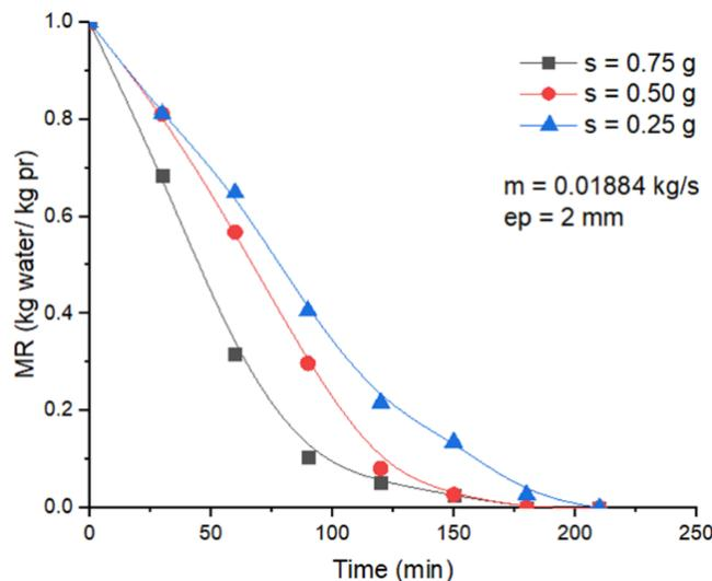
**Figure IV.6:** Moisture versus drying time of 2 mm thick potato chips with air flows 0,01884 kg/s (A).
