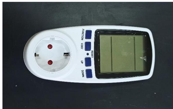
**Figure III.19:** A device for measuring electrical power in watts.
