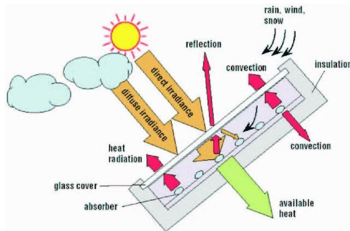
Figure I.11: Diagram of a flat air collector [14].
