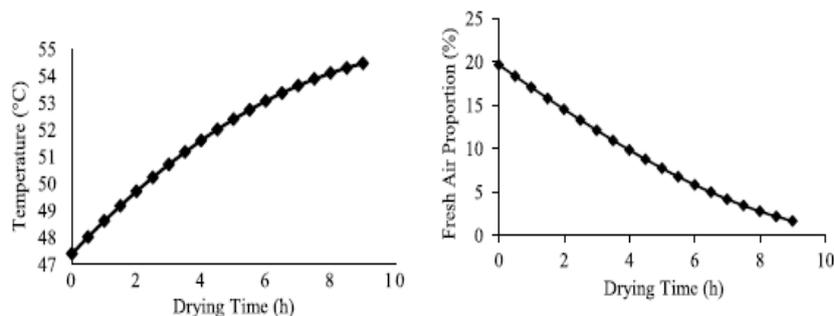
Figure II.8: Outlet Temperature and example of calculated fresh ambient air proportions admitted in the mixing chamber during drying air [4].
