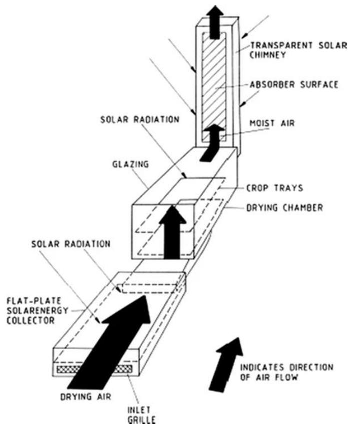
Figure I.5: Integral solar dryer [9].
