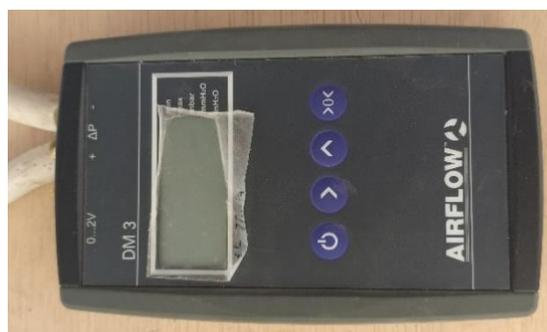
**Figure III.20:** Air loss measuring device (DM3).
