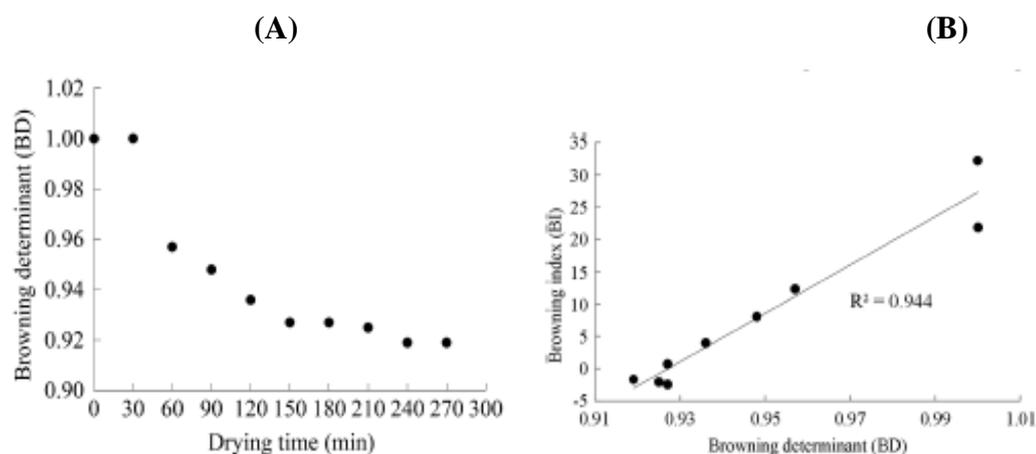
**Figure II.32:** A: Variation in BD of turmeric slices during direct solar drying.
