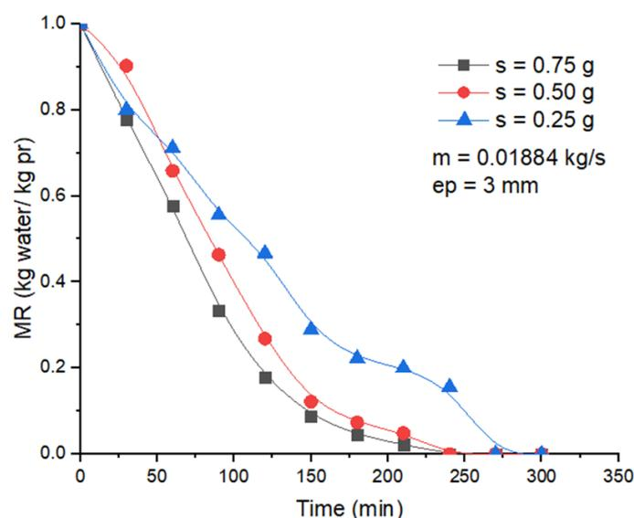
**Figure IV.11:** Moisture versus drying time of 3 mm thick potato chips with air flows  $0,01884 \text{ kg/s}$  (A).
