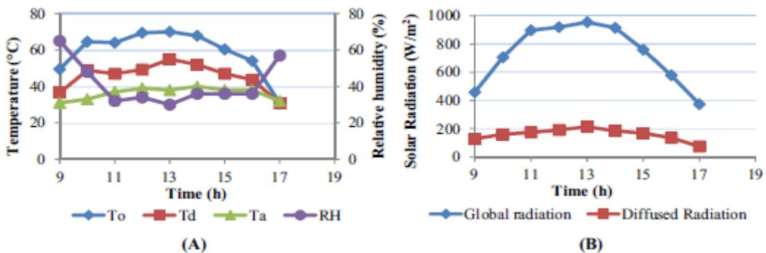
**Figure II.12:** Temperature (a) relative humidity and solar radiation (b) variation along the day [6].
