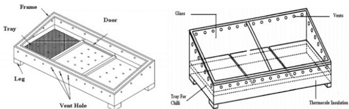
**Figure I.4:** Box of a direct solar dryer [8].
