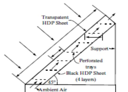
**Figure II.28:** Side view of farm solar dryer [9].
