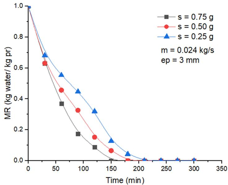
**Figure IV.12:** Moisture versus drying time of 3 mm thick potato chips with air flows 0,024kg/s (B).
