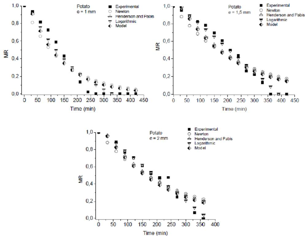
**Figure II.2:** The moisture ratio versus drying time for different models of potato slices with 1,1.5, and 2mm of thickness [1].
