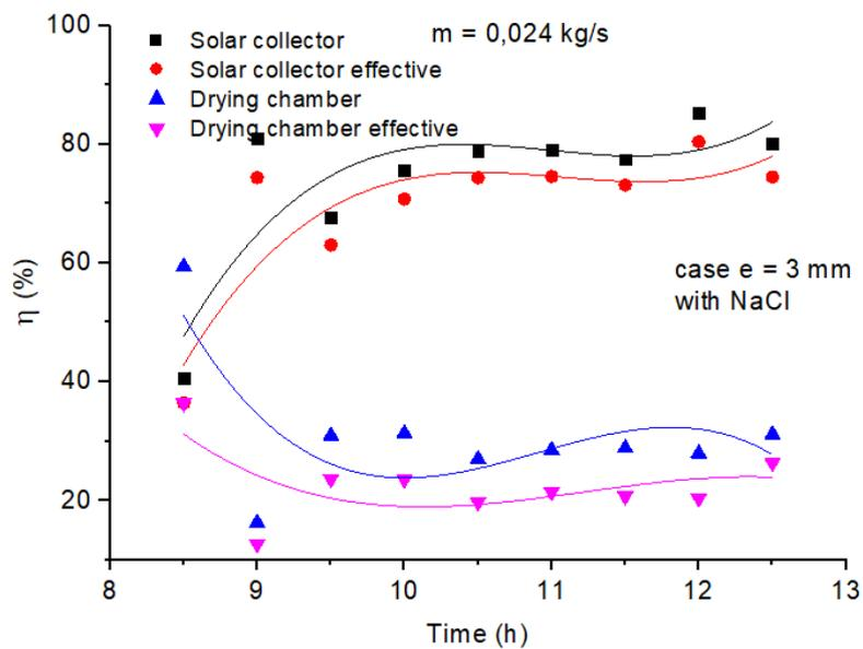
**Figure IV.25:** Performance of the solar collector and drying room with air flows 0.024 kg/s.
