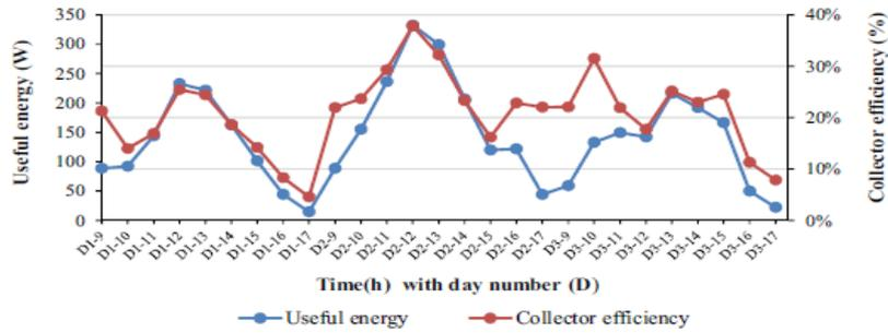
Figure II.14: Energy gained from the collector and thermal efficiency with drying time [6].
