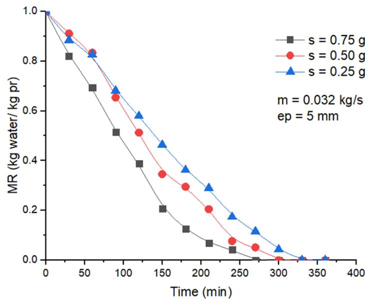
**Figure IV.18:** Moisture versus drying time of 5 mm thick potato chips with air flows 0,032 kg/s (C).
