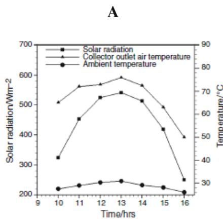
**Figure II.38:** Variation of solar radiation , ambient temperature and collector outlet air temperature with time of day (December month) for experimental run during drying of fenugreek leaves [14].
