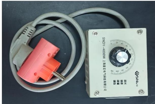
**Figure III.17:** Voltage regulator (AC 220V 4000W).
