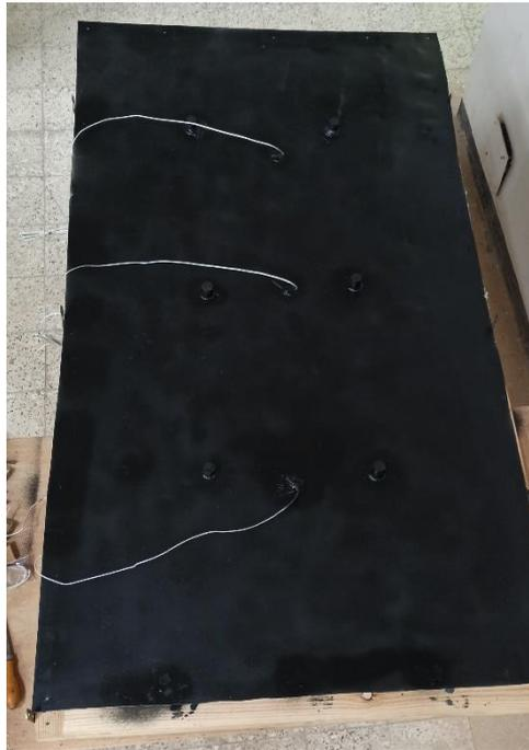
**Figure III.4:** Thermal pickup locations.
