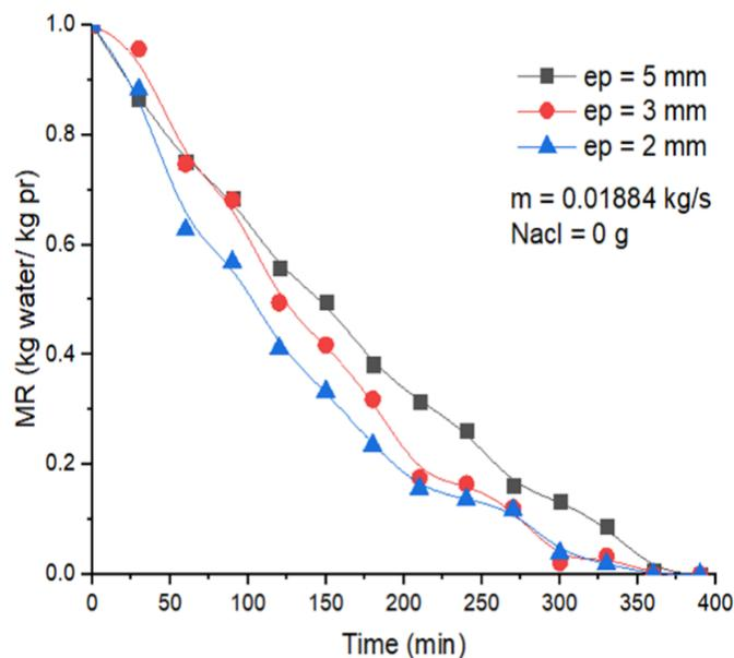
**Figure IV.1:** Moisture Ratio vs Drying Time for Different Models of 2,3 and 5mm Thickness Potato Chips, with air flows 0,01884 kg/s (A).
