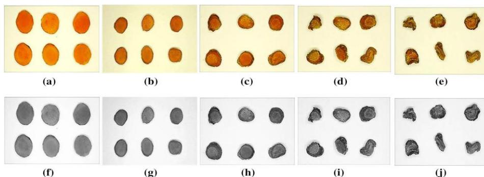
**Figure II.31:** RGB and Gray scale images of turmeric slices at different moisture content (w b) a and f 93.5%, b and g 39.39%, c and h 16.46%, d and I 3.90%, e and j 3.46% [11].
