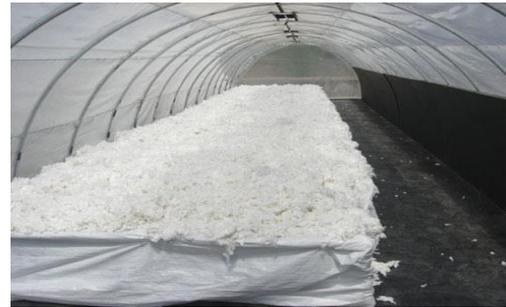
**Figure II.22:** Inside view of solar Tunnel dryer [8].
