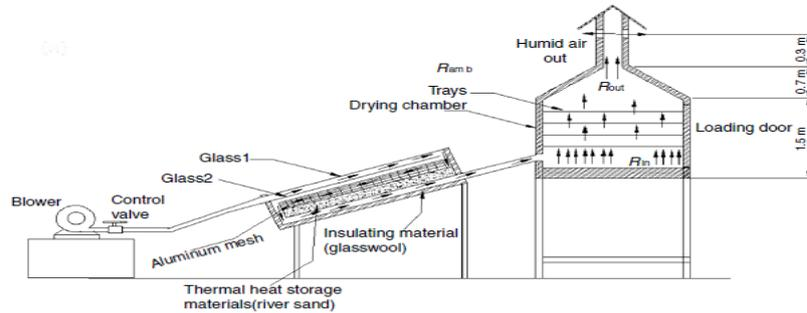
Figure II.16: Planned view of the experimental setup [7].
