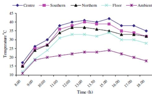
**Figure II.23:** Temperature variation at no full load [8].
