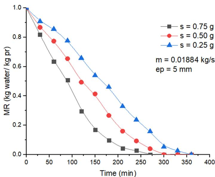
**Figure IV.16:** Moisture versus drying time of 5 mm thick potato chips with air flows  $0,01884 \text{ kg/s}$  (A).
