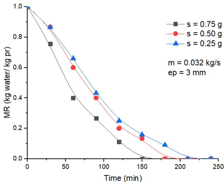
**Figure IV.13:** Moisture versus drying time of 2 mm thick potato chips with air flows 0,032 kg/s (C).
