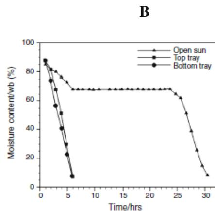
**Figure II.39:** Hourly variation of moisture content at different trays (top, bottom and open) with drying Time of fenugreek leaves [14].
