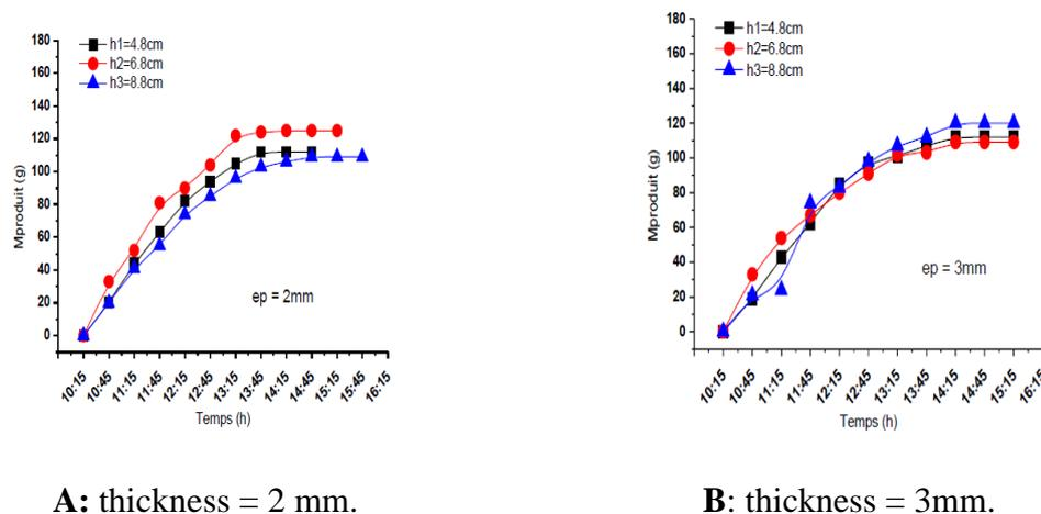
Figure II.6: Variation of liquid mass loss durin the drying time of the potatoes thickness= 2 mm and thickness = 3mm, flow rate = 0.01 kg/s [3].
