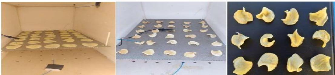
Figure II.5: Wet and dried potato slices 2 mm thick, 40mm in diameter, flow rate 0.011 Kg/s grid height 4.8 cm [3].
