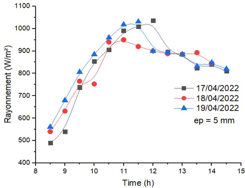
**Figure IV.20:** Variation of the intensity of solar radiation in 1-3 days of drying potatoes for a sample with a thickness of 5 mm.
