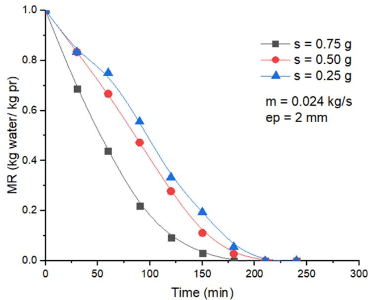
**Figure IV.7:** Moisture versus drying time of 2 mm thick potato chips with air flows 0,024kg/s (B).
