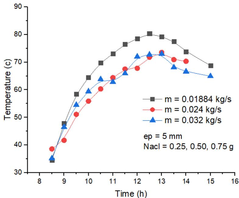
**Figure IV.19:** potato drying temperatures for samples 5 mm with three different air flows, with three different amounts of salt for this sample.
