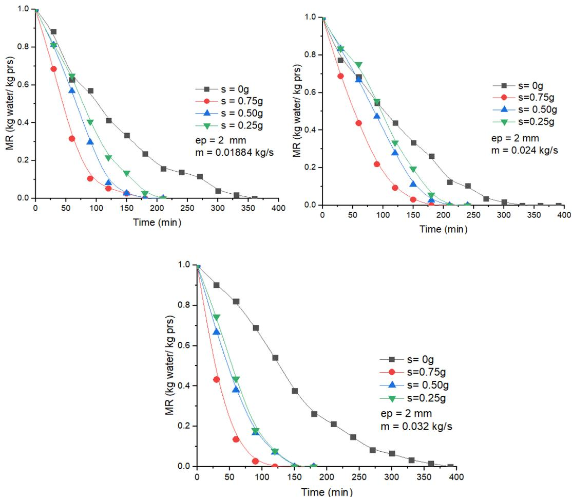
**Figure IV.21:** Moisture ratio versus drying time for 2 mm thick potato chips with three different air flows 0.01884, 0.024, 0.032 kg/s with amounts of salt 0 g, 0.75g, 0.50g, 0.25g.
