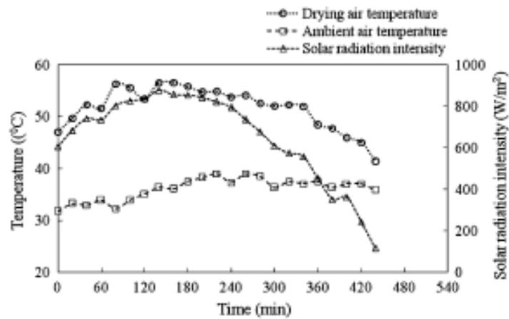
**Figure II.9:** Variation in drying air temperature, ambient air Temperature with solar radiation under no load condition [5].
