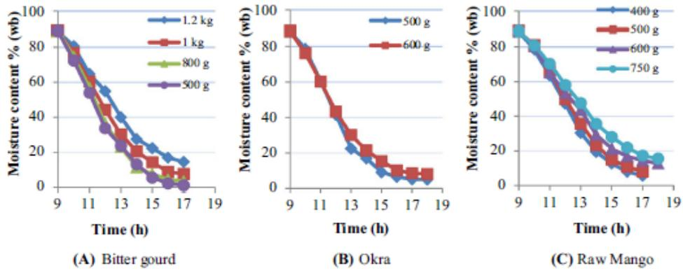
Figure II.13: Variation of moisture content of solar-dried products with drying time for varying loads. a Bitter gourd, b okra, and c raw mango [6].
