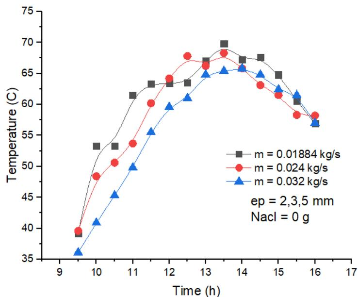
**Figure IV.4:** potato drying temperatures for three different samples 2,3,5 mm with three different air flows.
