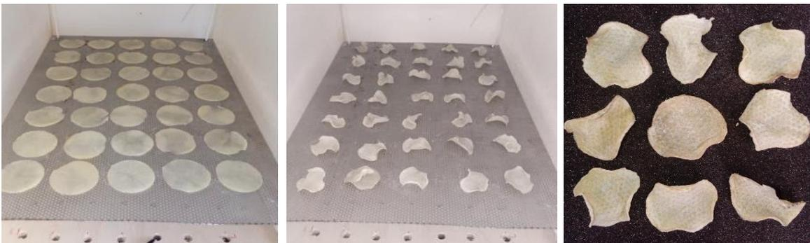
**Figure II.1:** Wet and dried slices of potato with 1mm of thickness and 44 mm of diameter [1].
