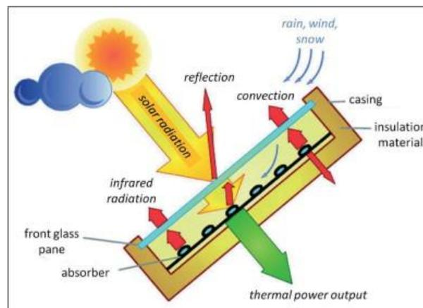
Figure I.12: principle of a flat solar collector [16].
