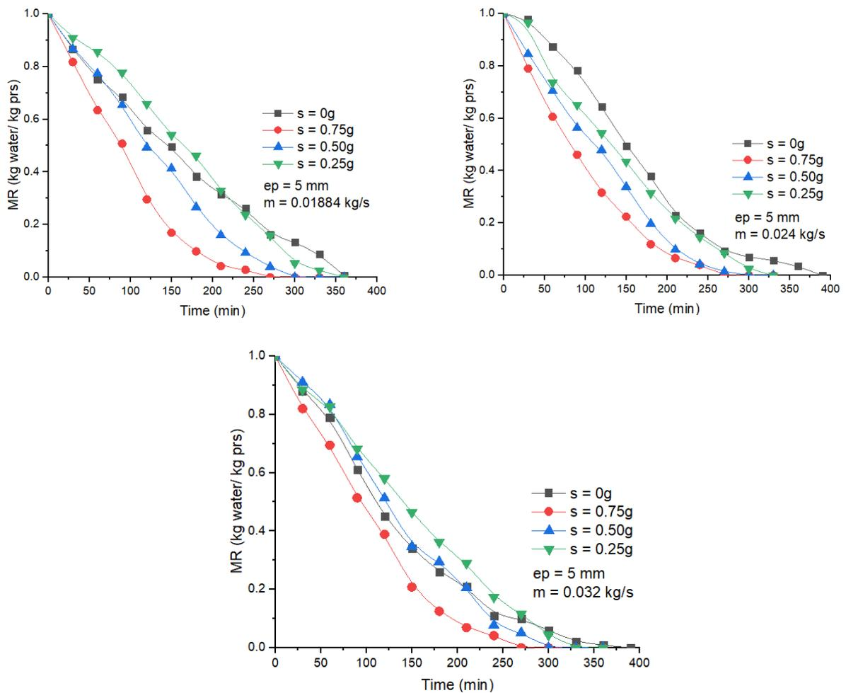
**Figure IV.23:** Moisture ratio versus drying time for 5 mm thick potato chips with three different air flows 0.01884, 0.024, 0.032 kg/s with amounts of salt 0 g, 0.75g, 0.50g, 0.25g.
