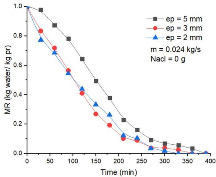
**Figure IV.2:** Moisture Ratio vs Drying Time for Different Models of 2,3 and 5mm Thickness Potato Chips, with air flows 0,024 kg/s (B).
