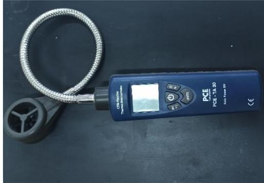
**Figure III.16:** A digital anemometer (Model PCE-TA30).
