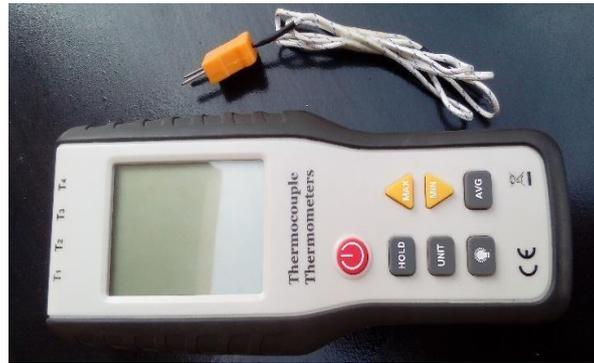
**Figure III.13:** A thermocouples type k.
