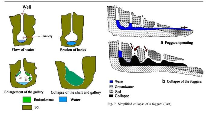
Fig. 5 Simplified collapse of foggara (slow) (Remini 2004)
