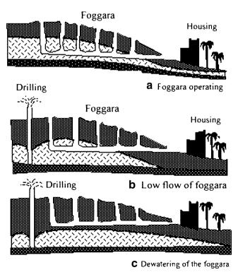
Fig. 11 Simplified diagram of a drying foggara
