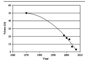
Fig. 14 El Meghier's Foggara flow evolution in time (Remini and Achour 2008)
