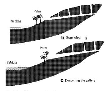
Fig. 9 Simplified process of flushing
