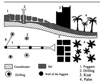
Fig. 12 Schematic overview of the state near the drilling foggara
