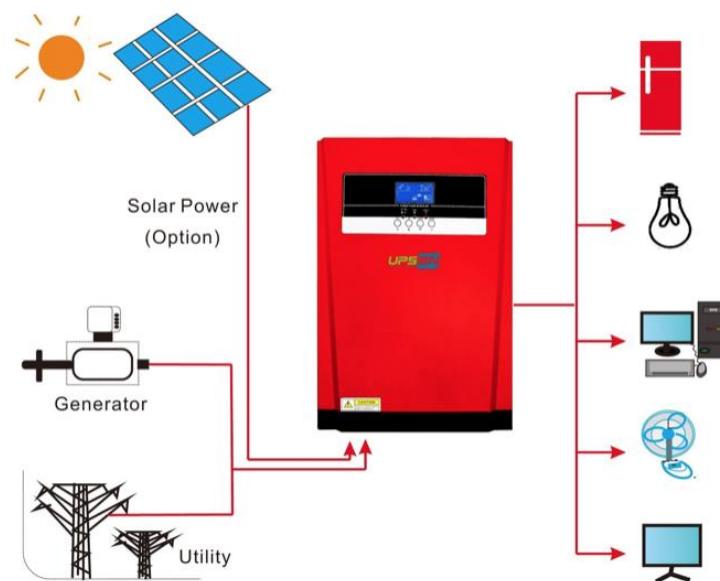
Figure 8: Installation of Hybrid inverters [ROM 21]
