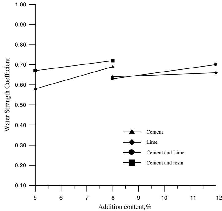
Fig. 4. Effect of additions on the water strength coefficient.
