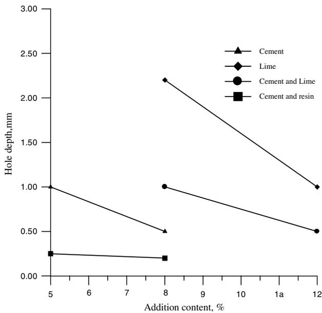
Fig. 7. Effect of additions on the hole depth – Spray test.
