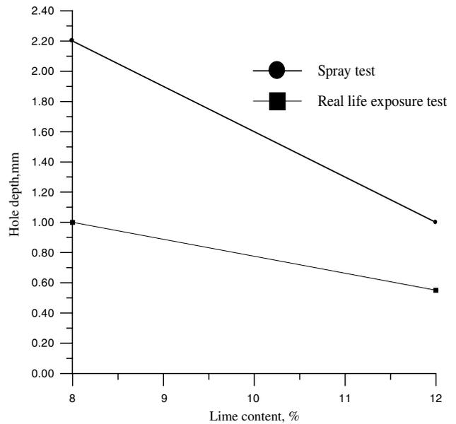
Fig. 8. Effect of lime content on the hole depth.
