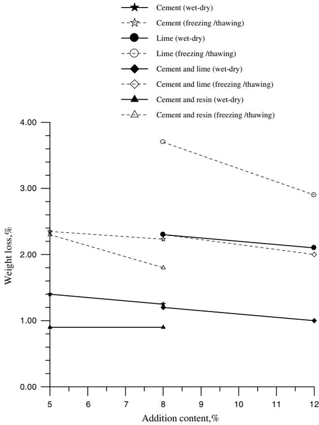
Fig. 6. Effect of additions on the weight loss.
