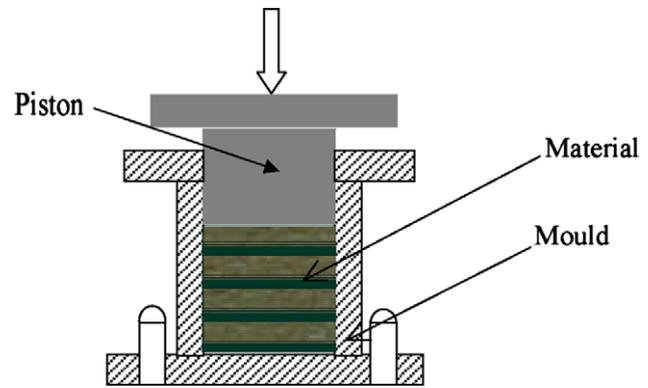
Fig. 1. Mould used for bricks making.
