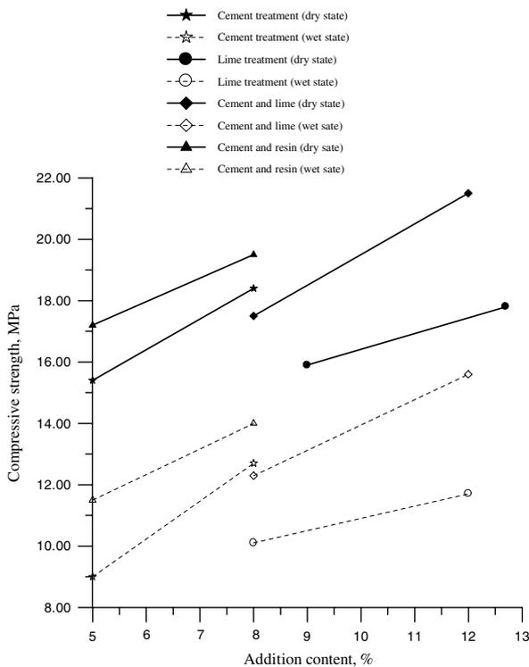
Fig. 3. Effect of additions on the compressive strength.
