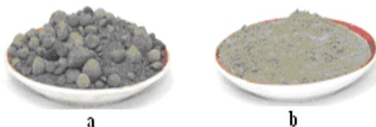
Figure 1. Clinker, a: Before crushing, b: After crushing
