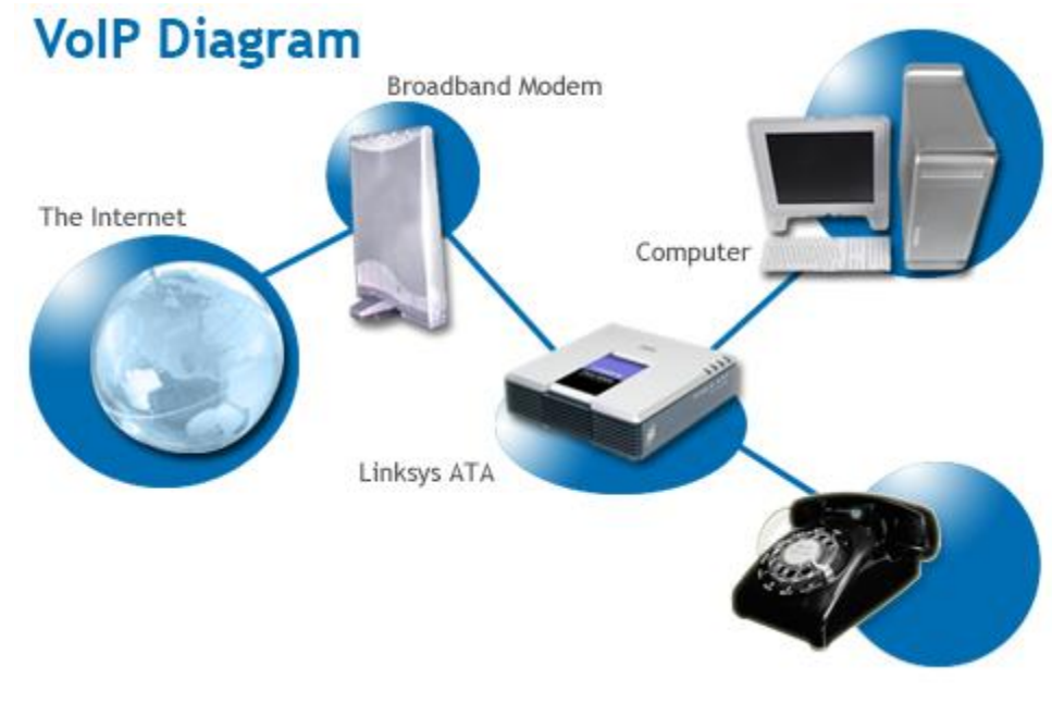
Figure 2.8 : Analogue Terminal Adapter.[54]
