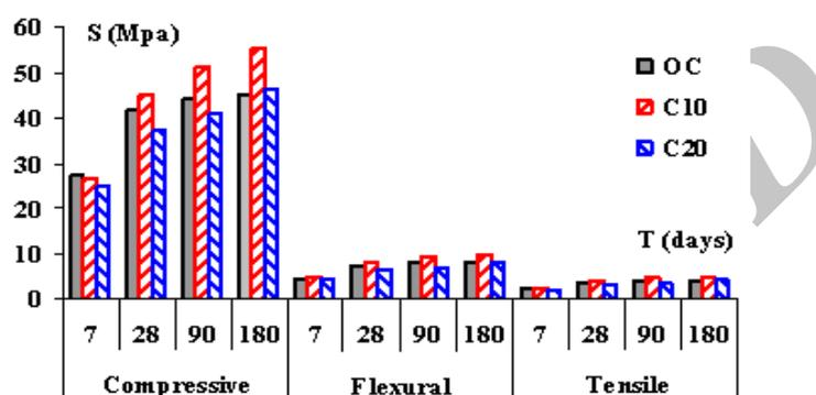
Figure 8. Compressive strength, flexural and tensile strength of concrete as a function of time
