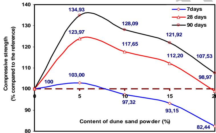
Figure 5. Effect of content of dune sand powder on the compressive strength ( $w/b = 0.25$ ) [23]
