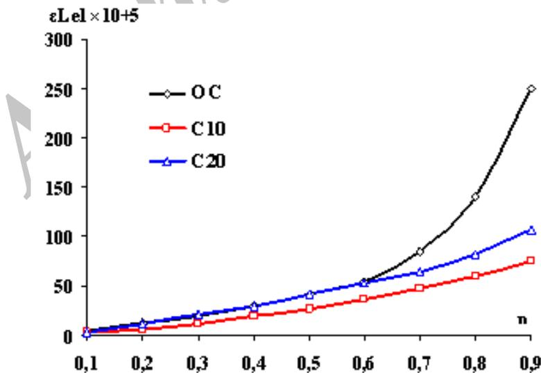
Figure 10. Elasto-instantaneous strain longitudinal of concrete as a function of relative stresses
