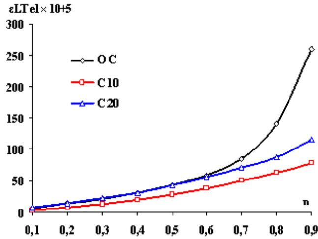
Figure 11 Elasto-instantaneous strain total longitudinal of concrete as a function of relative stresses
