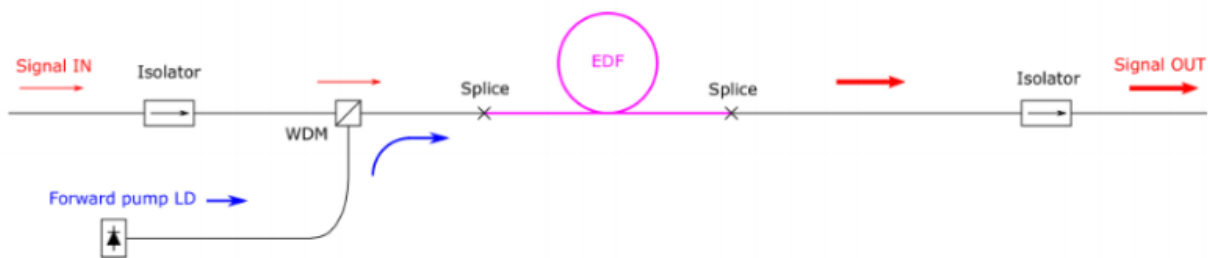
Figure 1.11: EDFA block diagram [4]
