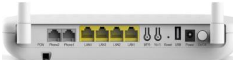
Figure 2.14: The rear panel of the ZXHN F660. [29]
