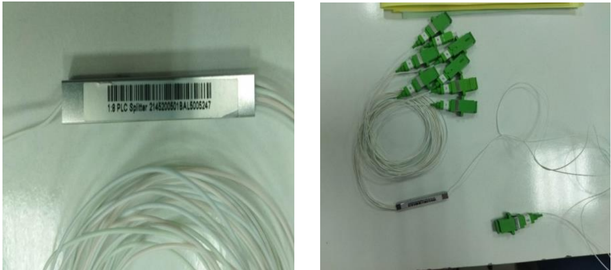
Figure 2.9: 1:8 PLC fiber splitter steel tube bare fibers 250µm. [Algerie telecom]
