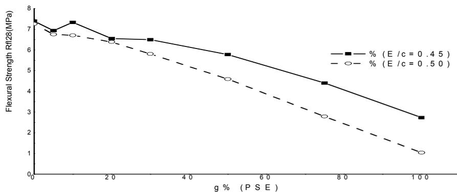
Fig. 3.: Evolution of the flexural strength at 28days according to the content of polystyrene aggregates and  $E/C = 0.45$  &  $0.5$
