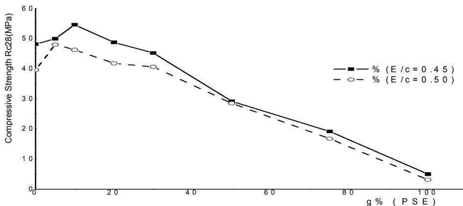
Fig. 2: Evolution of the compressive strength at 28days according to the content of polystyrene for  $E/C = 0.45$  &  $0.5$
