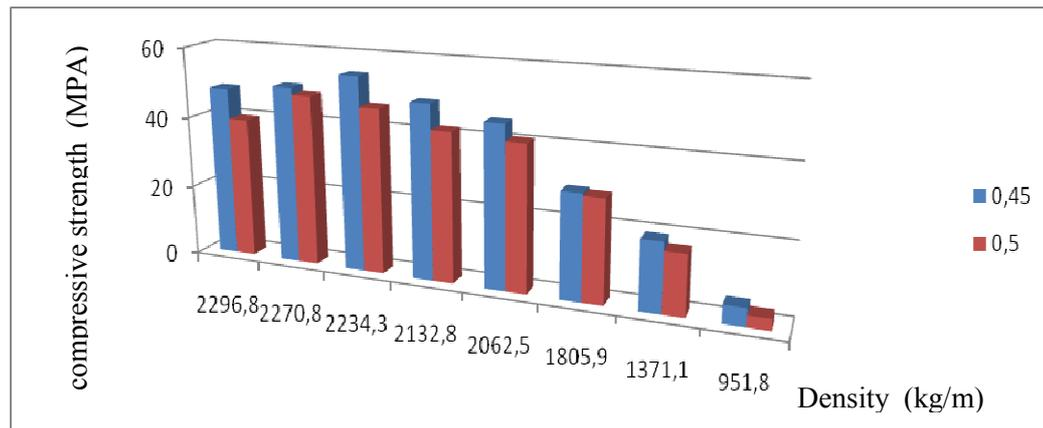
Fig. 6: Evolution of the compressive strength at 28days according to the density of the mixtures for E/C = 0.45&0.50
