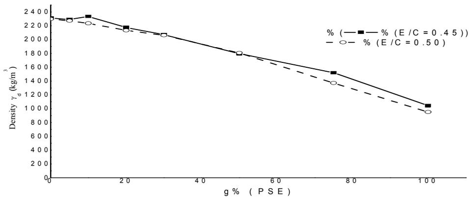
FIG. 1: Evolution of the density in the hardened state according to the content of polystyrene for  $E/C = 0.45$  &  $0.50$
