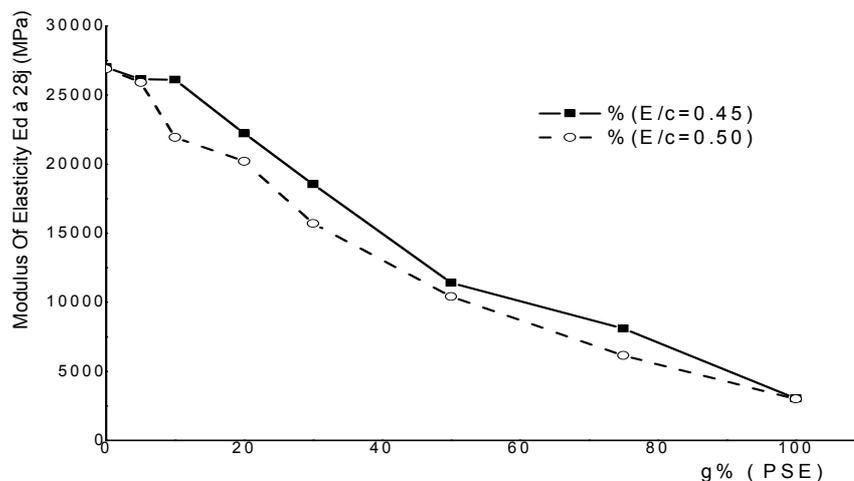
Fig. 5: Evolution of the dynamic modulus ED at 28 days according to the content of polystyrene for  $E/C = 0.45$  &  $0.50$
