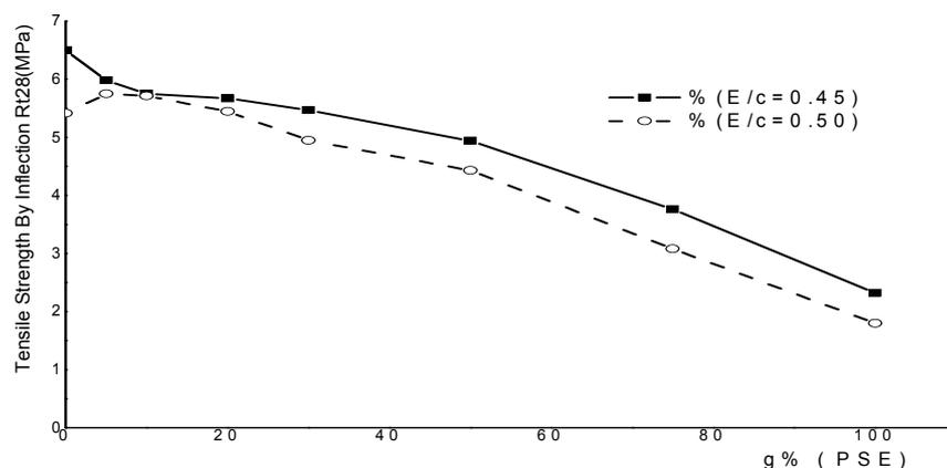
Fig. 4: Evolution of the tensile strength by inflection at 28 days according to the content of polystyrene for  $E/C = 0.45$  &  $0.5$
