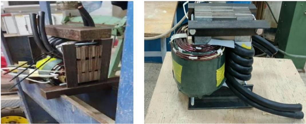
Figure 3.12 :construction de circuit secondaire
