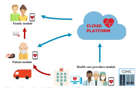
Figure 2.3. A Cloud-IoT based system for patient heart rate monitoring.
