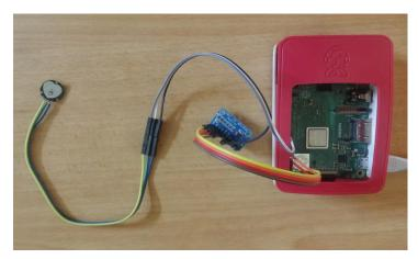
Figure 2.4. The heart rate measurement device of the proposed system.
