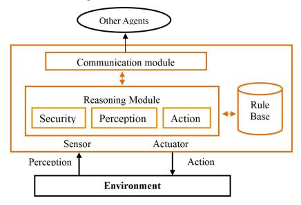
Figure 4.2. The architecture of device agent.
