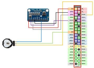
Figure 2.2. The wiring diagram of heart rate measurement device.
