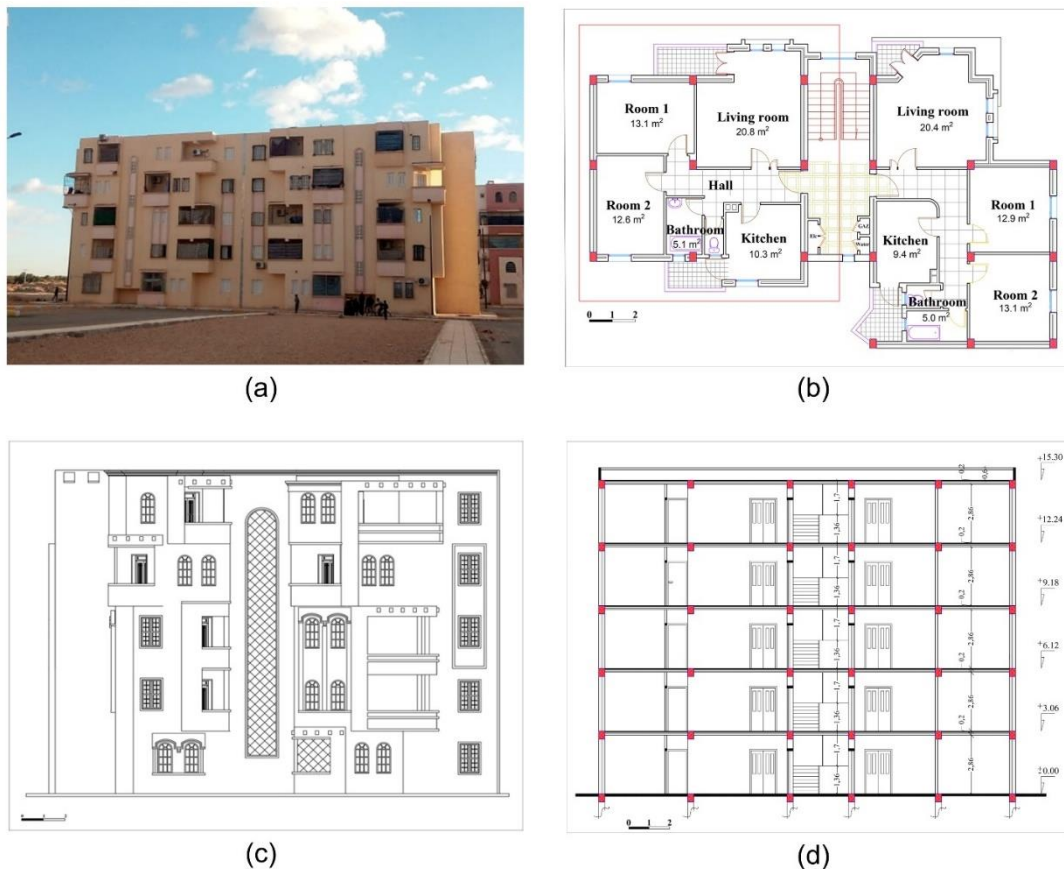
Figure II-5: Details of the selected multi-family social housing building typology; (a) real view of the building, (b) floor plan, (c) section, (d) front façade
