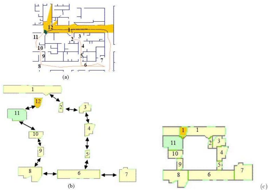
Figure III-14 : Problem of identification of the ASR;(b) it is difficult to detect that the ASR-12 and the ASR-1 account for the same space (c) ASRs-12 and 1 should logically be grouped together (Jefferies & Yeap 1998).
