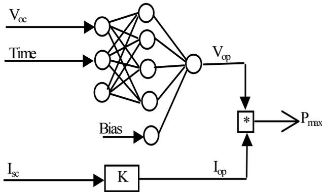
Figure 11 : Configuration of Neural Network
