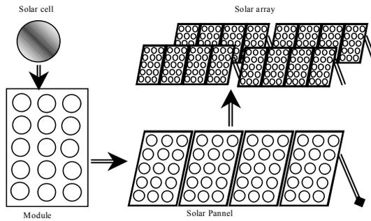
Figure 2 : PV generator hierarchy
