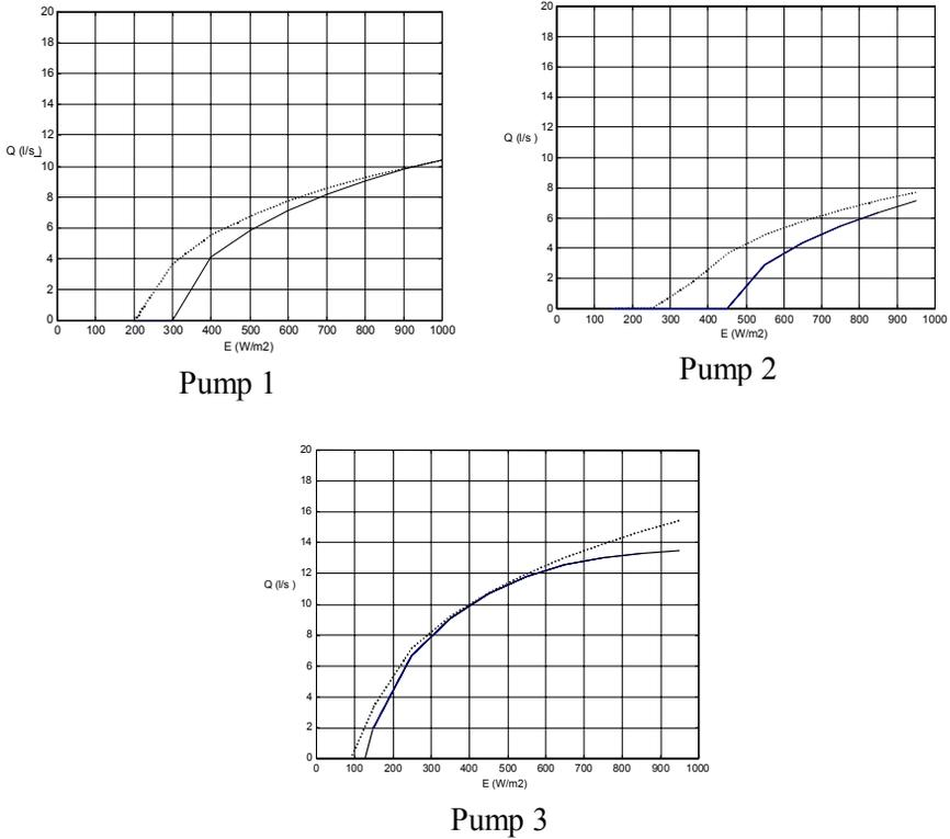
Figure 6: Pumps flow rate as a function of solar insolation
