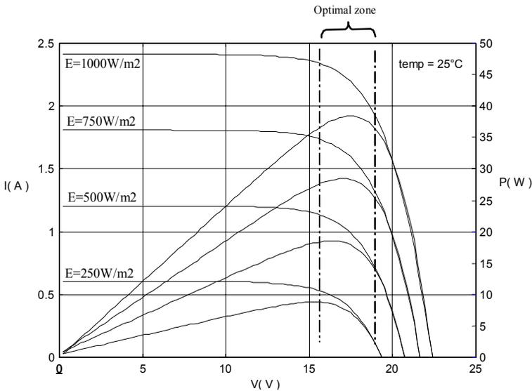
Figure 3 : Photovoltaic module characteristics
