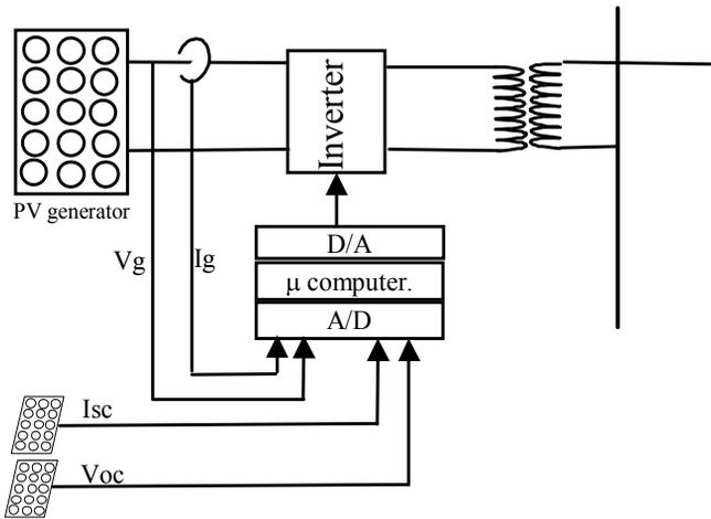
Figure 10 : Grid connected PV system
