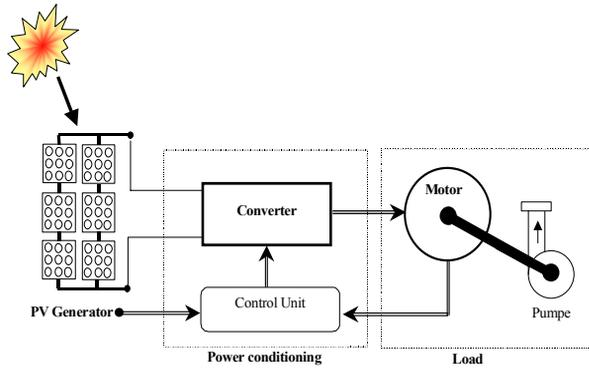
Figure1: Schematics of a photovoltaic pumping system
