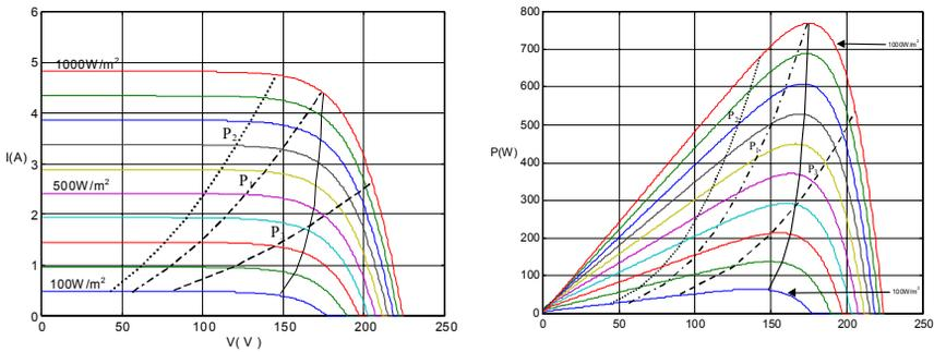
Figure 5: I-V and P-V characteristics of a PV pumping system, T=25°C
