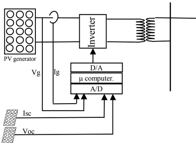
Figure 10 : Grid connected PV system
