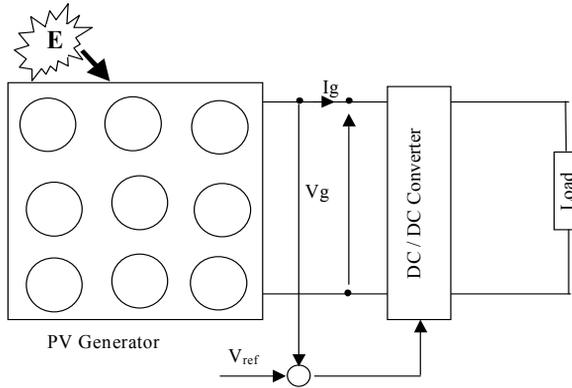
Figure 7 : MPPT without temperature compensation
