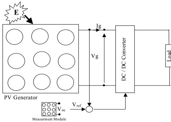
Figure 8 : MPPT with temperature compensation
