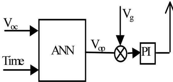
Figure 12 : Block diagram for optimal voltage identification
