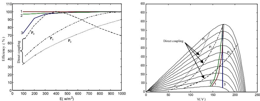
Figure 9 : System power efficiency as a function of solar insolation
