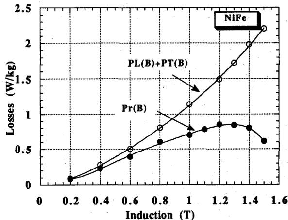
Figure 3 : Magnetic losses of the NiFe sheet obtained in circular and in sinusoidal induction (rolling and transverse directions)
