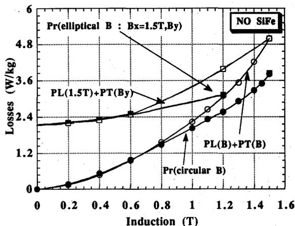
Figure 2 : Magnetic losses measured in different excitations for the NO SiFe sample
