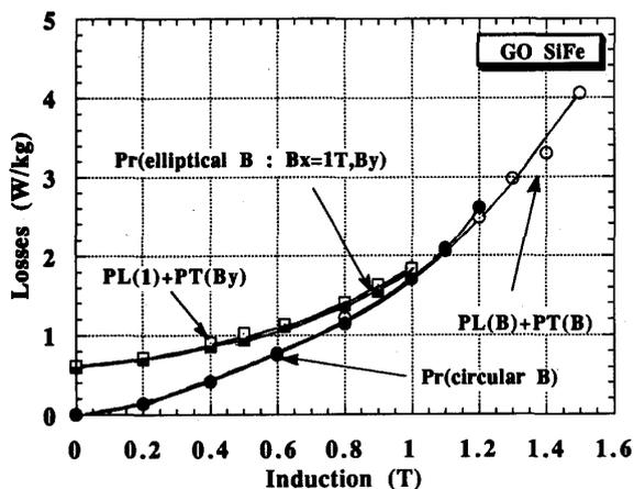
Figure 1 : Magnetic losses in alternating, circular and elliptical ( $B_x=1.0$  T,  $B_y$ ) conditions obtained for the GO SiFe sample
