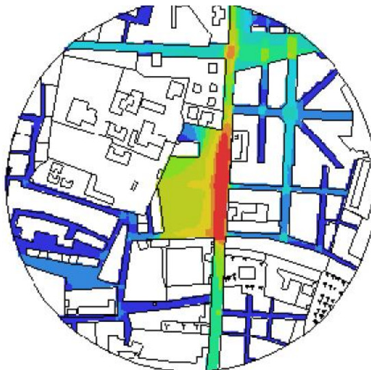
Figure VI.39: Connectivity within a 250 meter-radius perimeter
