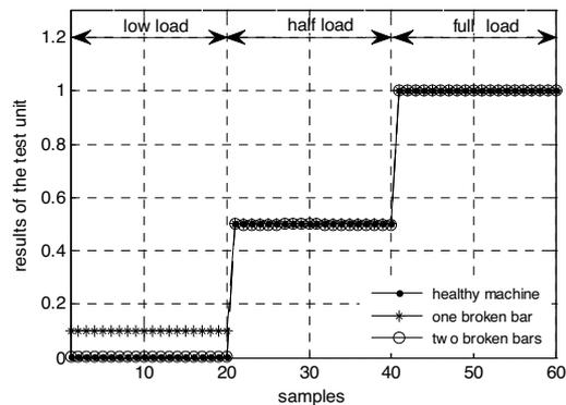
Fig. 11. Results of the test set. M1
