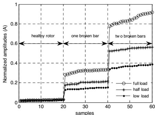
Fig. 9. Normalized amplitudes of the  $f_{bb}$  harmonics for : healthy rotor, one and two broken bars. Second classification, ascending order
