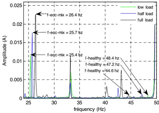
Fig. 2. Superposition of three stator currents spectra; healthy rotor: mixed-eccentricity harmonics and rotor asymmetry harmonics.
