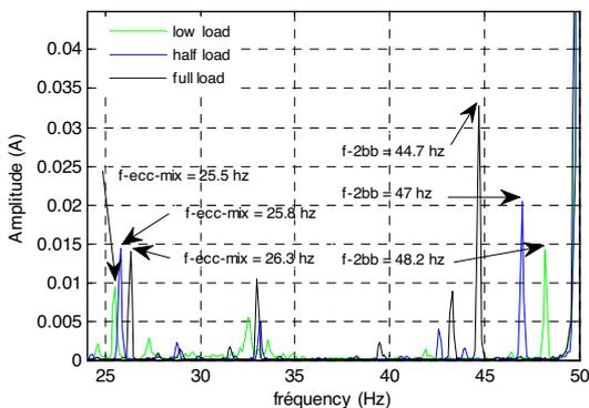
Fig.4. Superposition of three stator currents spectra; 2bb rotor: mixed-eccentricity harmonics and rotor asymmetry harmonics
