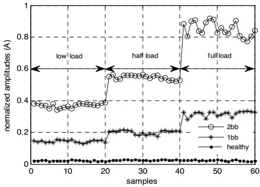
Fig. 5. Normalized amplitudes of the  $f_{bb}$  harmonics for: healthy rotor, one and two broken bars. First classification.
