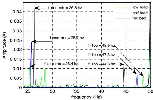
Fig. 3. Superposition of three stator currents spectra; 1bb rotor: mixed-eccentricity harmonics and rotor asymmetry harmonics.
