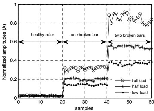
Fig. 6. Normalized amplitudes of the  $f_{bb}$  harmonics for the three rotors: healthy, one and two broken bars. Second classification.
