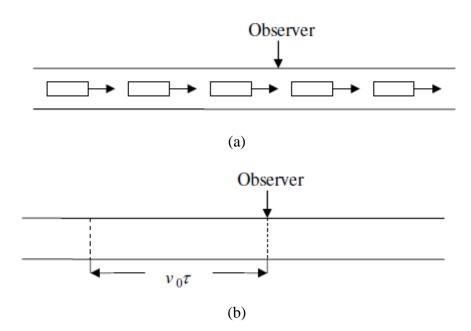
Figure 5. 2 (a) Constant flow of pedestrians, (b) Distance traveled in  $\tau$  hours for a single pedestrian.
