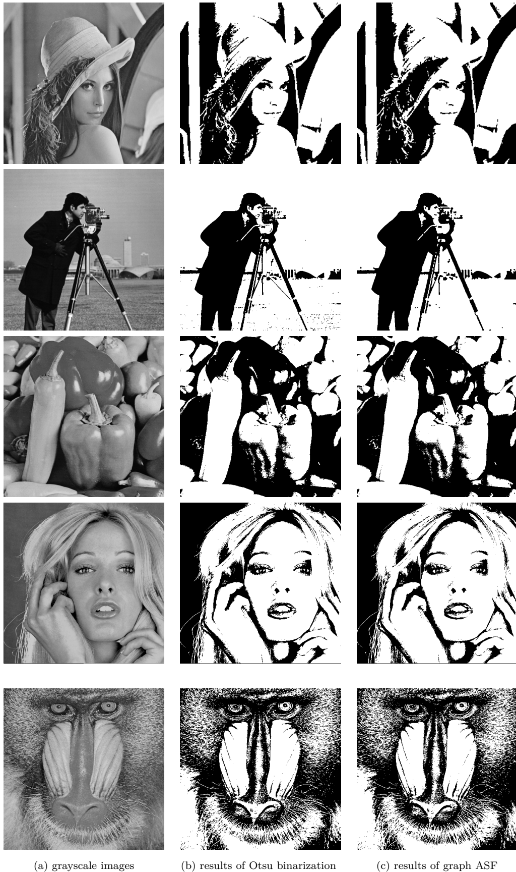
Figure 5.4: Illustration of Otsu binarization followed by mathematical morphology filtering on graphs from two images of the Standard image dataset.
