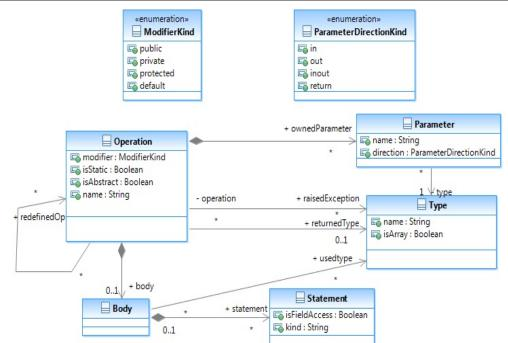
Figure 5.2 : The Operation Meta-model
