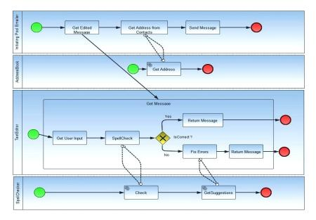
Figure 7.8: Recovered BPMN Architecture from the Emailer application
