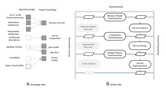
Figure 3.2 : An example of two-view approach representation. (A) Knowledge view and (B) activity view [Razavian et Lago, 2015]
