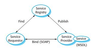
Figure 2.3 : Service Oriented Architecture [Sommerville, 2011]
