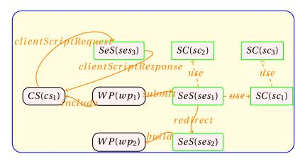
Figure 4.1 : Structure of a Web application
