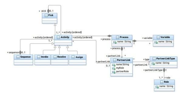
Figure 2.6 : An excerpt of the BPEL meta-model
