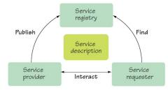
Figure 7.7: The service-oriented interaction pattern [Hall et al., 2011]
