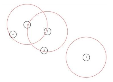
FIGURE 3.2: Networks where nodes face hidden and exposed nodes problem.
