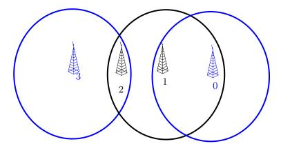
FIGURE 2.2: Illustration of exposed node problem.
