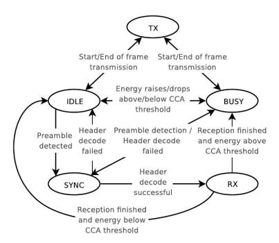
FIGURE 4.2: The state machine of the physical layer emulator distinguishes between Tx, Idle, Busy, Sync and Rx states [10].
