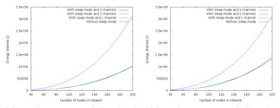
(A) Drained energy in a network of a grid topology of 3 cases of the number of channels.
