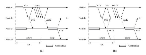
FIGURE 2.8: Data exchange in T-MAC, showing the early sleeping problem in (a) and the future-request-to-send technique in (b) [6].
