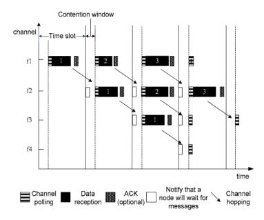
FIGURE 2.11: A light weight-channel hopping mechanism [8].
