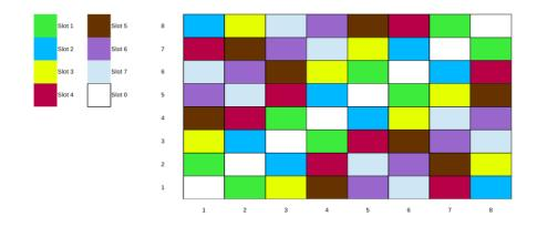
FIGURE 3.3: Time Slots Distribution based on Latin Square.
