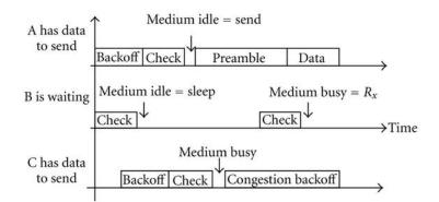
FIGURE 2.4: B-MAC communication example. All nodes are within range of each other. [3].
