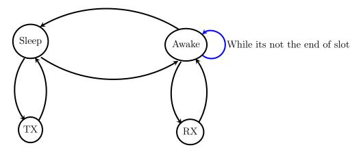
FIGURE 4.3: Abstract states of Phy layer that distinguishes between Sleep, Awake, RX and TX states after the installation of SlotChannelMannager layer.
