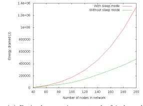
(C) Drained energy in a network of 1 channel in a random topology (10 nodes in 500m2).
