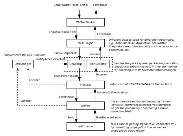
FIGURE 4.1: WifiNetDevice architecture [9].
