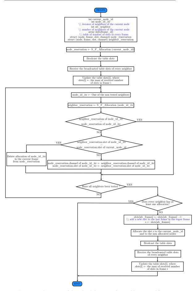
FIGURE 3.7: Reservation of channel and slot process (executed by every node).
