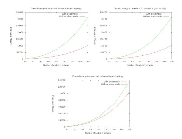
FIGURE 4.9: Drained energy in a network of grid topology.
