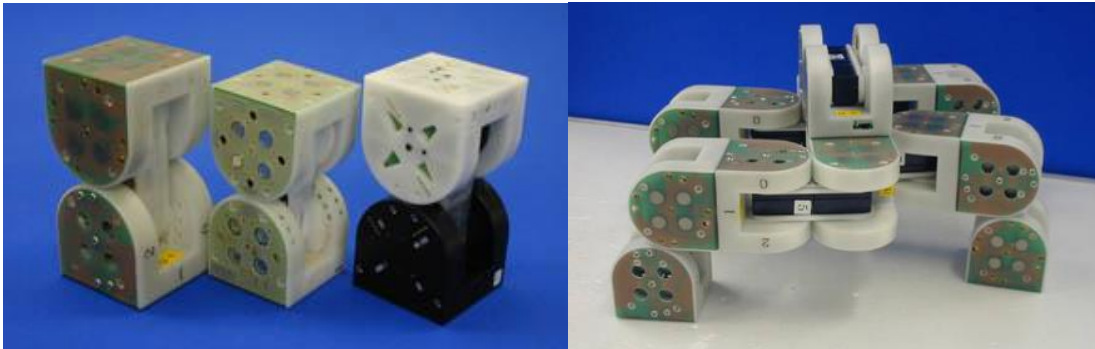
Figure 2.3. Robots modulaire M-TRAN. [YOS03]
