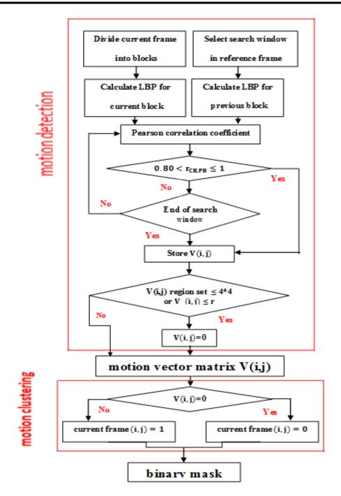
Figure 5.4: Flow-chart of the proposed object segmentation method
