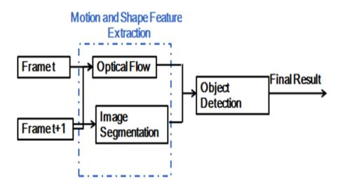
Figure 5.1: Block-diagram of the proposed moving object detection method
