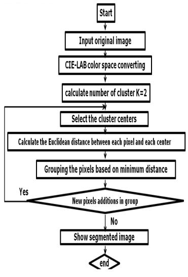
Figure 5.2: Flow-chart of K-means clustering algorithm
