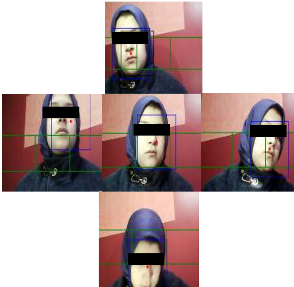
Figure 3.11 : Head gesture recognition results in a bright light condition.
