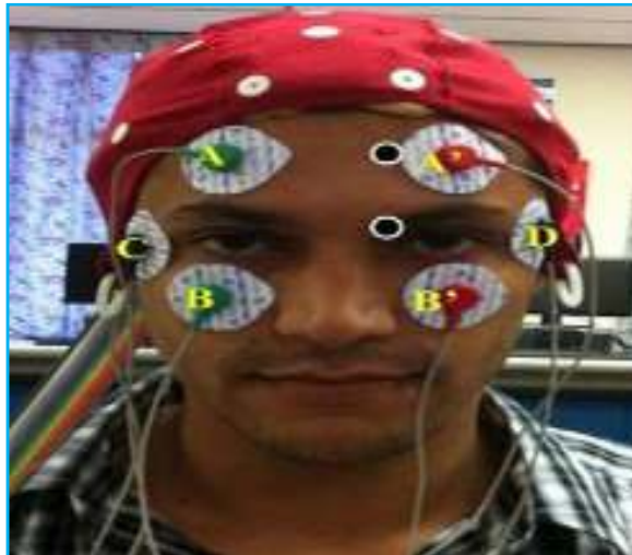
Figure 1.17: Placement of electrodes for EOG measurement.
