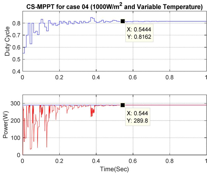
**Fig.III.23.** Duty cycle and PV power responses using PSO based MPPT technique Under case 04 (constant irradiation  $1000\text{W}/\text{m}^2$  with variable temperature)
