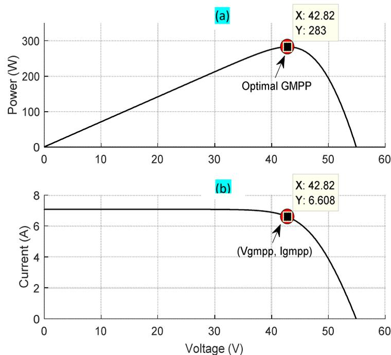
**Fig.III.14.** Characteristics curves of PV array 3S2P under case 03 ( $1000\text{W/m}^2$  and  $55^\circ\text{C}$ )
