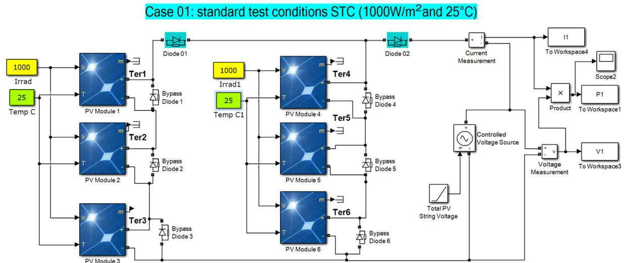
**Fig.III.2.** Simulink model of the tested PV array configuration (3S2P) for case 01 (STC)
