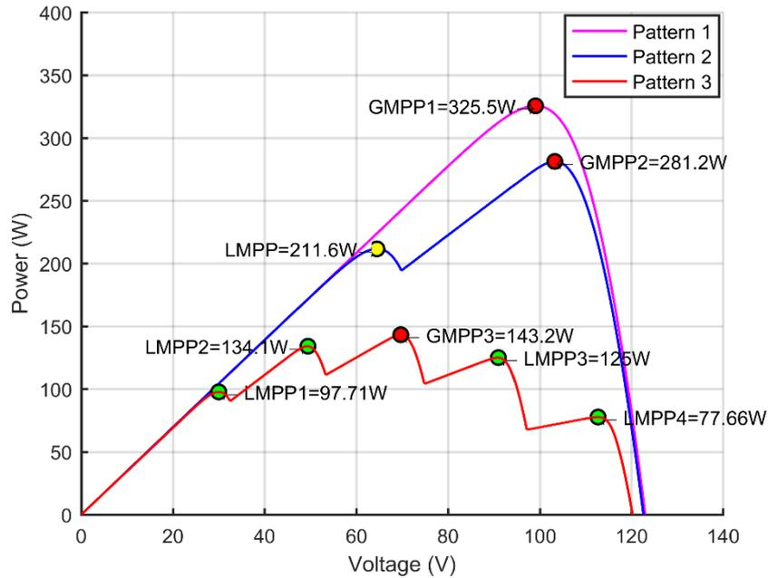
**Fig.IV.3.** Curve of power-voltage (P-V) characteristics for different partial shading cases
