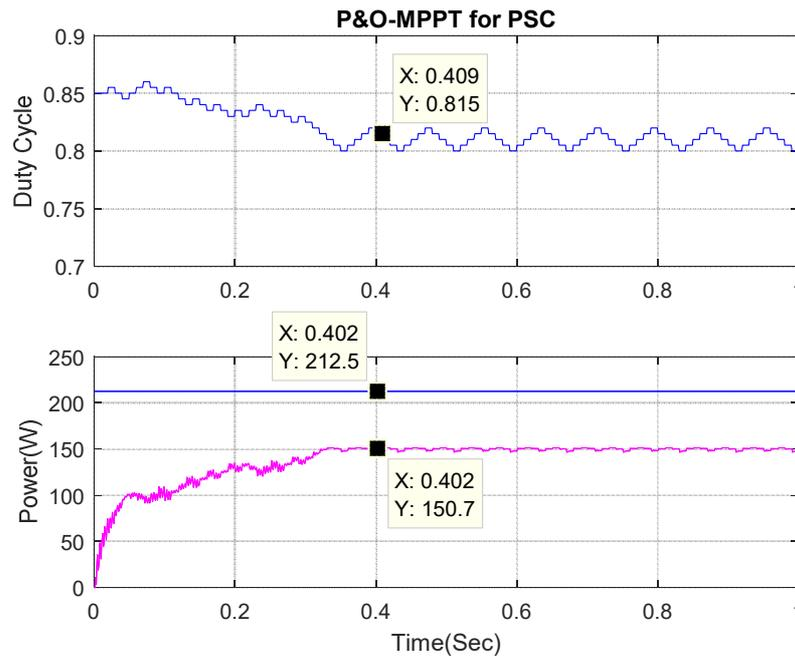
Fig.III.10. Duty cycle and PV power responses using P&O based MPPT technique for case 02 (PSC)
