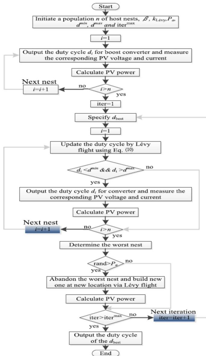
Fig. I.10. Flowchart of Cuckoo Search (CS) based MPPT method [61].
