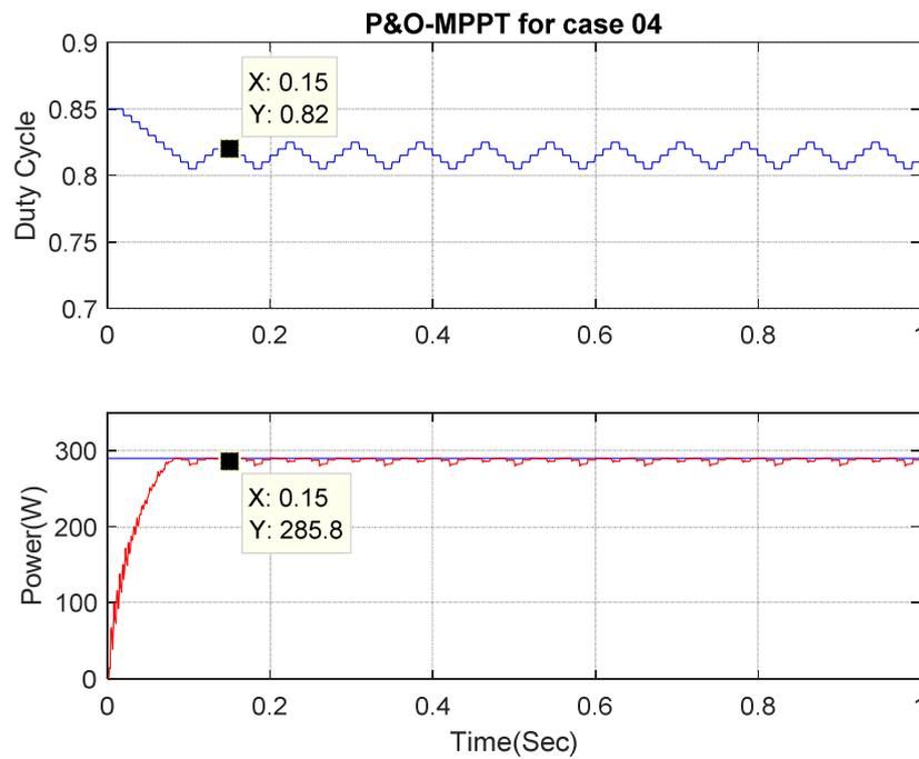
**Fig.III.21.** Duty cycle and PV power responses using P&O based MPPT technique Under case 04 (constant irradiation at  $1000\text{W}/\text{m}^2$  and variable temperature)
