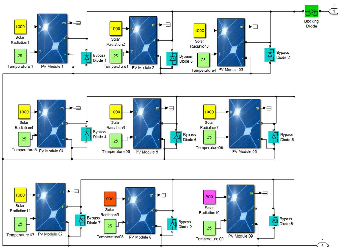
Fig. II.17. Simulink model of the PV configuration parallel (9P) under PSC
