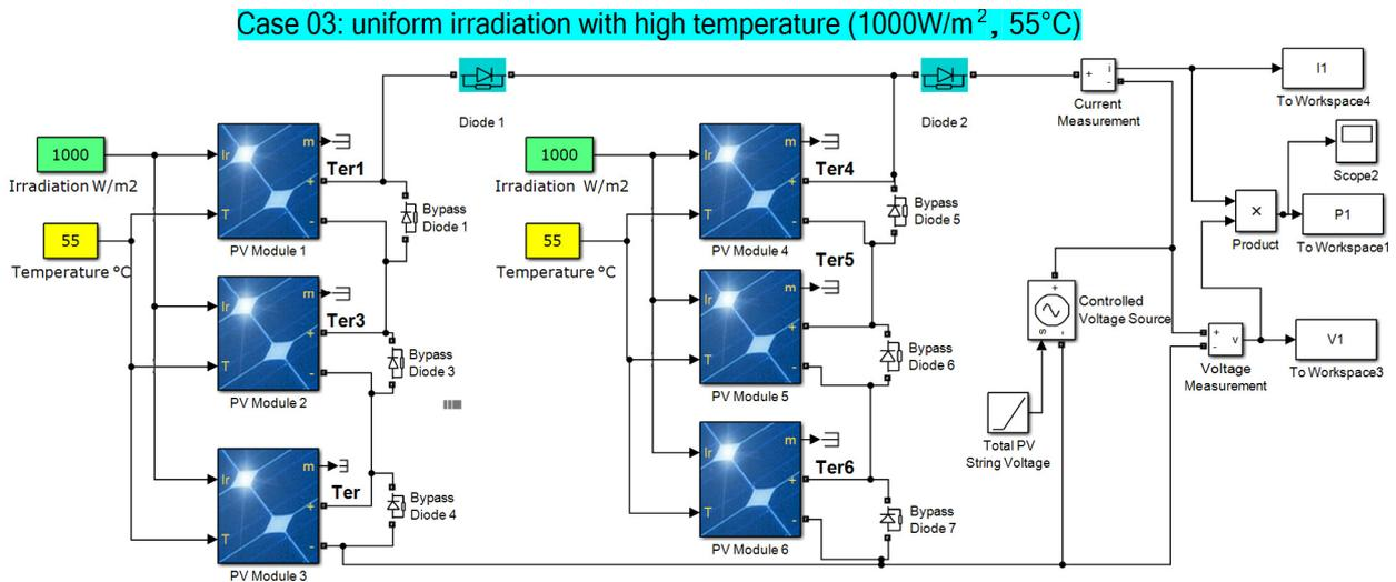
**Fig.III.13.** Simulink model of the tested PV array 3S2P under case 03 ( $1000\text{W/m}^2$  and  $55^\circ\text{C}$ )
