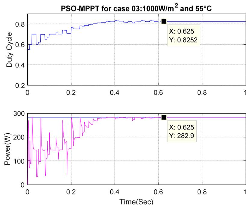
**Fig.III.16.** Duty cycle and PV power responses using PSO based MPPT technique for case 03 ( $1000\text{W}/\text{m}^2$ ,  $55^\circ\text{C}$ )
