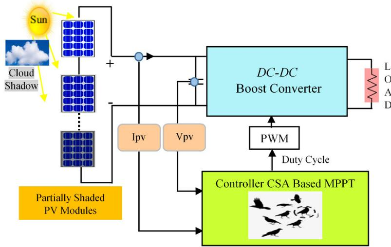
Fig. IV.7. General diagram of the partially shaded PV system with proposed CSA based MPPT controller
