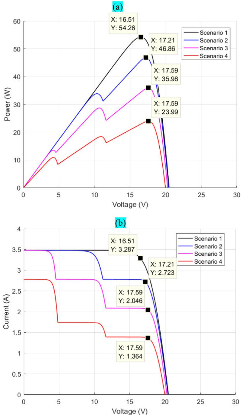
**Fig. II.13.** Curves of electrical characteristics for partially shaded solar cells in PV module
