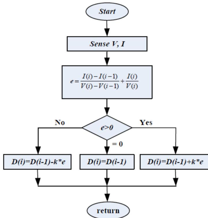
Fig. I.6. Flowchart for Incremental conductance algorithm based MPPT [48].
