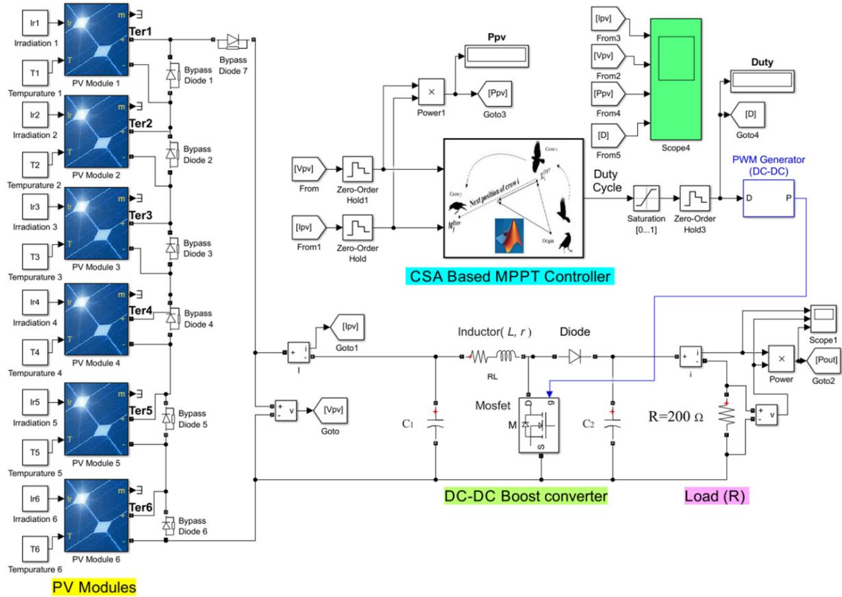
**Fig. IV.10.** Simulation model of the used PV system with CSA based MPPT controller
