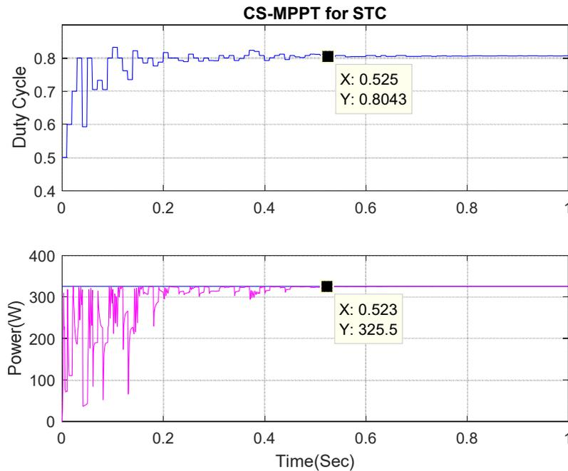
Fig.III.9. Duty cycle and PV power responses using CS based MPPT technique for STC case
