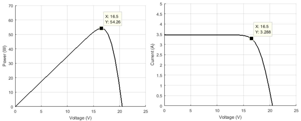
Fig. II.10. Simulated characteristics of PV module (SM55W) under standard test conditions STC
