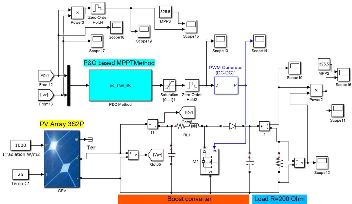
Fig.III.6. Simulink model of standalone PV system with P&O Based MPPT controller under STC
