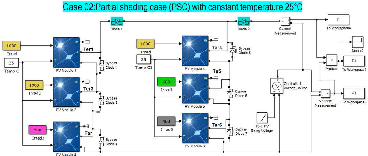
Fig. III.10. Simulink model of the tested PV array 3S2P under case 02 partial shading case (PSC)
