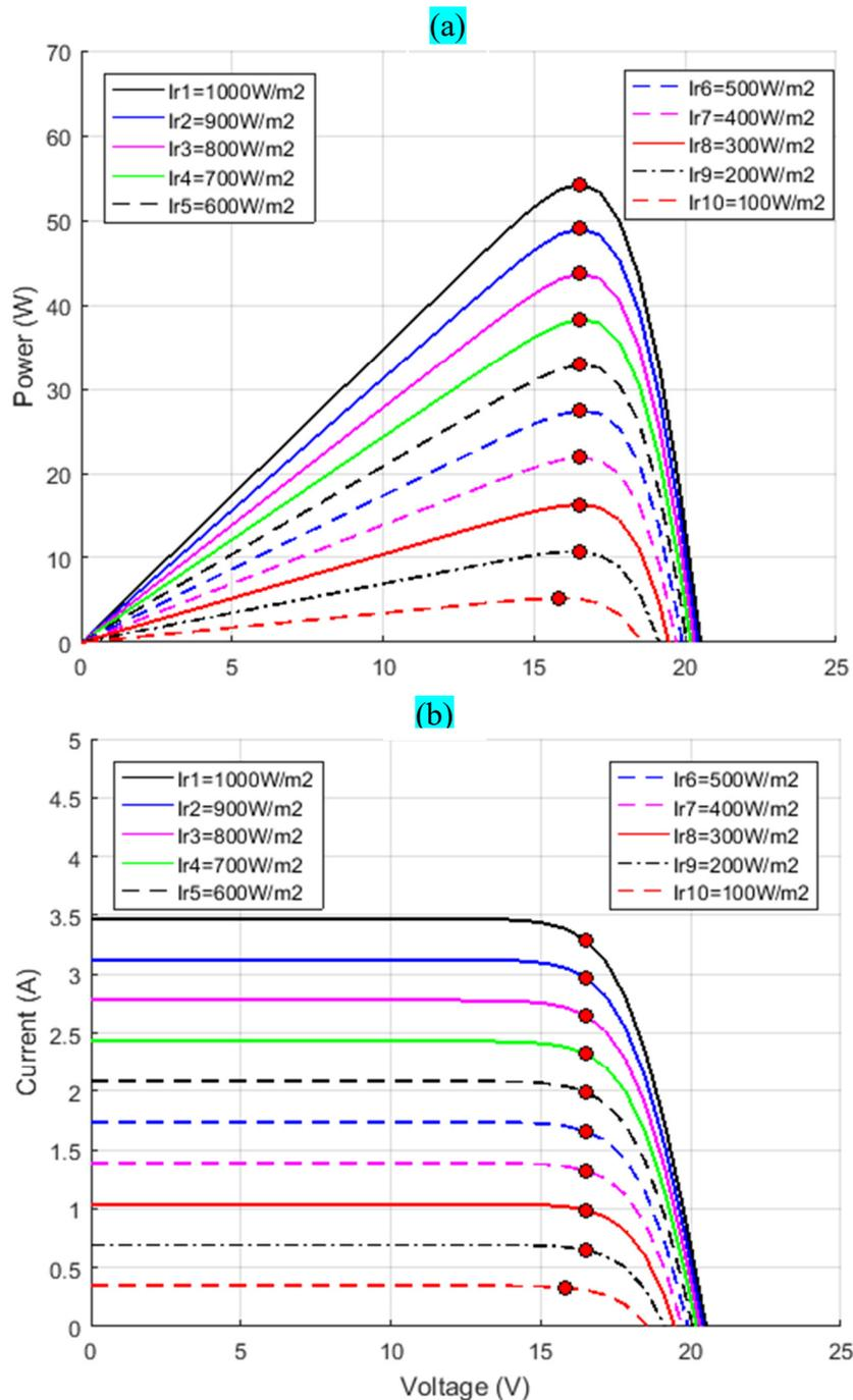
**Fig. II.11.** Output characteristics of PV module (SM55W) under different irradiation levels
