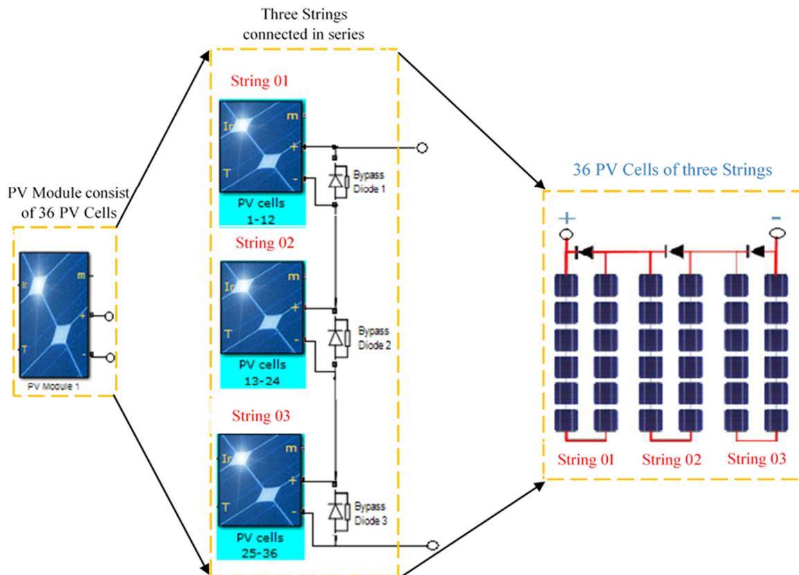
Fig. II.8. Illustrative schema for the interconnection of solar cells inside the used PV module
