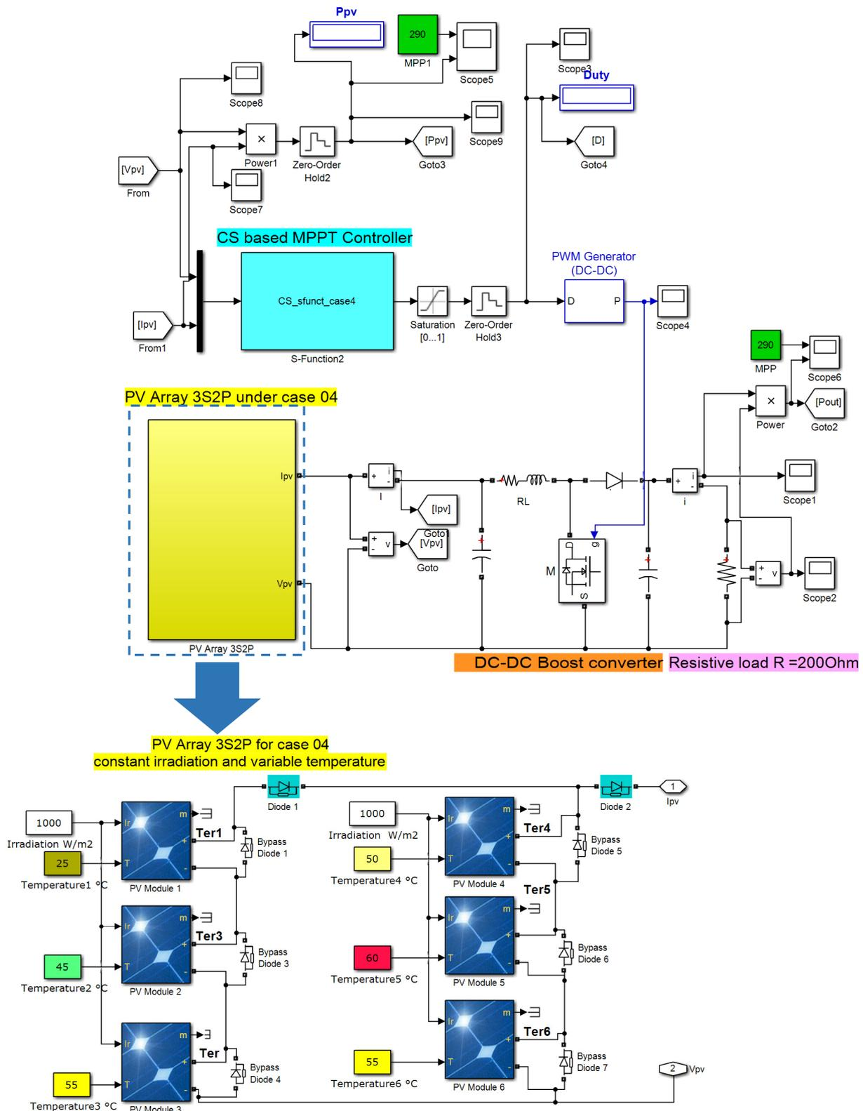
Fig.III.20. Simulink model of PV system with 3S2P configuration and CS-MPPT controller under Conditions of case 04 (Constant irradiation with variable temperature)
