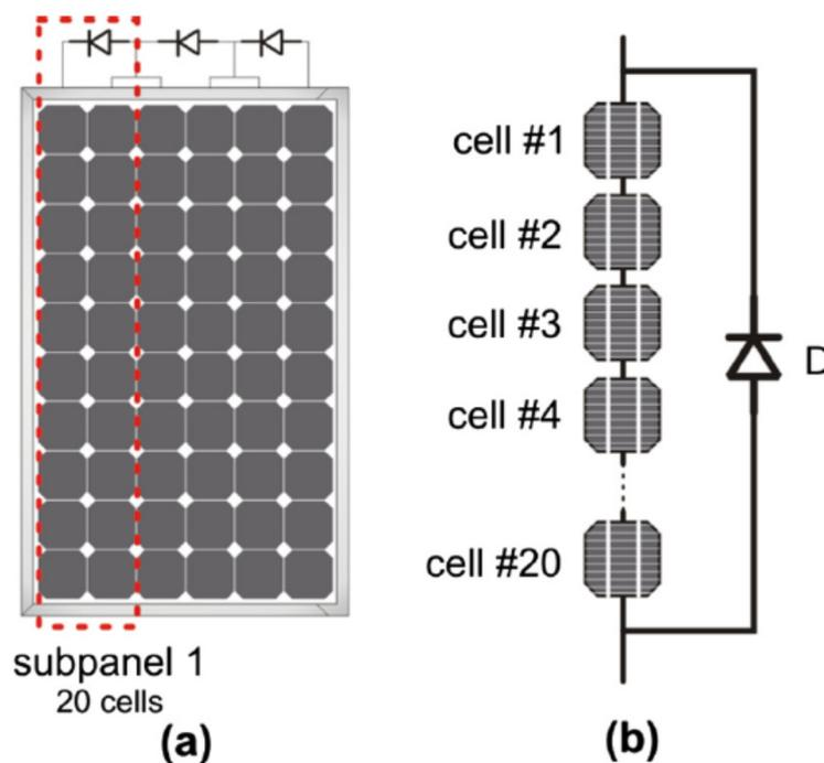
**Fig. II.3.** Role of diodes in PV panel (a) Sketch of a solar panel partitioned into 3x20-cell subpanels, (b) simplified representation of an individual subpanel
