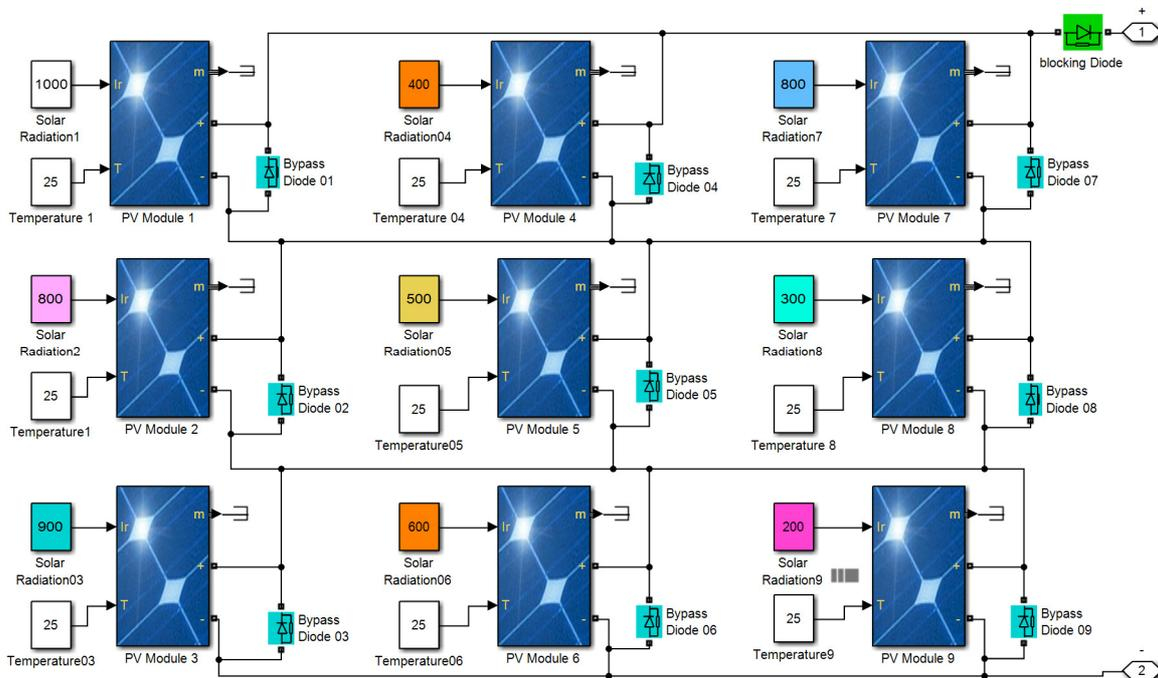
Fig. II.21. Simulink model of partially shaded PV configuration TCT for scenario 4
