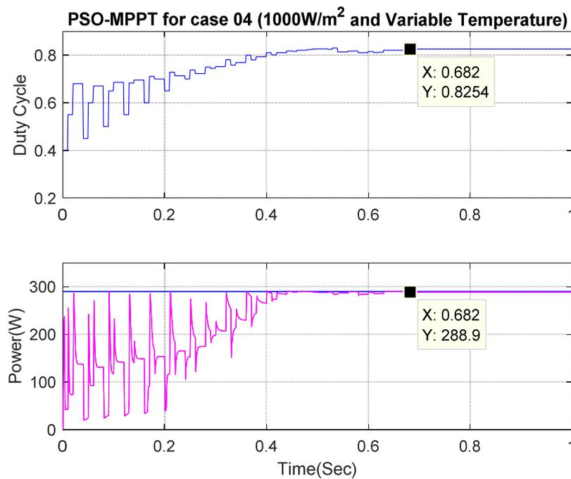
**Fig.III.22.** Duty cycle and PV power responses using PSO based MPPT technique Under case 04 (constant irradiation  $1000\text{W}/\text{m}^2$  and variable temperature)
