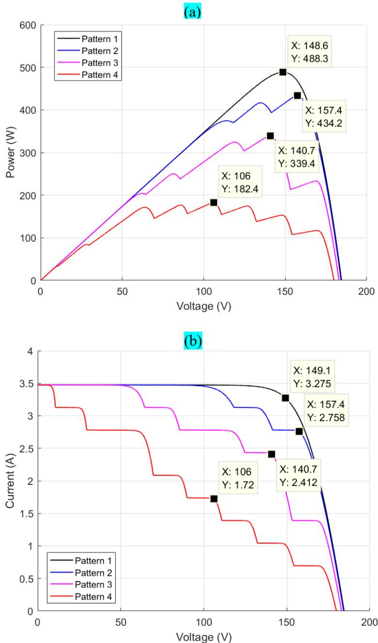
**Fig. II.16.** Curves of electrical characteristics for series PV configuration (9S) under the conditions of the four scenarios tested (a) P-V curve, (b) I-V curve
