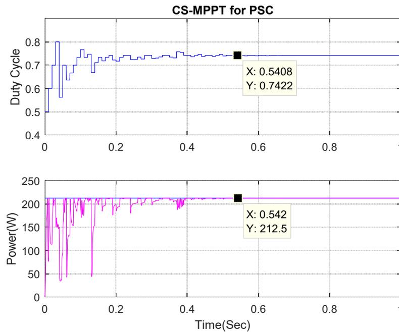
**Fig.III.12.** Duty cycle and PV power responses using CS based MPPT technique for case 02 (PSC)
