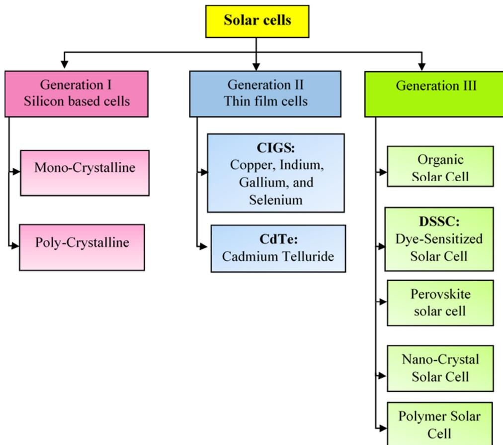
Fig.I.1 Classification of Solar Cells [6].
