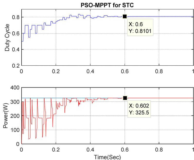
**Fig.III.8.** Duty cycle and PV power responses using PSO based MPPT technique for STC case
