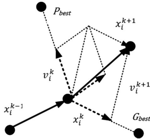
Fig. I.9. Particles movement in PSO
