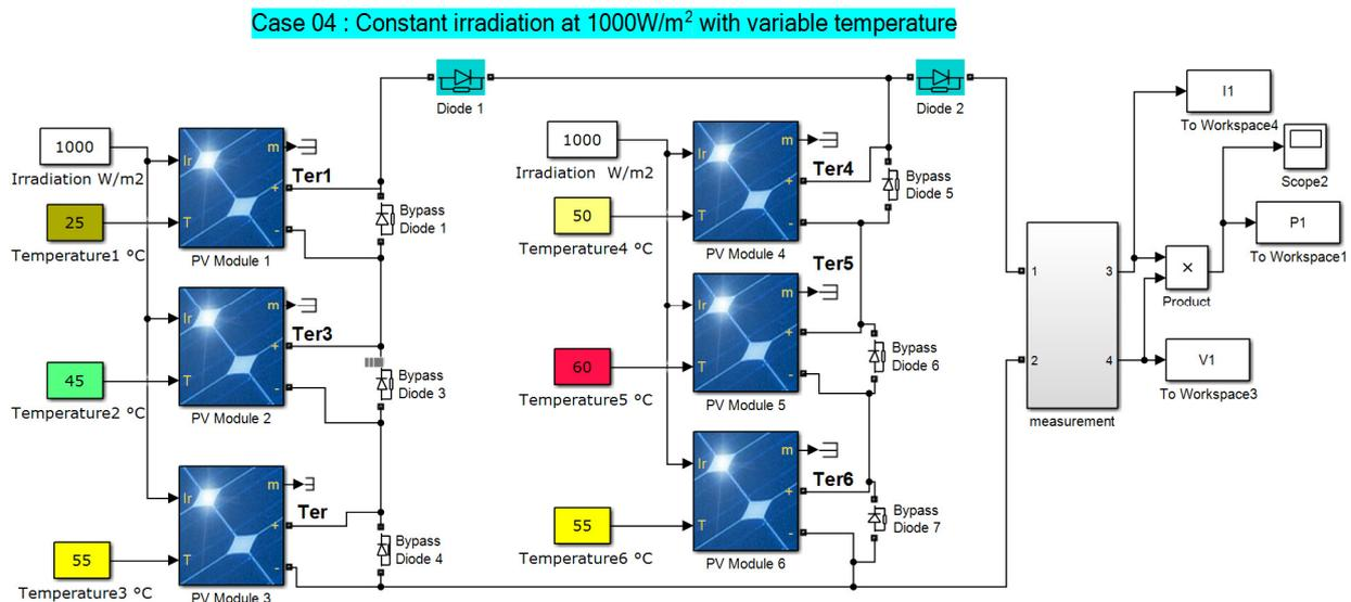
Fig.III.18. Simulink model of PV array configuration 3S2P for case 04 (1000W/m<sup>2</sup> with variable temperature)
