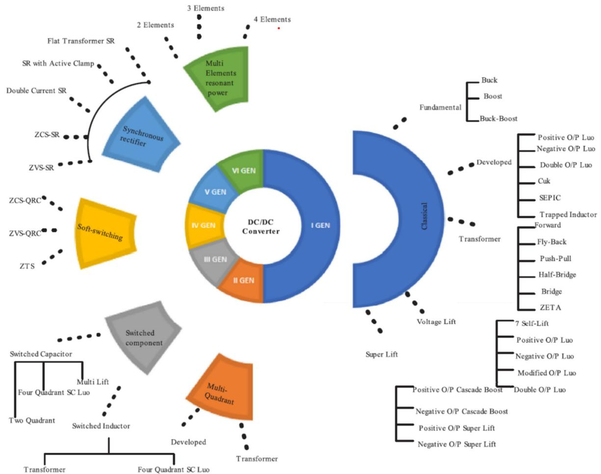
Fig. I.3. Classification of DC/DC converters [6].
