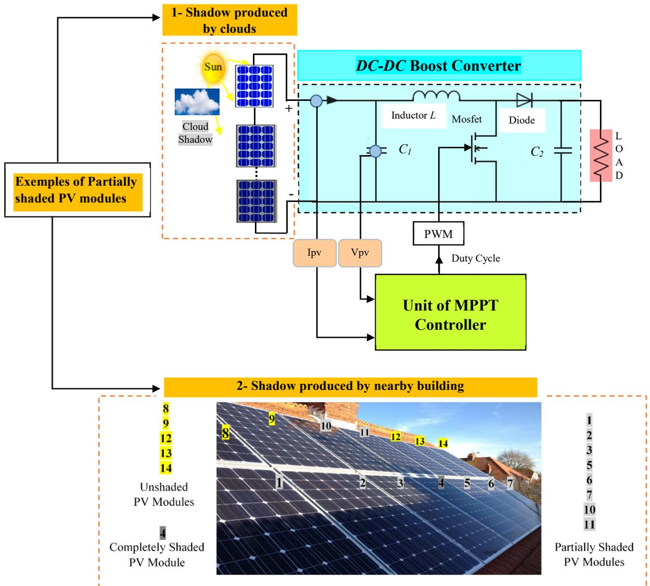
Fig. 1. General diagram of an autonomous PV system with a MPPT controller and examples of partial shade
