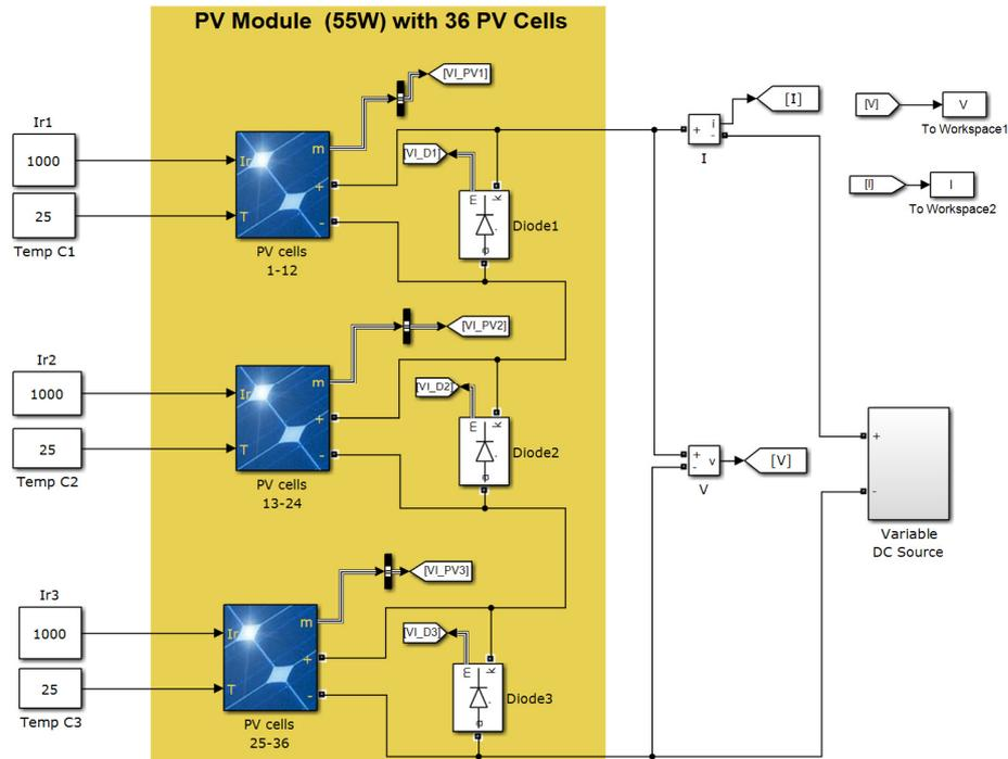
Fig. II.9. Simulated solar cells of PV module as three strings under standard test conditions STC
