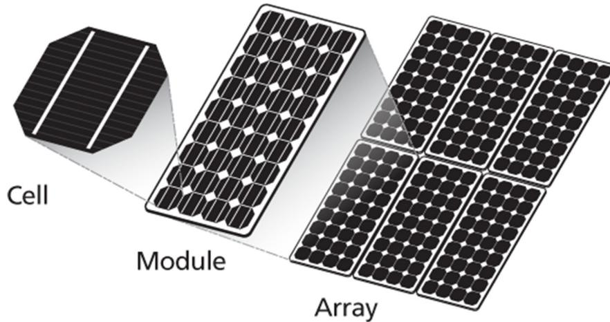
Fig. II.7. PV generator from cell to array
