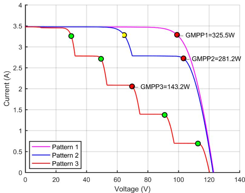
**Fig.IV.4.** Curve of current-voltage (I-V) characteristics for different partial shading cases
