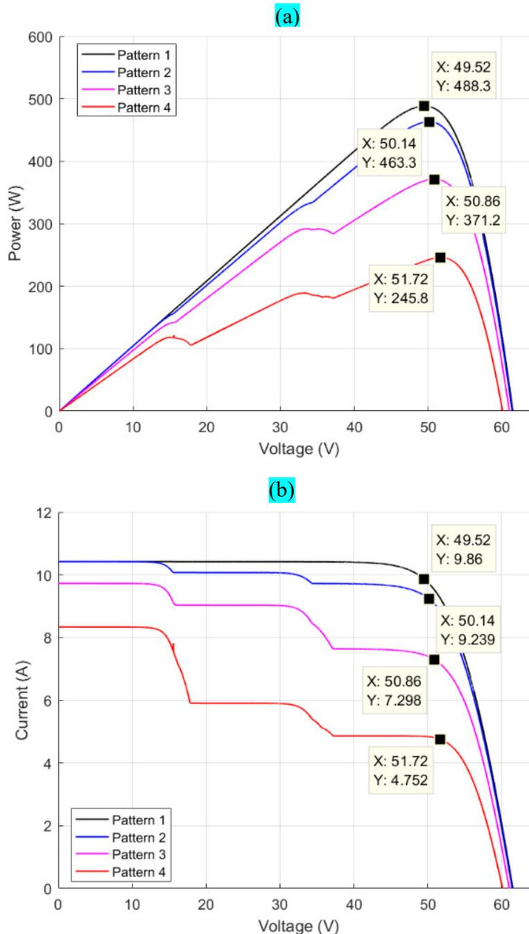
**Fig. II.20.** Simulated characteristics of PV array configuration (3S3P) under four used scenarios
