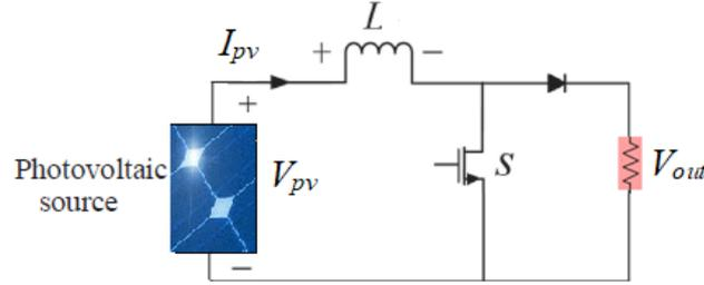
Fig. IV.5. Topology circuit of DC-DC boost converter
