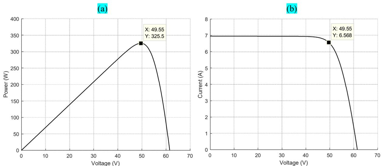
**Fig.III.3.** Characteristics curves of PV array 3S2P under standard test conditions STC
