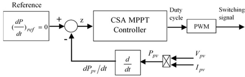
**Fig. IV.9.** Single loop control in PV system based CSA-MPPT controller
