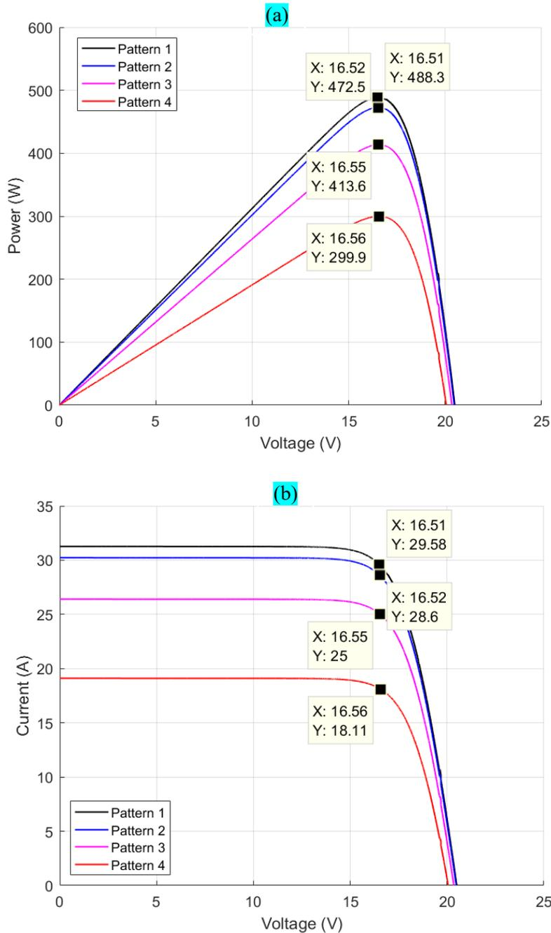
**Fig. II.18.** Curves of electrical characteristics of the PV configuration parallel (9P) under the conditions of the four scenarios tested (a) P-V curve, (b) I-V Curve
