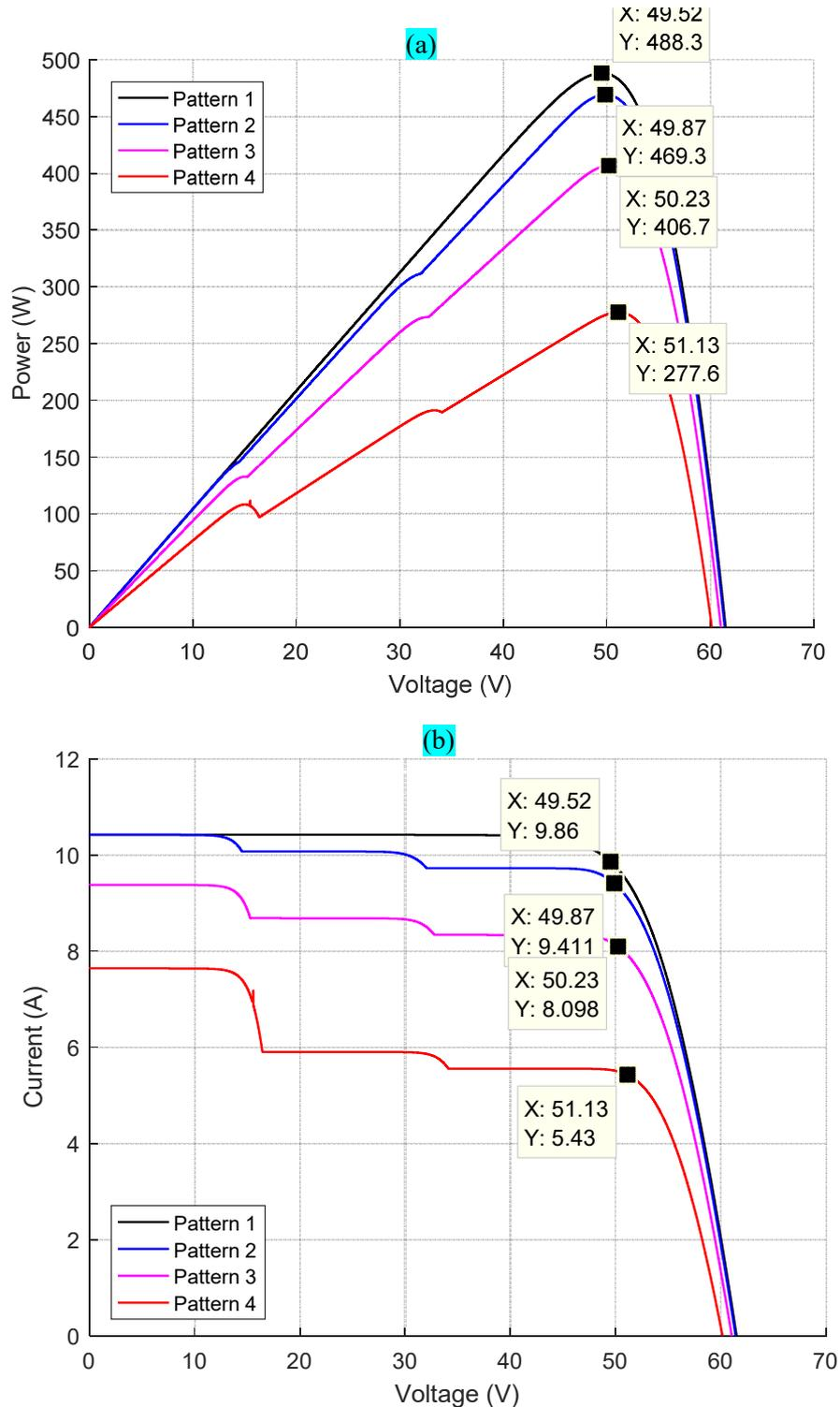
**Fig. II.22.** Simulated characteristics of PV configuration 3x3 TCT under four used scenarios
