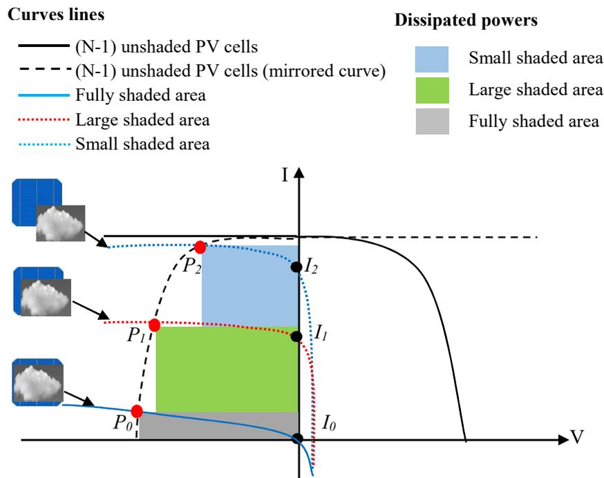
**Fig. II.6.** The dissipated power resulted by the shaded area in PV cells
