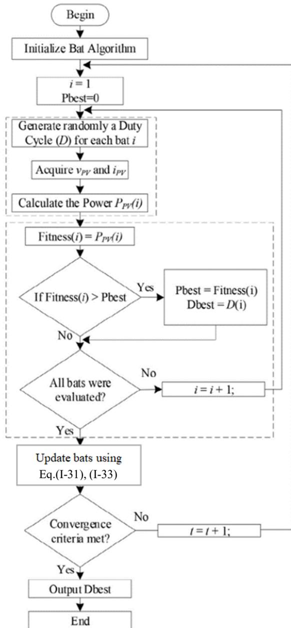
Fig. I.14. Bat Algorithm (BA) based MPPT [20]
