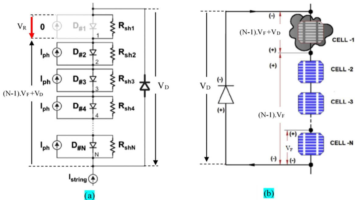
**Fig. II.4.** Shaded PV cells modeling (a) Equivalent circuit and (b) pictorial description of a subpanel comprising 20 cells. Cell 1 is assumed fully shaded.
