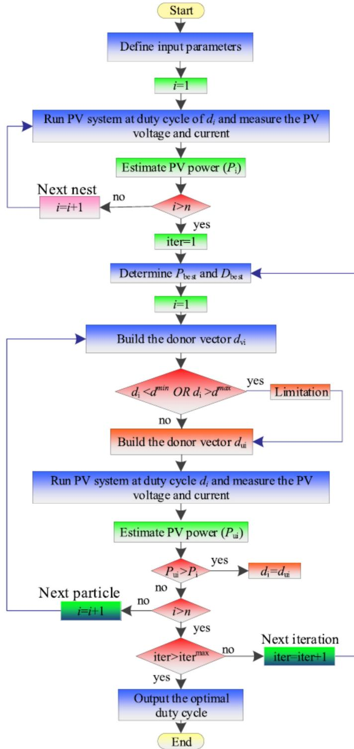
**Fig. I.8** The searching procedure of DE based MPPT algorithm [59].
