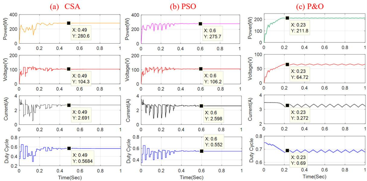
Fig.IV.12. Simulated system responses of CSA, PSO and P&O methods under case 2
