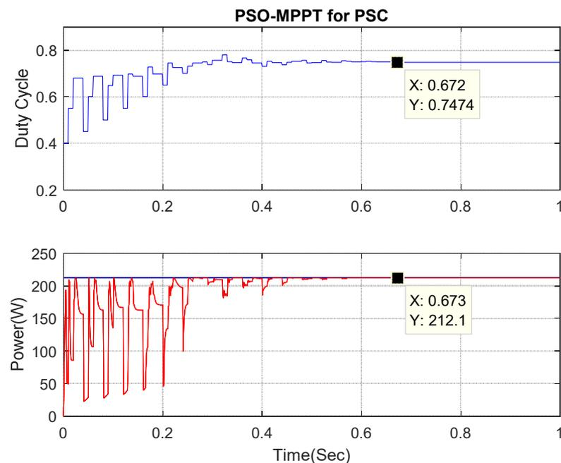
Fig.III.11. Duty cycle and PV power responses using PSO based MPPT technique for case 02 (PSC)
