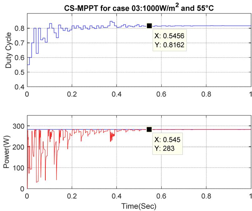
**Fig.III.17.** Duty cycle and PV power responses using CS based MPPT technique for case 03 (1000W/m<sup>2</sup> and 55°C)
