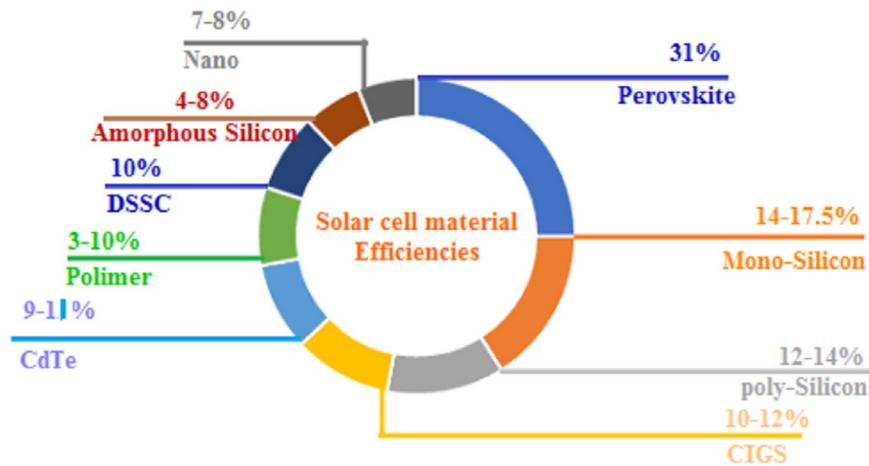
Fig.I.2. Efficiency of various PV materials [6].
