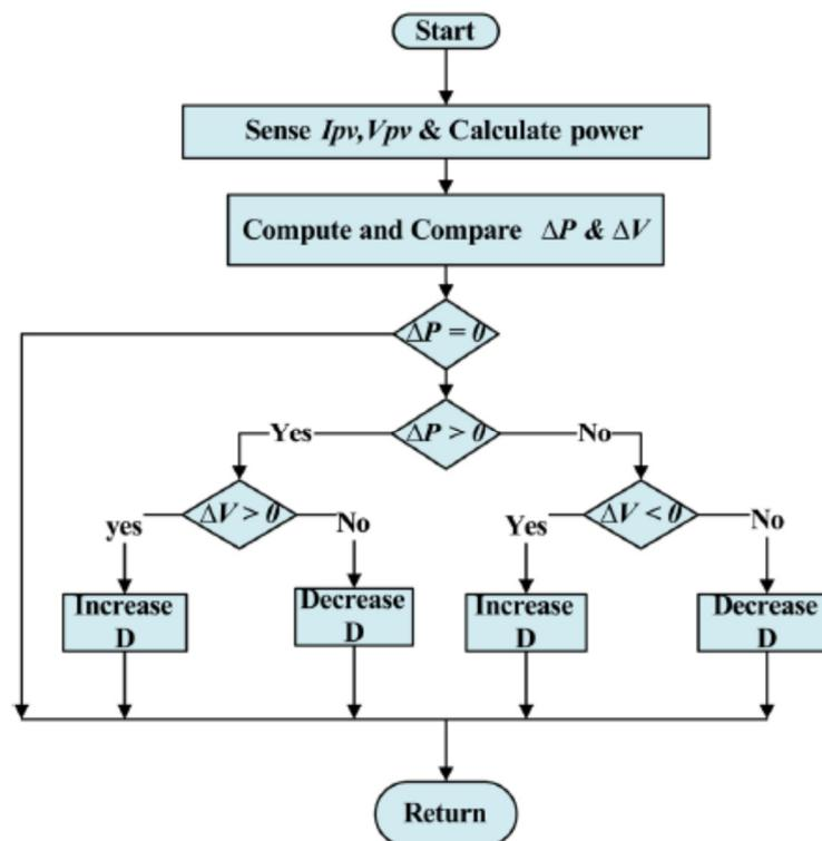
Fig. I.5. Flowchart of P&O based MPPT algorithm [50].
