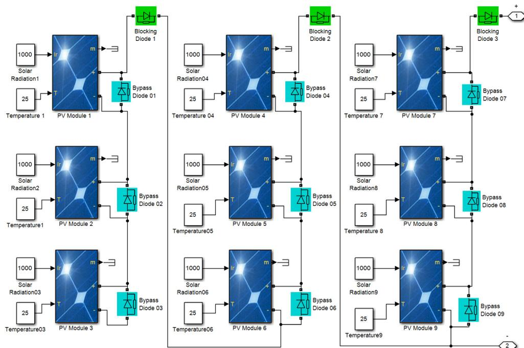
**Fig. II.15.** Simulink model of the PV configuration series (9S) under STC
