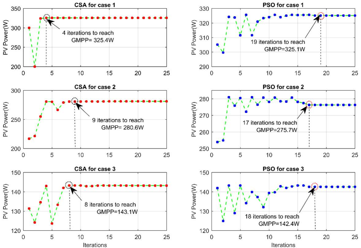
Fig. IV.14. The convergence process to GMPP versus iterations in CSA and PSO methods under three shading cases
