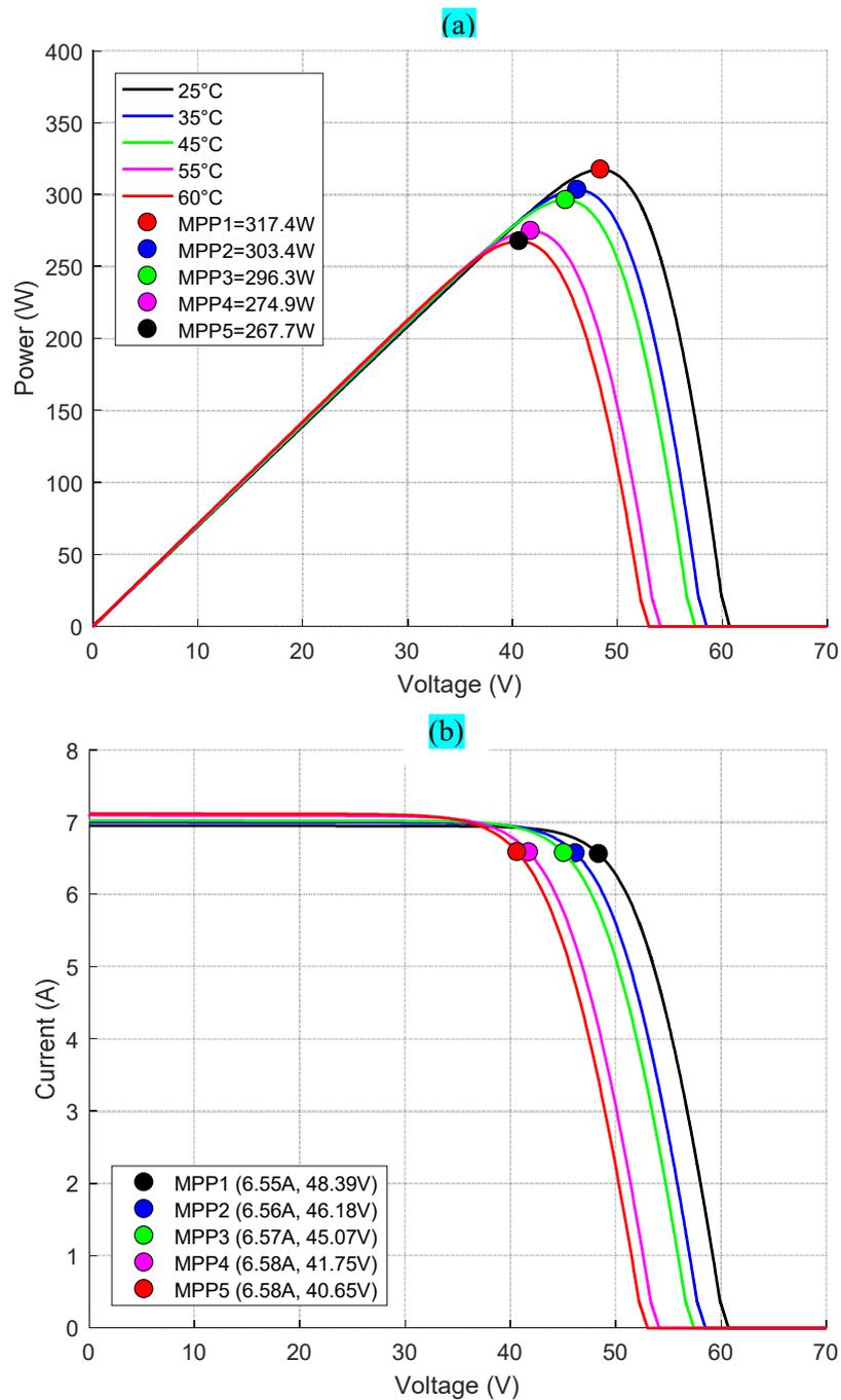
**Fig.III.5.** Curves of PV characteristics of PV array 3S2P under constant irradiation  $1000\text{W}/\text{m}^2$  and variable temperature (a) P-V curve, (b) I-V curve
