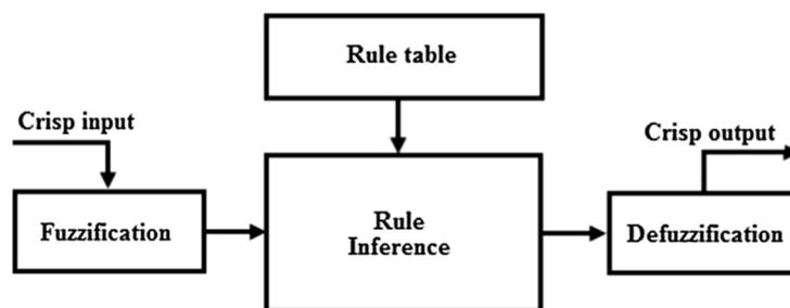
Fig. I.7. Basic fuzzy logic structure [53].
