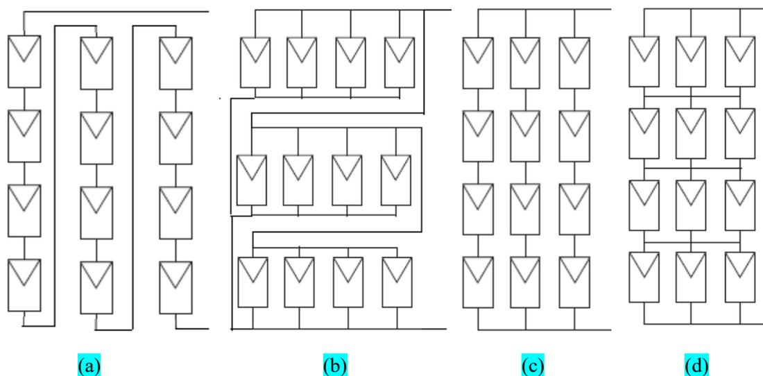
**Fig. II.14.** PV array configurations (a) series S, (b) parallel P, (c) Series-Parallel S-P (d) Total-Cross-Tied TCT
