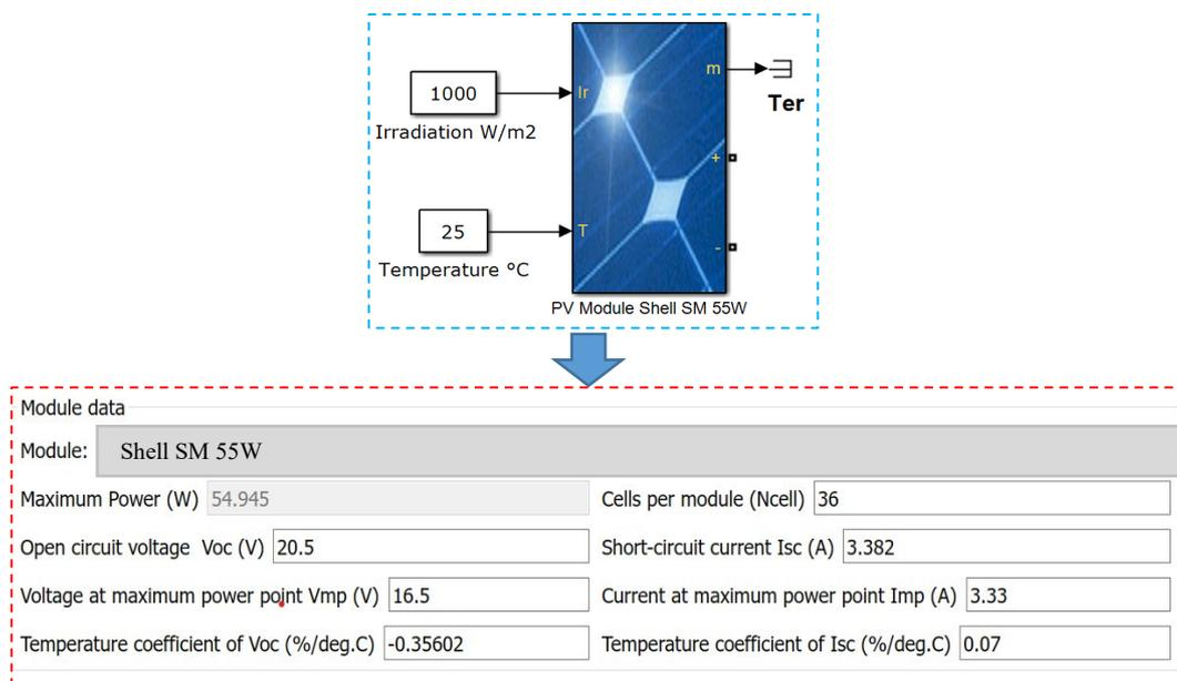
**Fig. III.1.** Electrical specifications data of the used PV module Shell SM 55W for STC conditions
