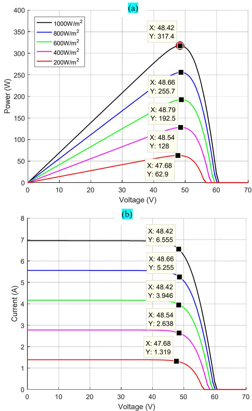
**Fig.III.4.** Characteristics curves of PV array 3S2P under different irradiation levels and constant temperature 25°C, (a) P-V curve, (b) I-V curve
