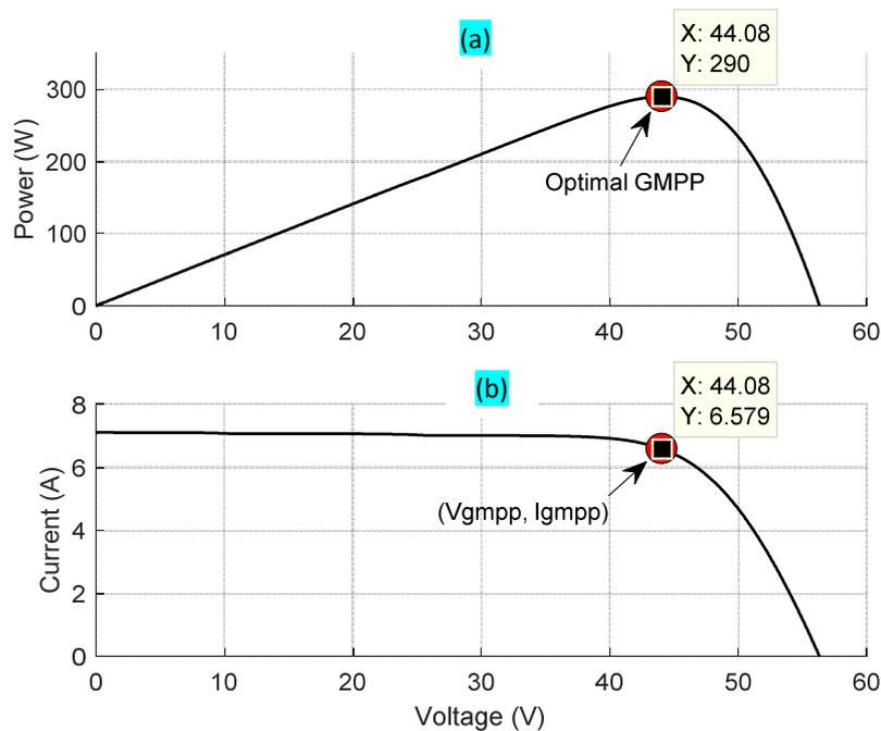
Fig.III.19. Characteristics curves of PV array 3S2P for case 04 (1000W/m<sup>2</sup> and variable temperature)
