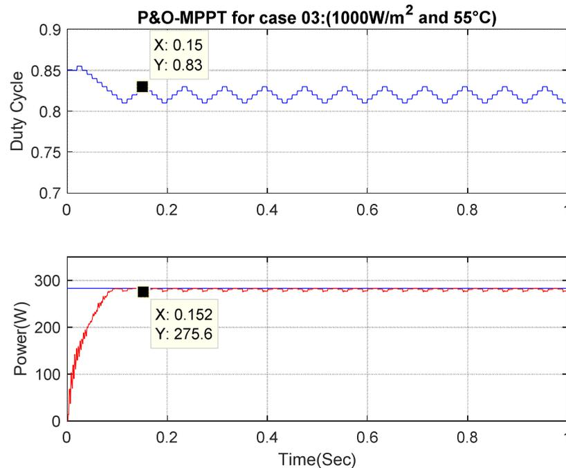
**Fig.III.15.** Duty cycle and PV power responses using P&O based MPPT technique for case 03 ( $1000\text{W}/\text{m}^2$ ,  $55^\circ\text{C}$ )
