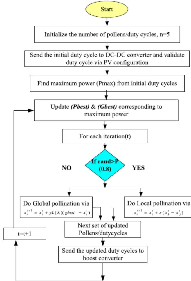
Fig. I.11. Flowchart for FPA implemented MPPT [63]
