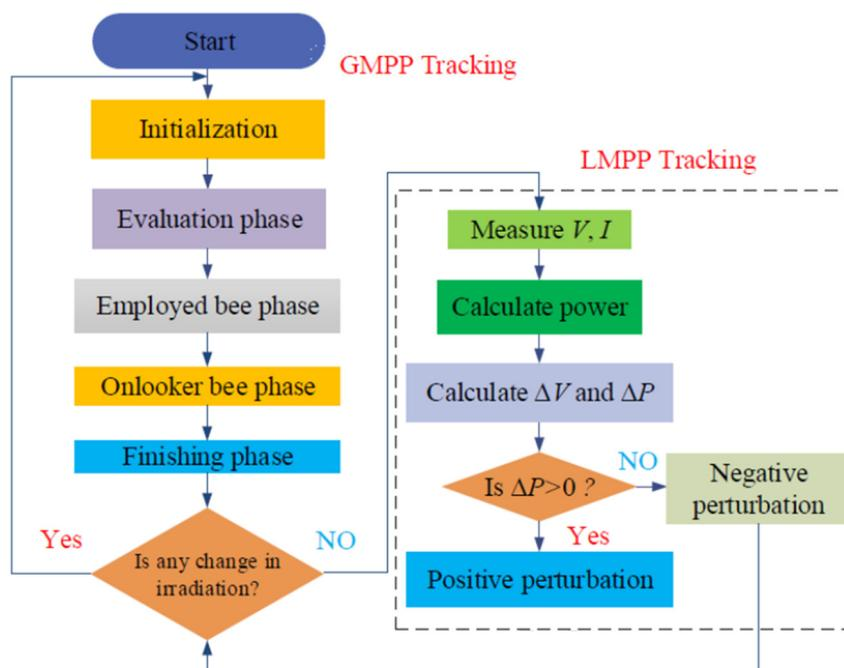
Fig. I.16. Flowchart of hybrid algorithm ABC-P&O based MPPT [76]
