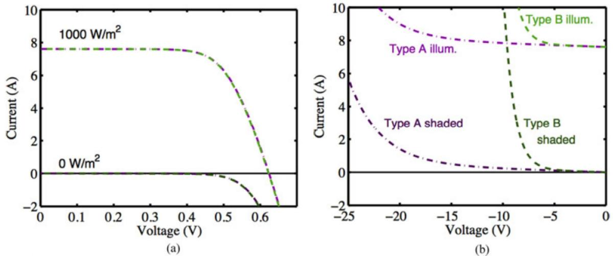
**Fig. II.2.**  $I$ - $V$  curve in (a) forward and (b) reverse voltage region for illuminated and shaded Type A and B cells.
