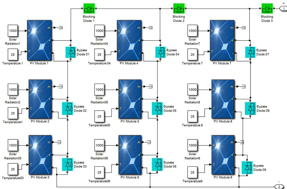
Fig. II.19. Simulink model of PV configuration Series-Parallel (3S3P) under STC
