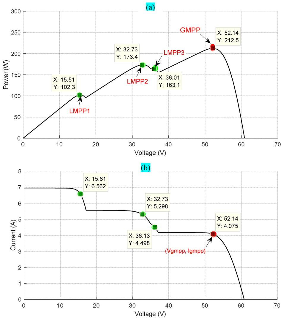
**Fig.III.11.** Characteristics curves of PV array 3S2P under PSC (a) P-V curve (b) I-V curve
