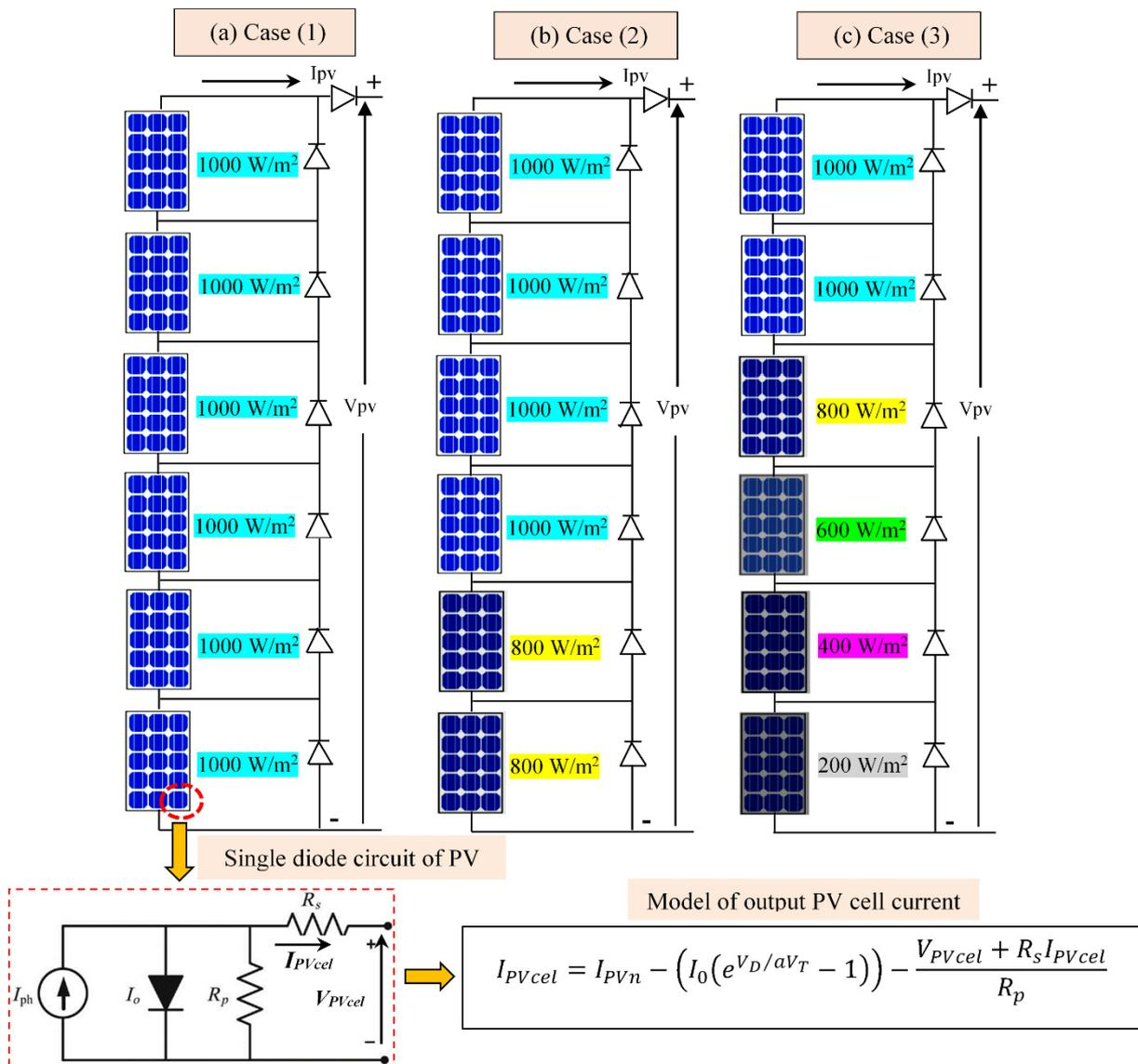
**Fig.IV.2.** PV modules configuration (6S) under tested partial shading cases with the equivalent single diode circuit of the PV cell
