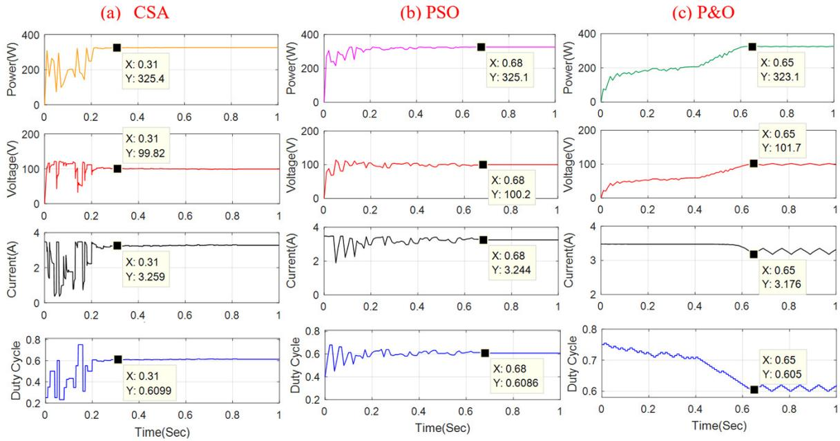
Fig.IV.11. Simulated system responses of CSA, PSO and P&O methods under case 1
