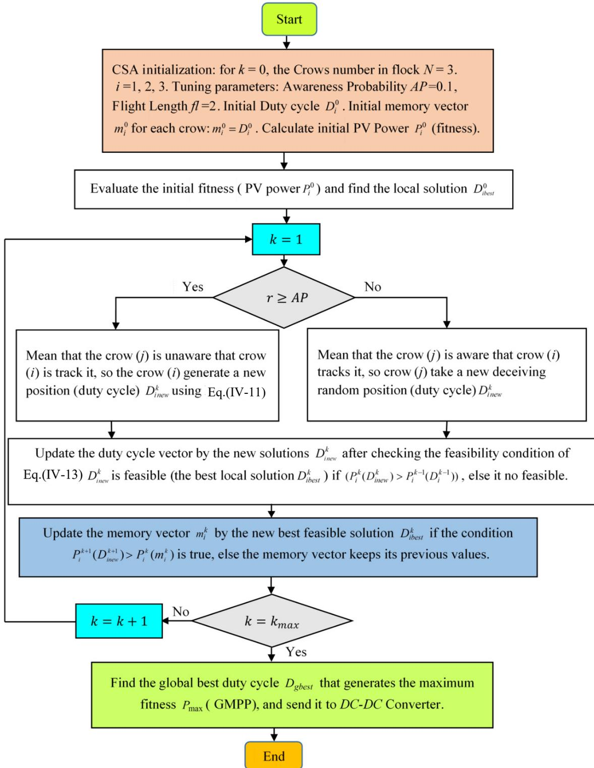
**Fig. IV.8.** Flowchart of the proposed CSA technique implemented for the global optimization problem based MPPT
