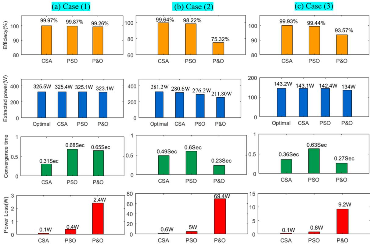
**Fig.IV.15.** Quantitative comparison between the performances of CSA, PSO and P&O methods for different PSCs
