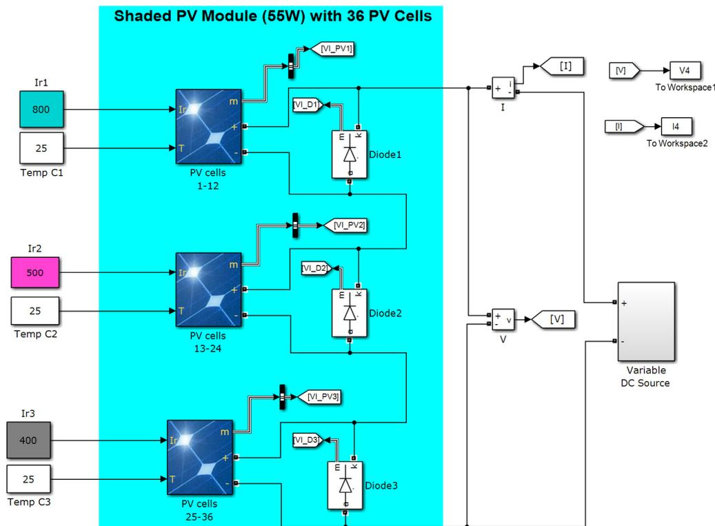
**Fig. II.12.** Model of partially shaded PV module cells (36 cells) under the partial shading conditions of scenario 4
