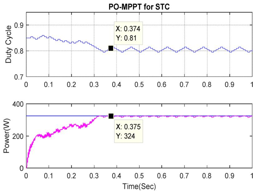
**Fig.III.7.** Duty cycle and PV power responses using P&O based MPPT technique for STC case
