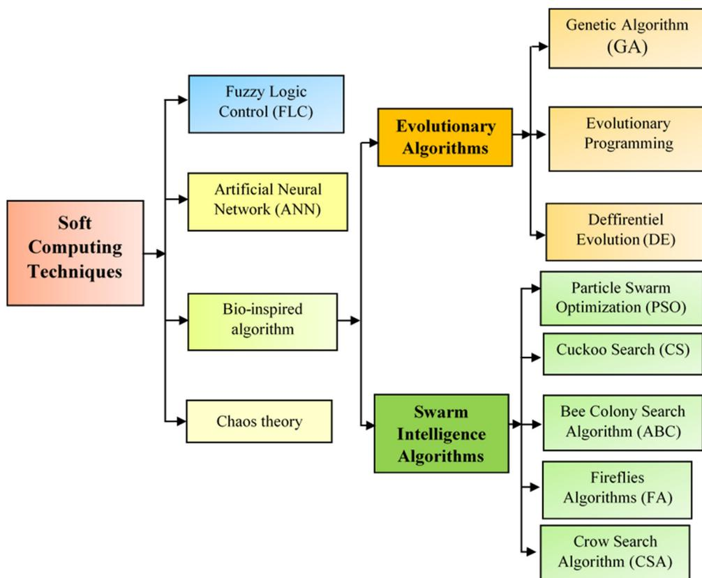
Fig. I.4. Soft computing techniques used for MPPT application [49].
