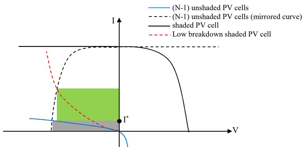
**Fig. II.5.** Geometric approach to determine the power dissipation in a fully shaded cell based on the I–V curve
