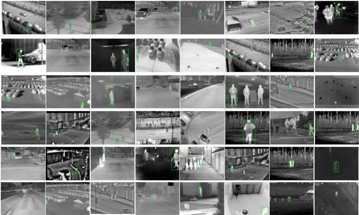
Fig.2.8 The first frame from some selected sequences of the PTB-TIR Dataset. The target is surrounded by a green bounding box [92].
