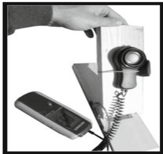
Fig. 1. The slope angle variation of pyranometer.
