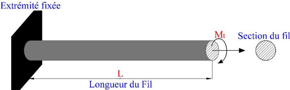
Figure 67. Principe de torsion simple.
