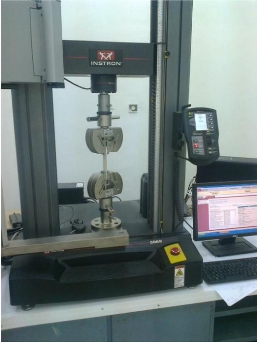
**Figure (III.4) :** Machine de traction
