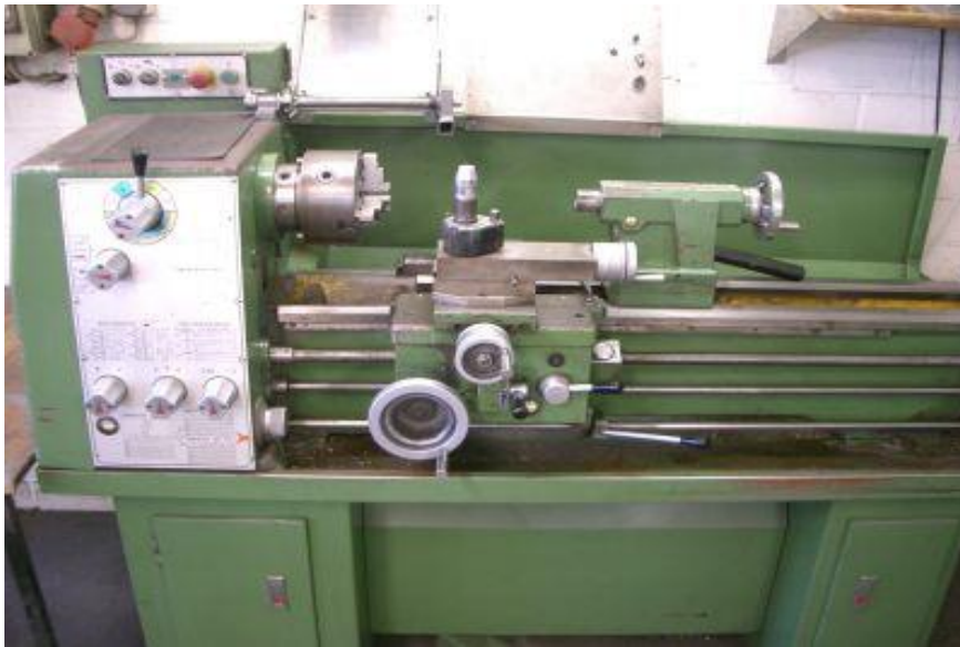
Figure III. 3: Tour type KNUTH model: sh 150/915 super.
