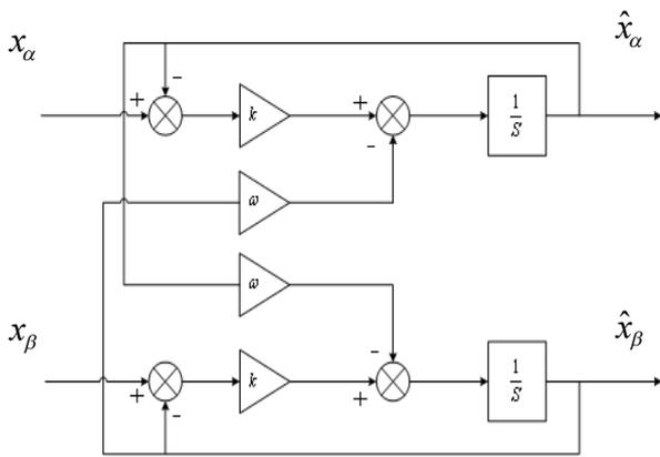
**Figure.3** - block diagram for STF
