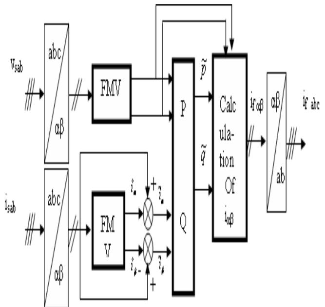
Figure. 2: The method of instantaneous active and reactive power
