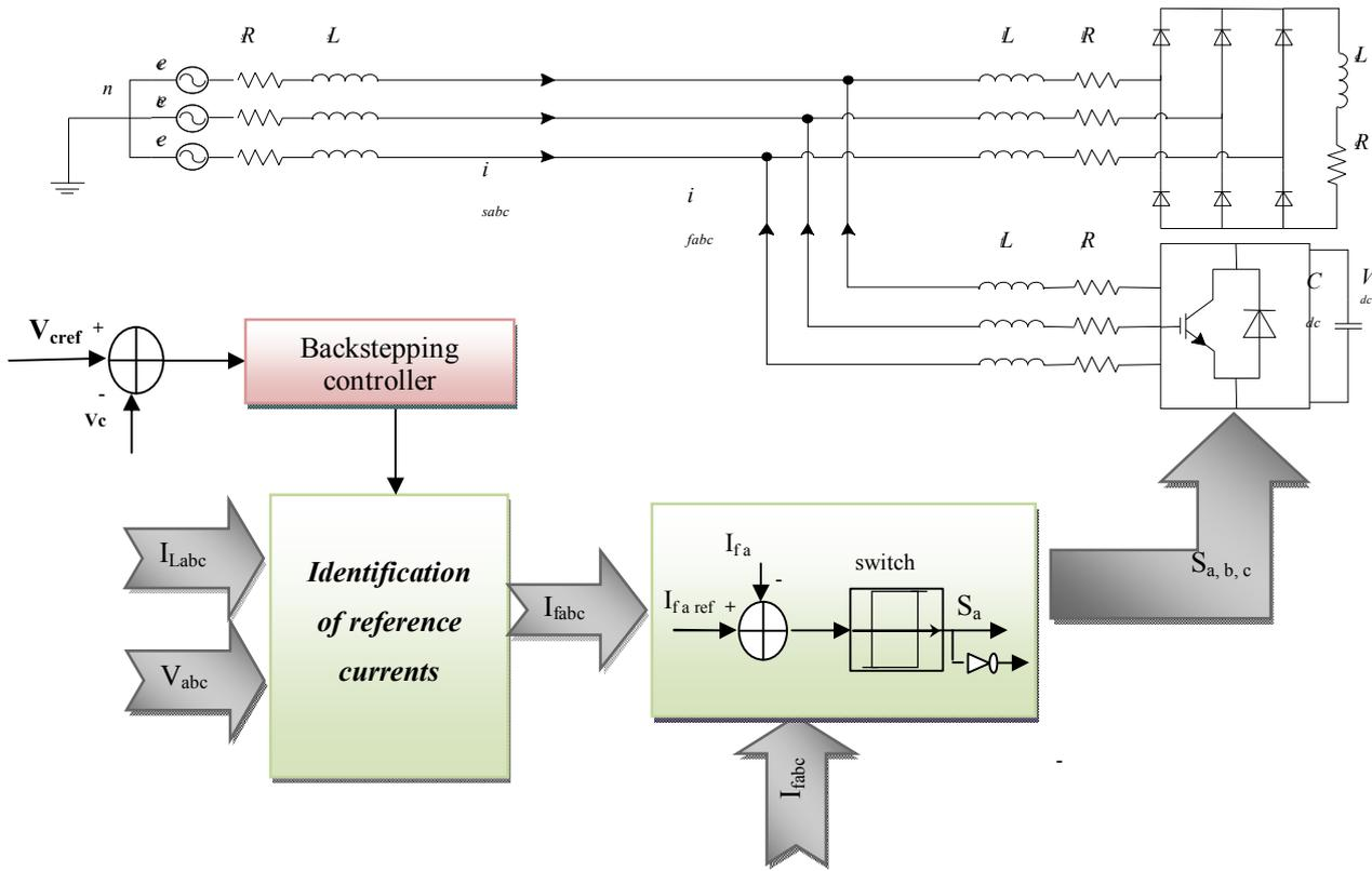
Figure.1 -Network and shunt active filter presentation
