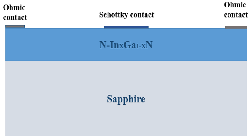
Figure III. 1: Structure of the InGaN based Schottky barrier solar cell studied in the simulation.
