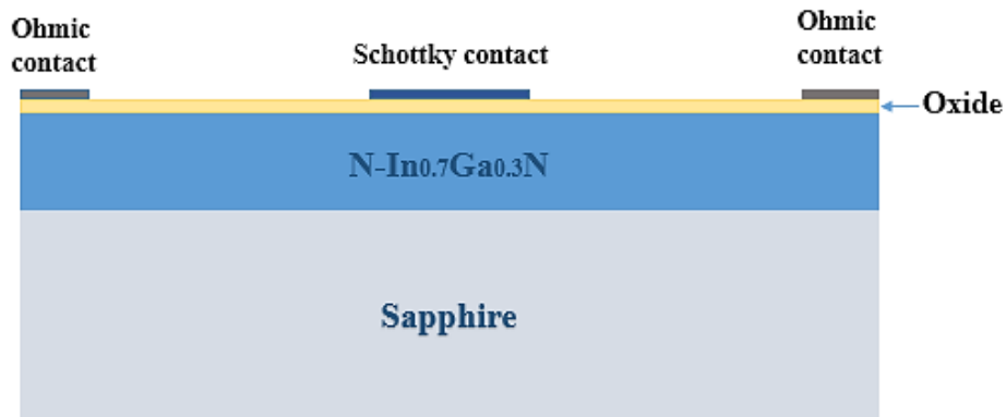
Figure III. 19: InGaN based MIS solar cell structure.
