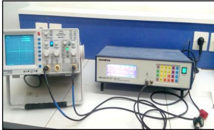
Figure II.8: Pulse-Echo device equipment: Immersion transducer with an Olympus Model 5800RP generator, coupled to a 20GHz oscilloscope (HAMEG type).
