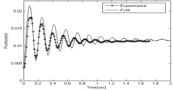
Fig. 4. Measured and computed values of the levitation height of the aluminum plate.
