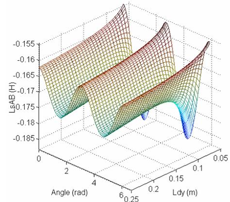
Fig. 8. Mutual inductance between stator winding  $A$  and  $B$  in dynamic axial eccentricity of  $\delta_{d0}=60\%$ , and  $L_{dy}=0.5x l \dots 2x l$
