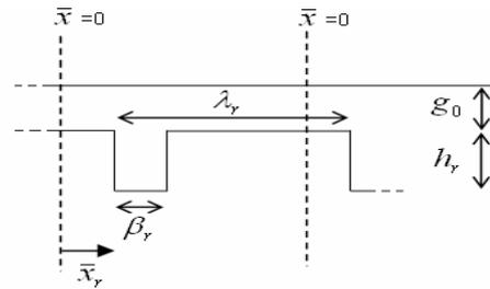
Fig. 13. air-gap variation due to rotor slotting effect
