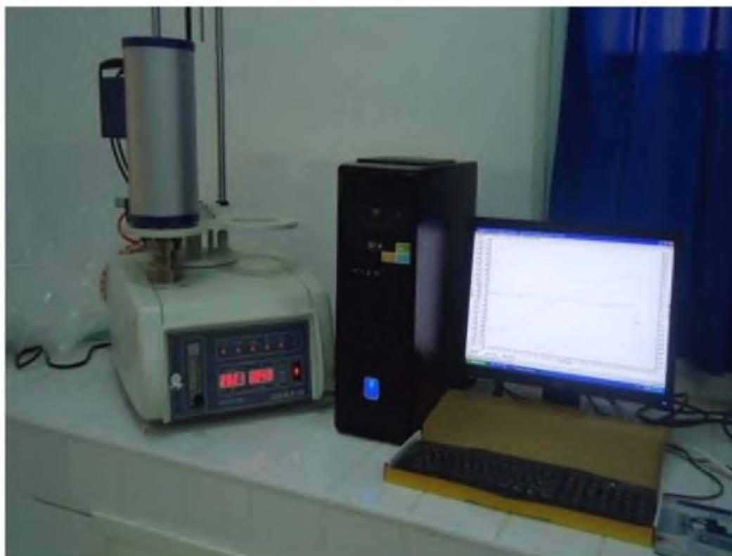
Figure II. 3: Appareil Linseis STA PT1600.
