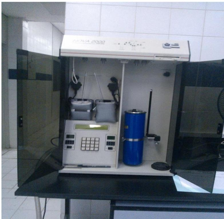
**Figure III.6.** Appareil Quantachrome NOVA 2200.
