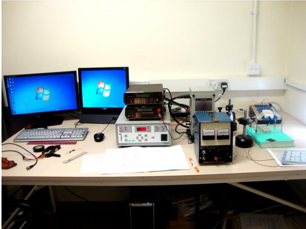
Figure A-1: Measure equipment of the micromorph tandem cell I - V characteristic at Dundee University.
