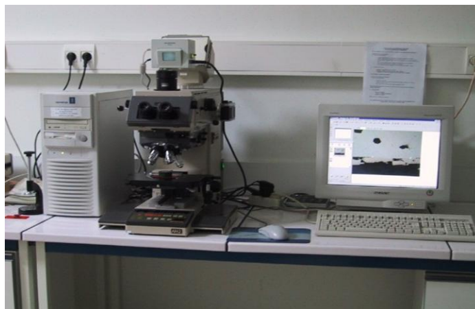
Figure II.5. Microscope optique OLYMPUS Vanox-AH2
