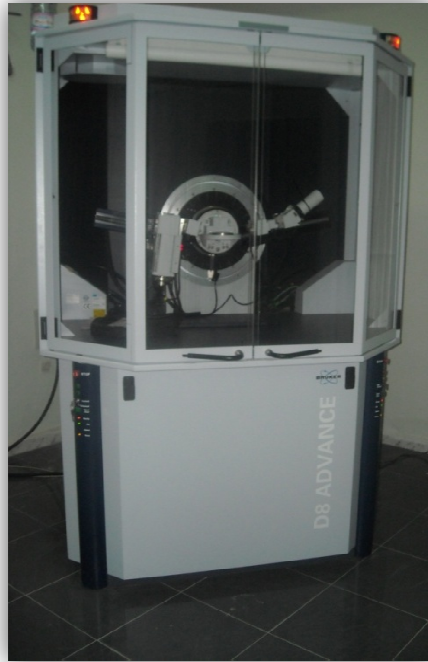
Fig II.8: diffractomètre de type BRUKER D8 ADVANCE AXS (XRD)
