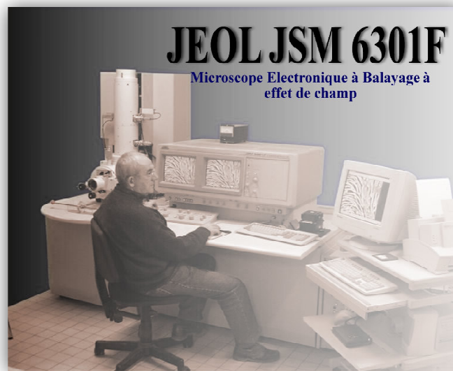
Fig .II.10 : JEOL, model JSM 6301F Scanning Microscopy
