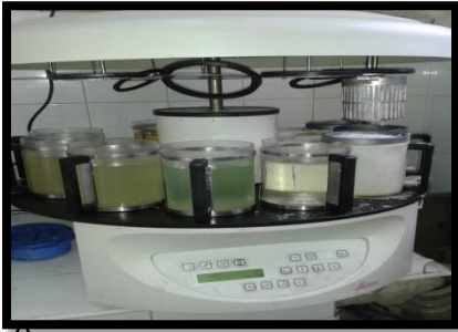
Figure 61. Automate de circulation
