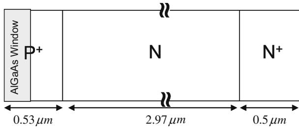
Fig. 1. A schematic diagram of the solar cell used in this work.
