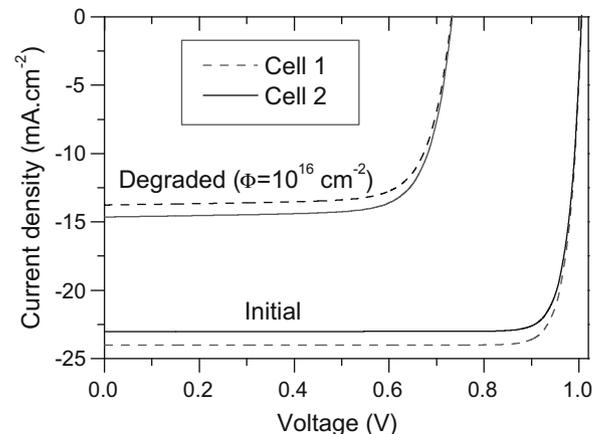
Fig. 3. The calculated  $J$ – $V$  characteristics of the illuminated solar cells before and after irradiation by  $1 \times 10^{16}$  cm<sup>-2</sup> electron fluence.
