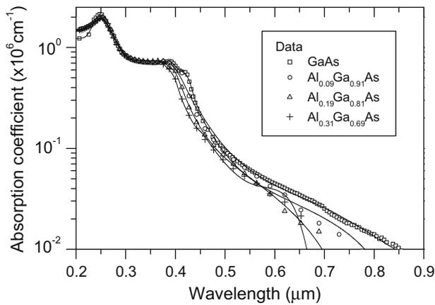
Fig. 4. The fitted and tabulated [21] absorption coefficient for the different  $\text{Al}_x\text{Ga}_{1-x}\text{As}$  layers.
