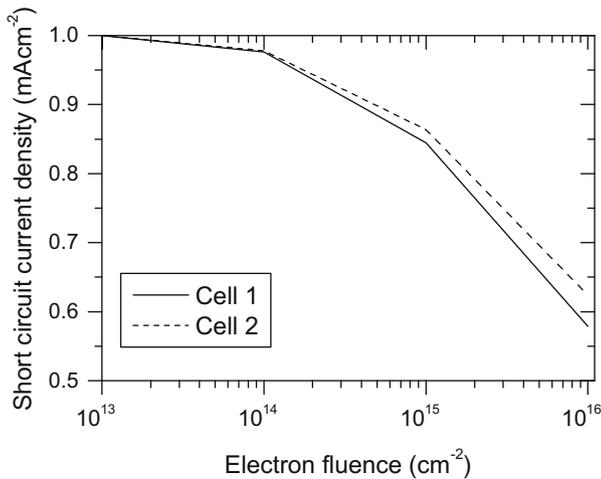
Fig. 5. The normalized short circuit current density degradation.
