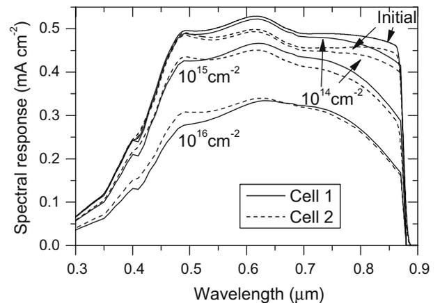
Fig. 2. Degradation of the spectral response by the different electron fluences.
