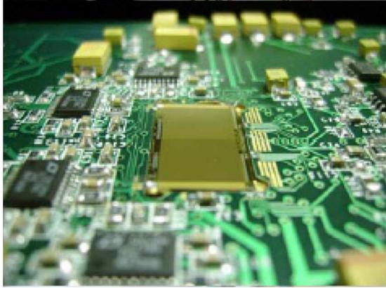
Fig. 2. CPC1 (in the center of the picture) with external electronics.
