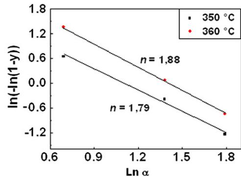
Fig. 6.  $\ln(-\ln(1-Y))=f(\ln \alpha)$  curves of Ni-3 at% In alloy at two different temperatures.
