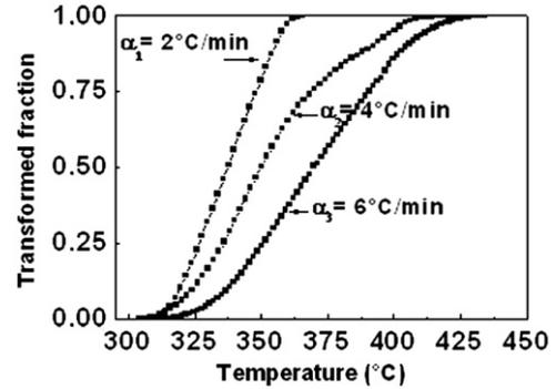
Fig. 5. Transformed fraction of Ni-3 at% In alloy at different heating rates  $\alpha=2, 4$  and  $6^\circ\text{C}/\text{min}$  as a function of temperature.
