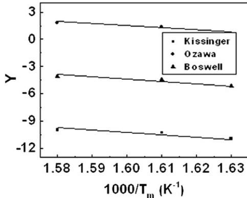
Fig. 4.  $Y=f(1000/T_m)$  curves of Ni-3 at% In alloy using three different methods.
