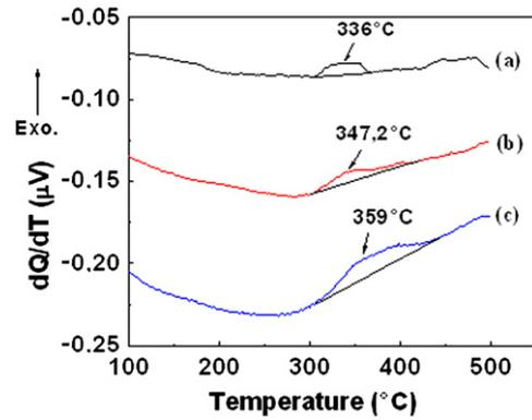
Fig. 3. DSC thermograms of Ni-3%at In alloy as a function of heating rate  $\alpha$ : (a)  $\alpha=2$  °C/min, (b)  $\alpha=4$  °C/min and (c)  $\alpha=6$  °C/min .
