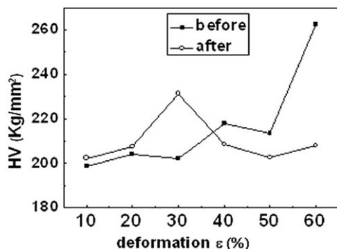
Fig. 9. Evolution of microhardness as a function of plastic deformation in Ni-3 at% In alloy (before and after DSC treatment).
