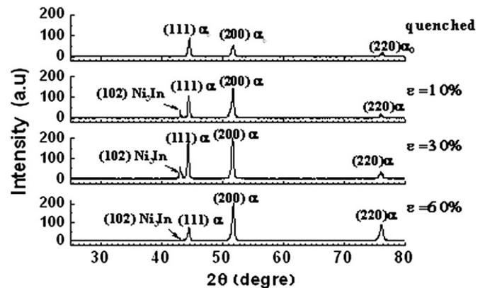
Fig. 7. X-ray spectra diffraction of Ni-3 at% In alloy quenched and deformed 10%, 30% and 60% (after DSC treatment).
