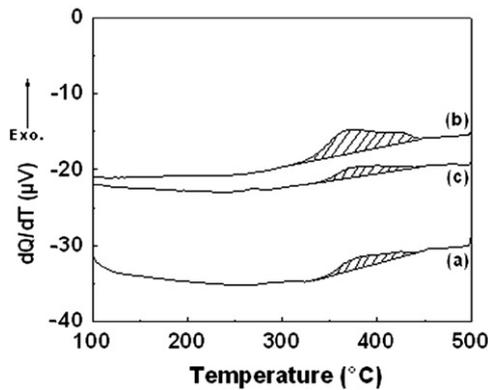
Fig. 1. DSC curves of Ni-3%at In alloy homogenized for 20 h at 1000 °C, quenched and deformed at  $\epsilon=10\%$ , 30% and 60% of reduction (heating rate  $\alpha=15$  °C/min).
