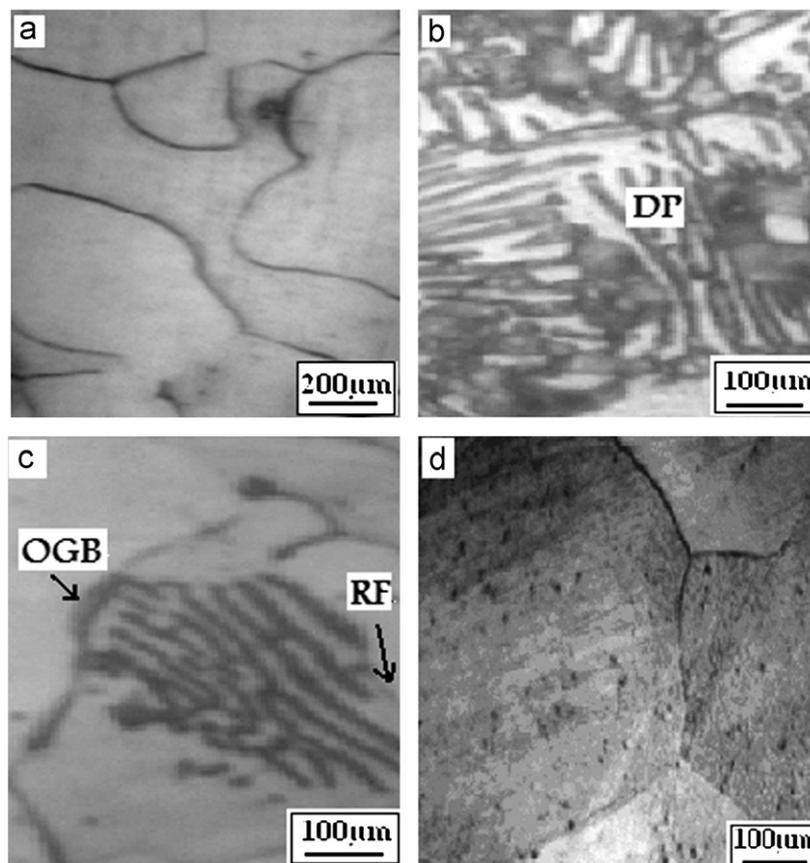
Fig. 8. Microstructures of Ni-3 at% In alloy homogenized at 1000 °C for 20 h; quenched and deformed 10% (a), 30% (b, c) and 60% (d), OGB—original grain boundary, RF—reaction front, and DP—discontinuous precipitation (microstructures after DSC treatment).
