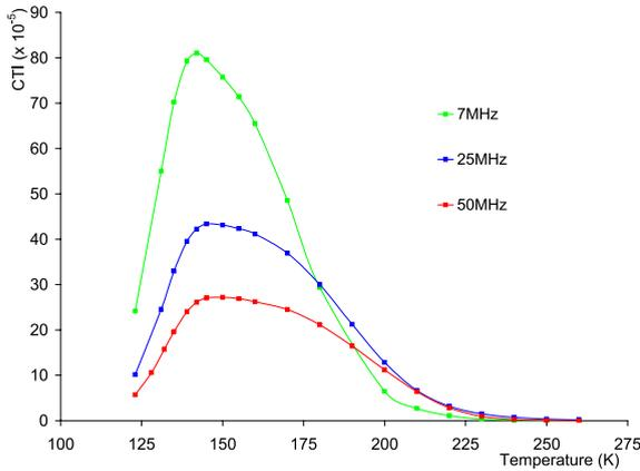
Figure 1. CTI for simulations with 0.17 eV partially filled traps clocked at 7, 25 and 50 MHz.
