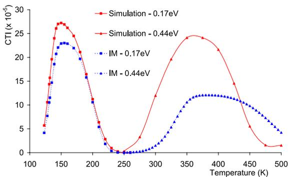
Figure 4. CTI values for simulations for 0.17 eV versus 0.44 eV partially filled traps at clocking frequency 50 MHz. Comparison of Improved Model (IM) with full DESSIS simulation.
