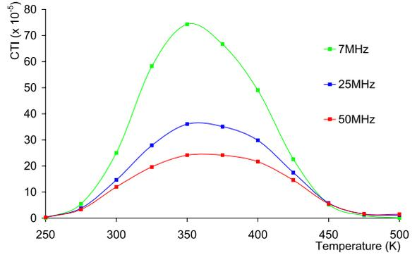
Figure 2. CTI for simulations with 0.44 eV partially filled traps clocked at 7, 25 and 50 MHz.
