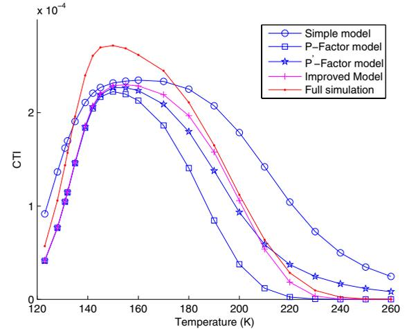
Figure 3. CTI values against temperature for different models with 50 MHz readout. See text.
