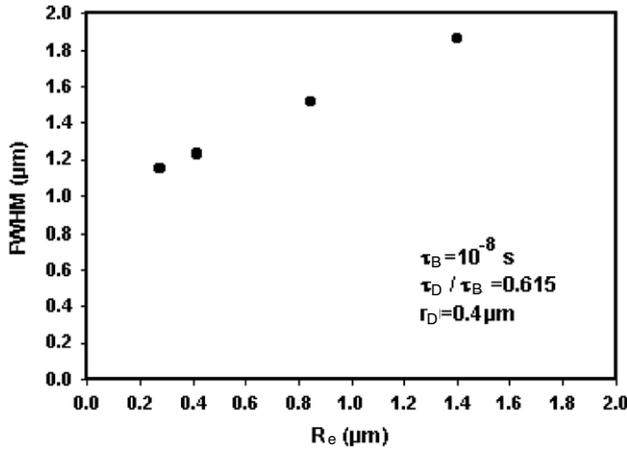
Figure 4. The FWHM of the contrast profile of a straight dislocation perpendicular to the surface versus the electron range in germanium.
