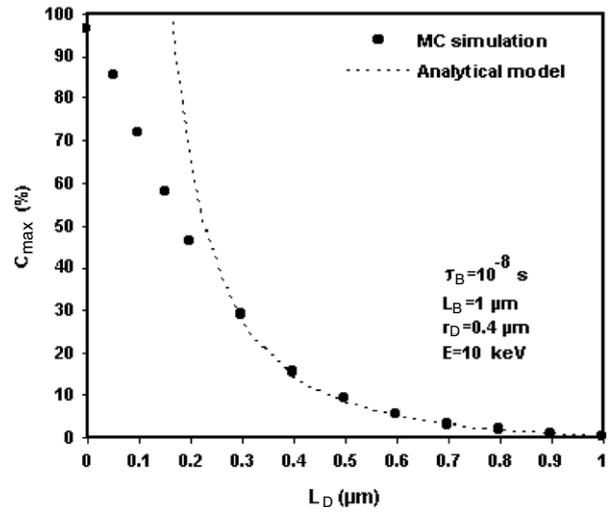
Figure 6. The variation of the maximum contrast upon the minority carrier diffusion length  $L_D$  within the dislocation cylinder.
