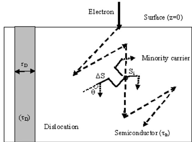
**Figure 2.** Schematic diagram of the random diffusion of the minority carriers.
