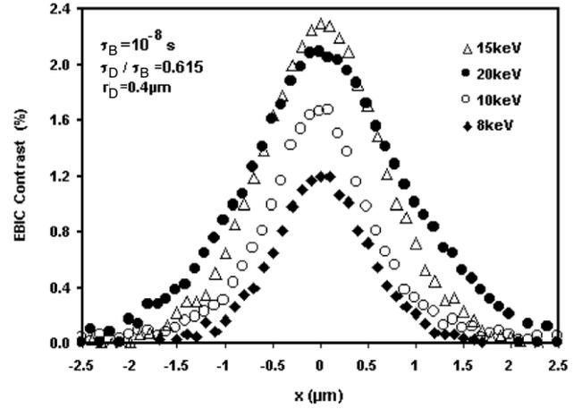
**Figure 3.** Simulated EBIC contrast profiles of a straight dislocation perpendicular to the surface for different beam energies in germanium.
