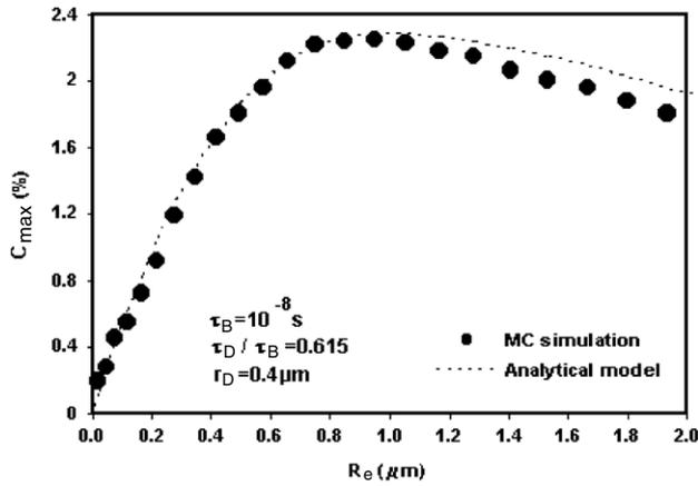
Figure 5. Maximum EBIC contrast of a straight dislocation perpendicular to the surface versus the electron range in germanium.
