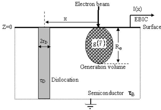
**Figure 1.** Schematic diagram of the EBIC analysis of a dislocation normal to the surface of a Schottky contact.
