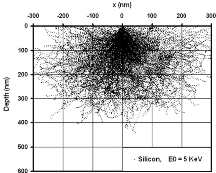
The generation function was obtained in the form of a three dimensional distribution of pointlike sources  $S_i$  localised at the middle of the path between two successive primary electron collisions.
