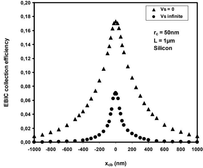
**Figure 3** Variation of the simulated maximum collection efficiency upon the nano Schottky contact radius in a silicon sample at 5 KeV for two different values of the free surface recombination velocity  $v_s = 0$  and  $v_s$  infinite (see online version for colours)
