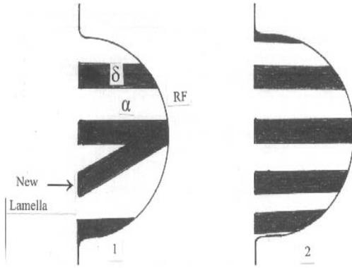
**FIG.5:** Illustration of branching mechanism observed in aged Cu-4.5 at. % In alloy: ( a ) : Formation of new  $\delta$  lamella by branching at the RF in the area indicated by narrow . ( b ) : an ideal DP colony, where the precipitate lamellae are equidistant, parallel to each other.
