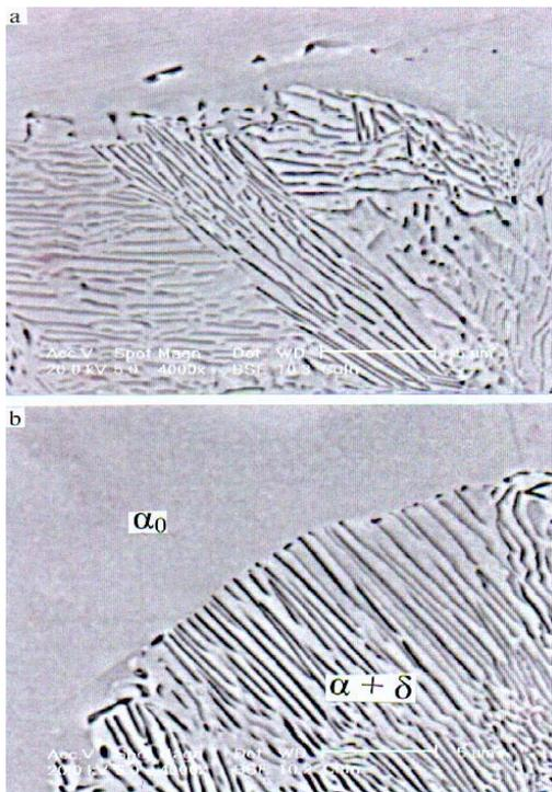
**FIG.3:** Two types of cells: ( a ) : cell characterized by irregular lamellar spacing ( b ) : ideal DP colony in aged Cu-4.5 at. % In alloy at 673K during 2 hours.
