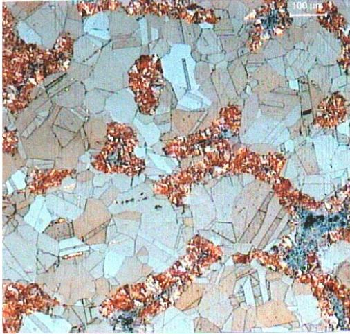
**FIG.2:** Development of cellular precipitation from a eutectic colony in an isothermally aged Cu-4.5 at. % In alloy at 673K during 1 hour.
