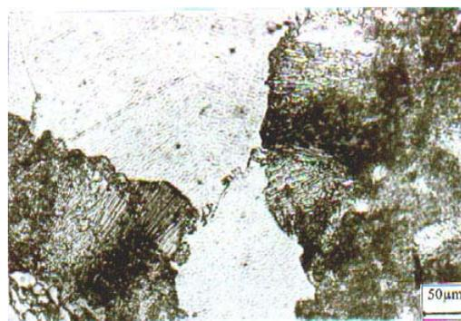
**FIG.1:** Cellular precipitation in an isothermally aged Cu-4.5 at. % In alloy at 673K during 2 hours.
