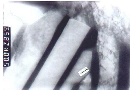
**FIG. 4:** Typical branching mechanism observed by MET in aged Cu-4.5 at. % In alloy at 673K during 2 hours.
